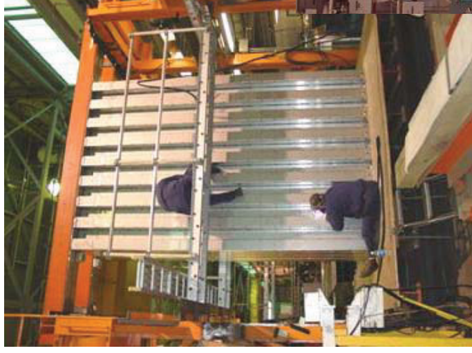
Holtec racks in fabrication at HMD
