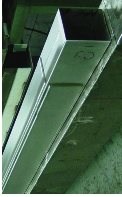
Holtec Rack Cell Box Fabricated at HMD
