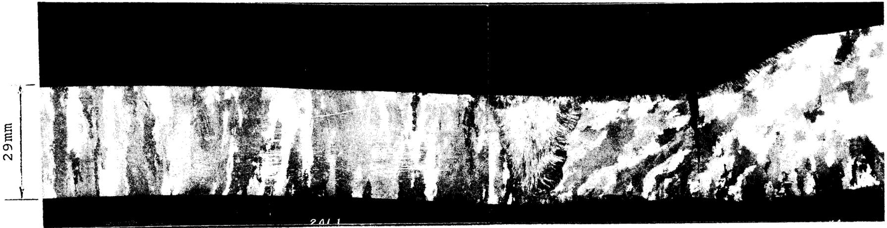
Figure 3.1 Longitudinal Section of the Elbow Showing Location of the Crack
