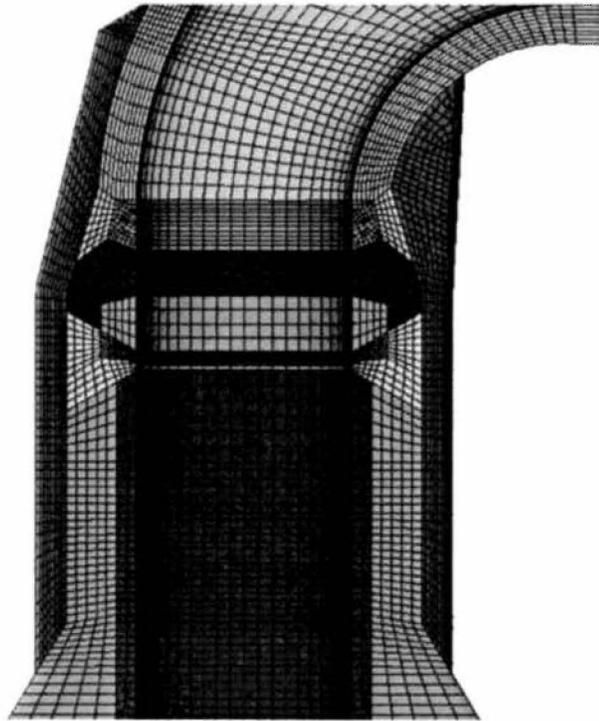
**Figure 3-10: Detailed mesh showing Weld Overlay**
