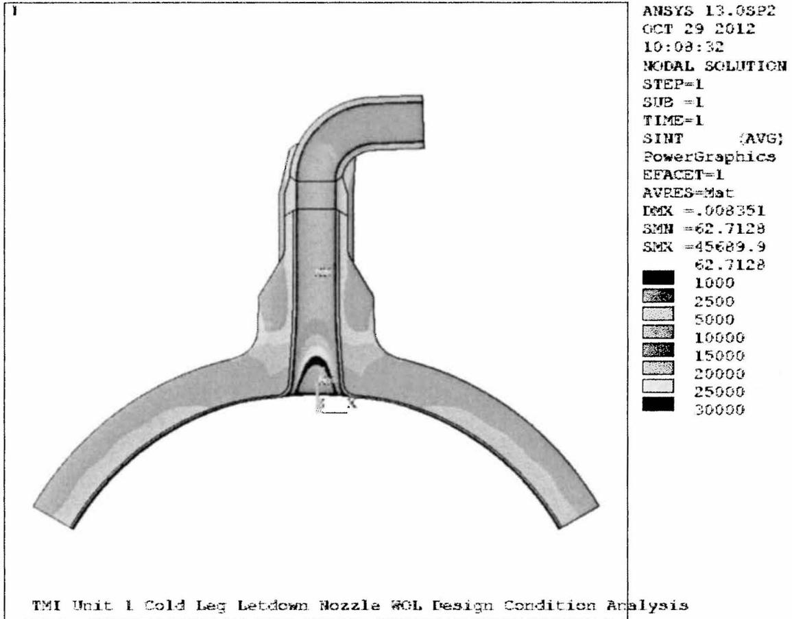
Figure 6-2: Stress Intensity Contours for Design Condition
