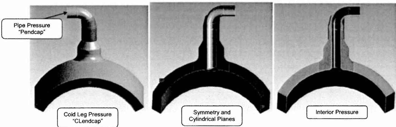
Figure 4-4: Structural Boundary Conditions
