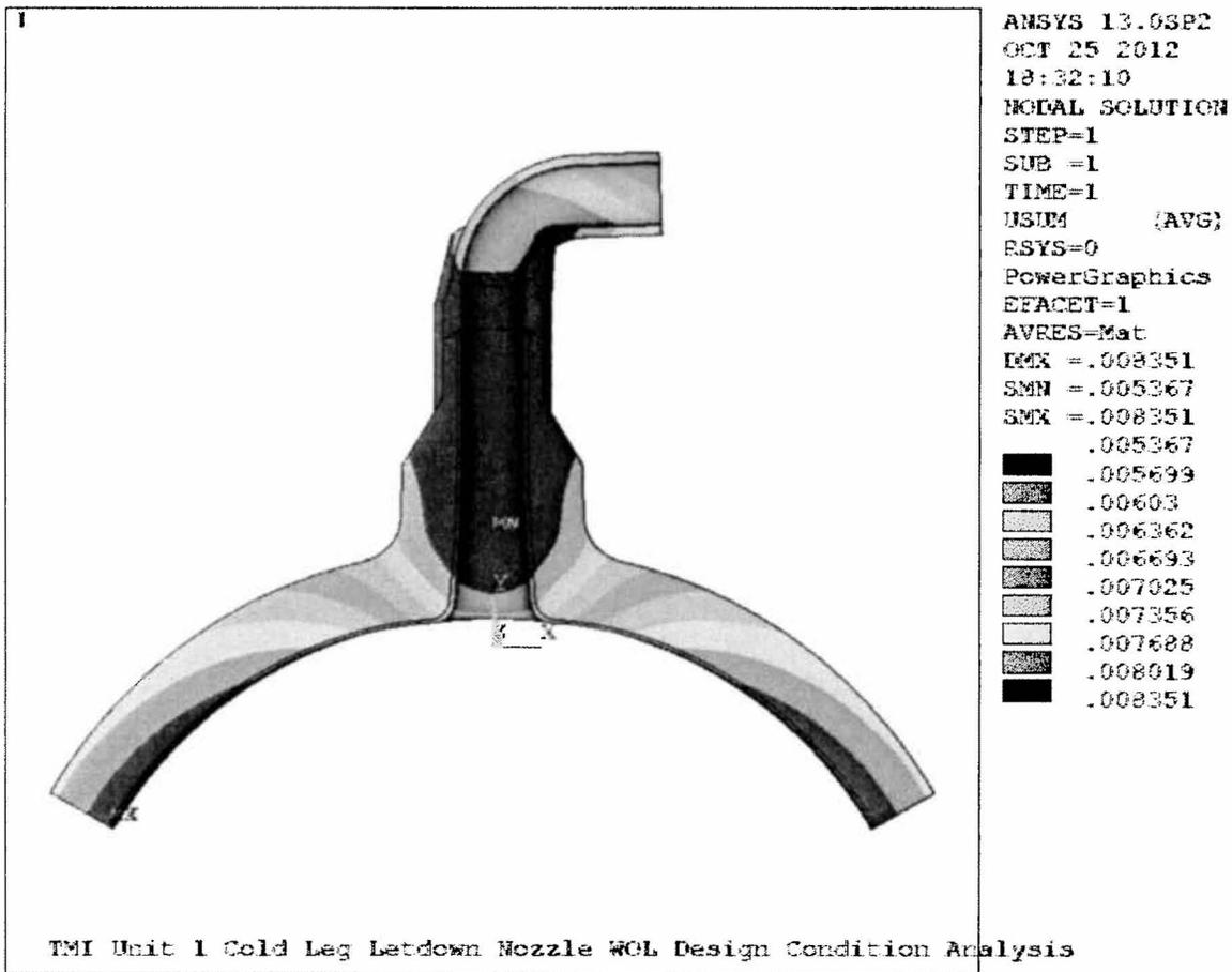
Figure 6-1: Deformed Shape for Design Condition
