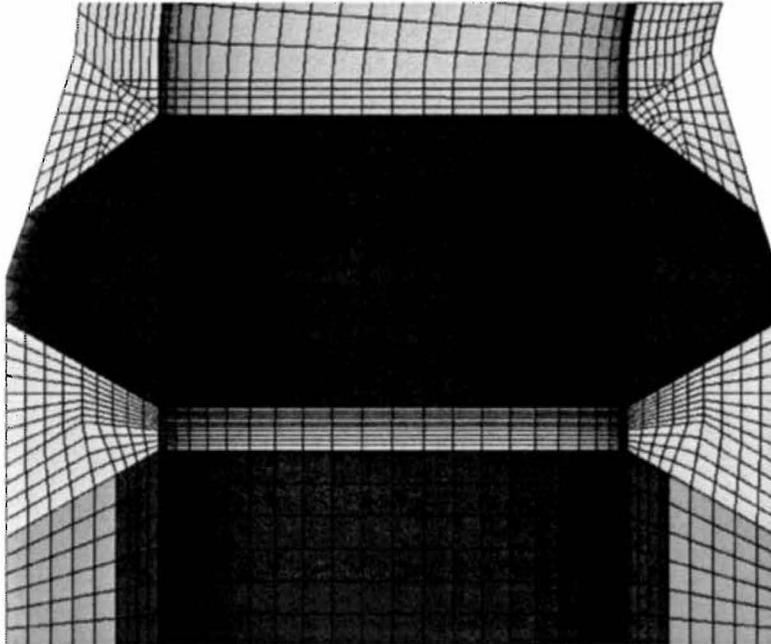
**Figure 3-8: Detailed mesh showing Repair Welds**
