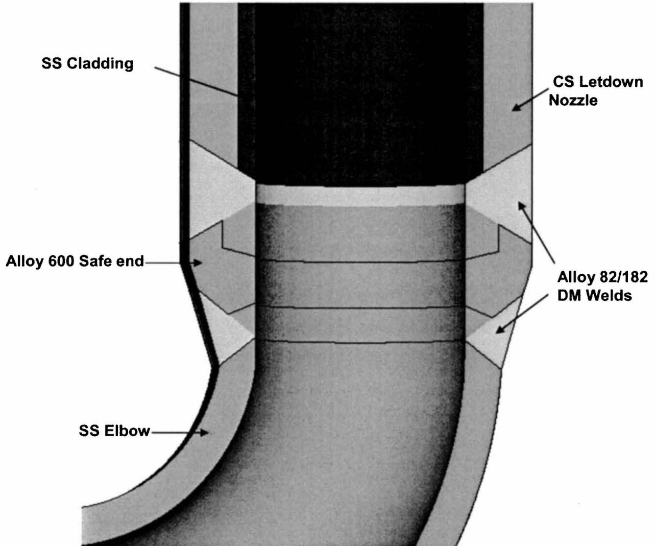
**Figure 3-3: ID Repair welds extending 50% of the original DM Weld**
