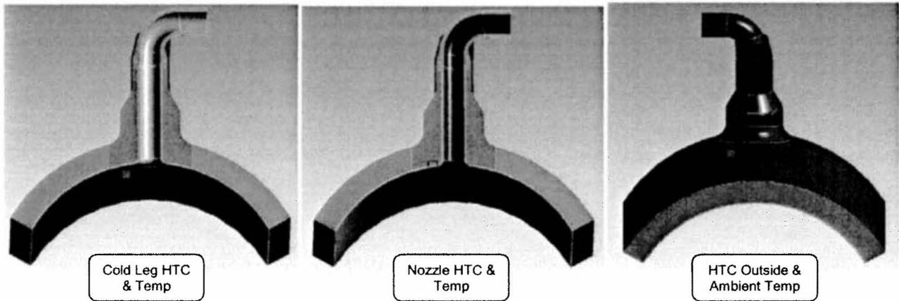
Figure 4-3: Thermal Boundary Conditions
