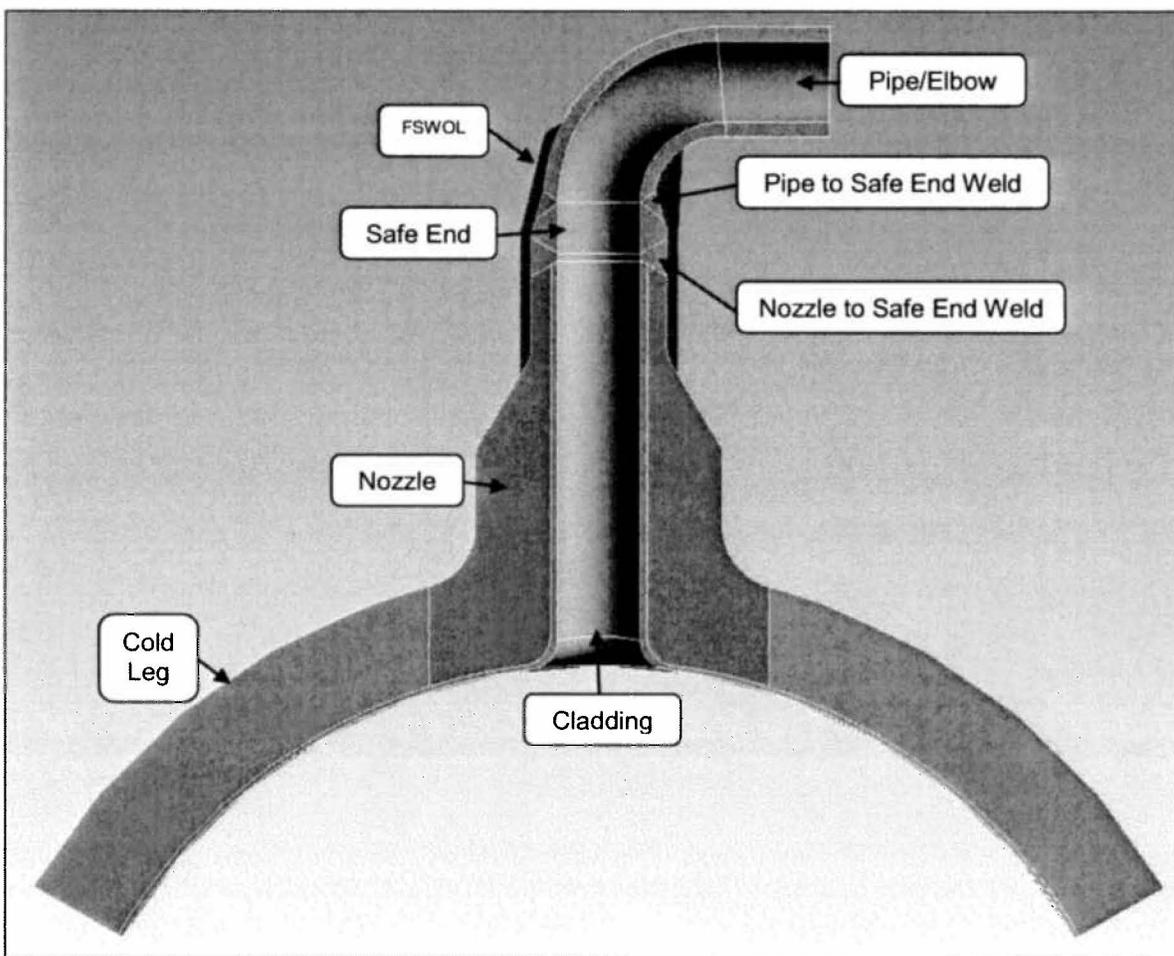
**Figure 4-1: Nozzle-FSWOL Geometry**
