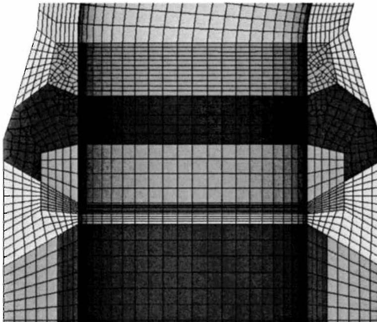
**Figure 3-9: Detailed mesh showing Weld Overlay**
