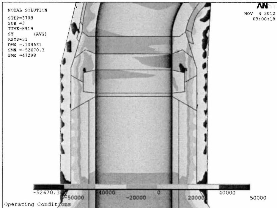
TMI Unit 1 Weld Residual Stress Analysis for CL Letdown Nozzle Weld Overlay – Non Proprietary
