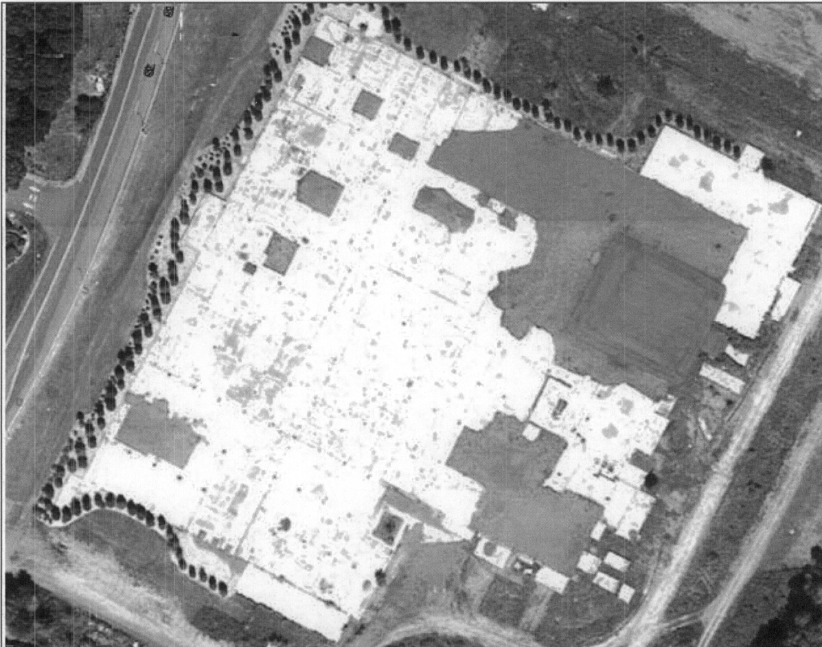
Figure 1. The Building 10 pad as it now exists. Concrete has been removed from the dark areas. The darkest area (upper right) is a large bituminous concrete cap, part of the PCB remediation project.
