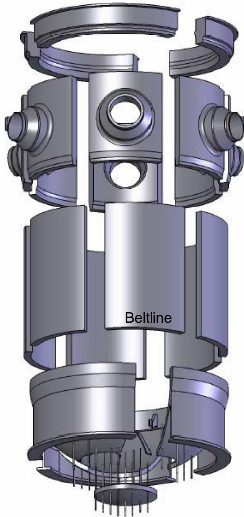
Figure 4.1. Reactor Vessel Cut Plan (Reference 24)
