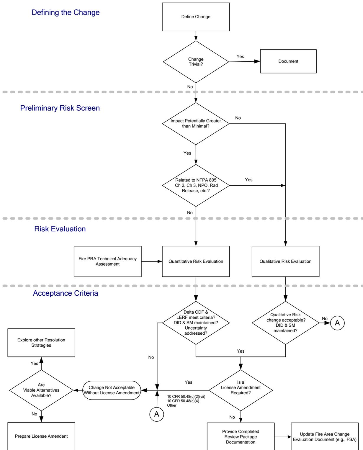
Figure 5-1 – Fire Protection Change Impact Review Process
