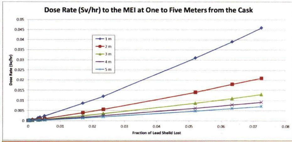
Figure 5-2. Radiation dose rates to the maximally exposed individual (MEI) from loss of lead gamma shielding at distances from one to five meters from the cask carrying spent fuel. The horizontal axis represents the fraction of shielding lost—the shielding gap.
