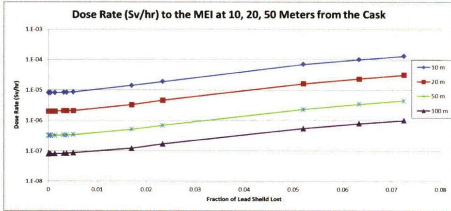
Figure 5-3. Radiation dose rates to the maximally exposed individual from loss of lead gamma shielding at distances from 10 to 100 meters from the cask carrying spent fuel. The vertical axis is logarithmic so that all of the doses can be shown on the same graph. The horizontal axis represents the fraction of shielding lost—the shielding gap.
