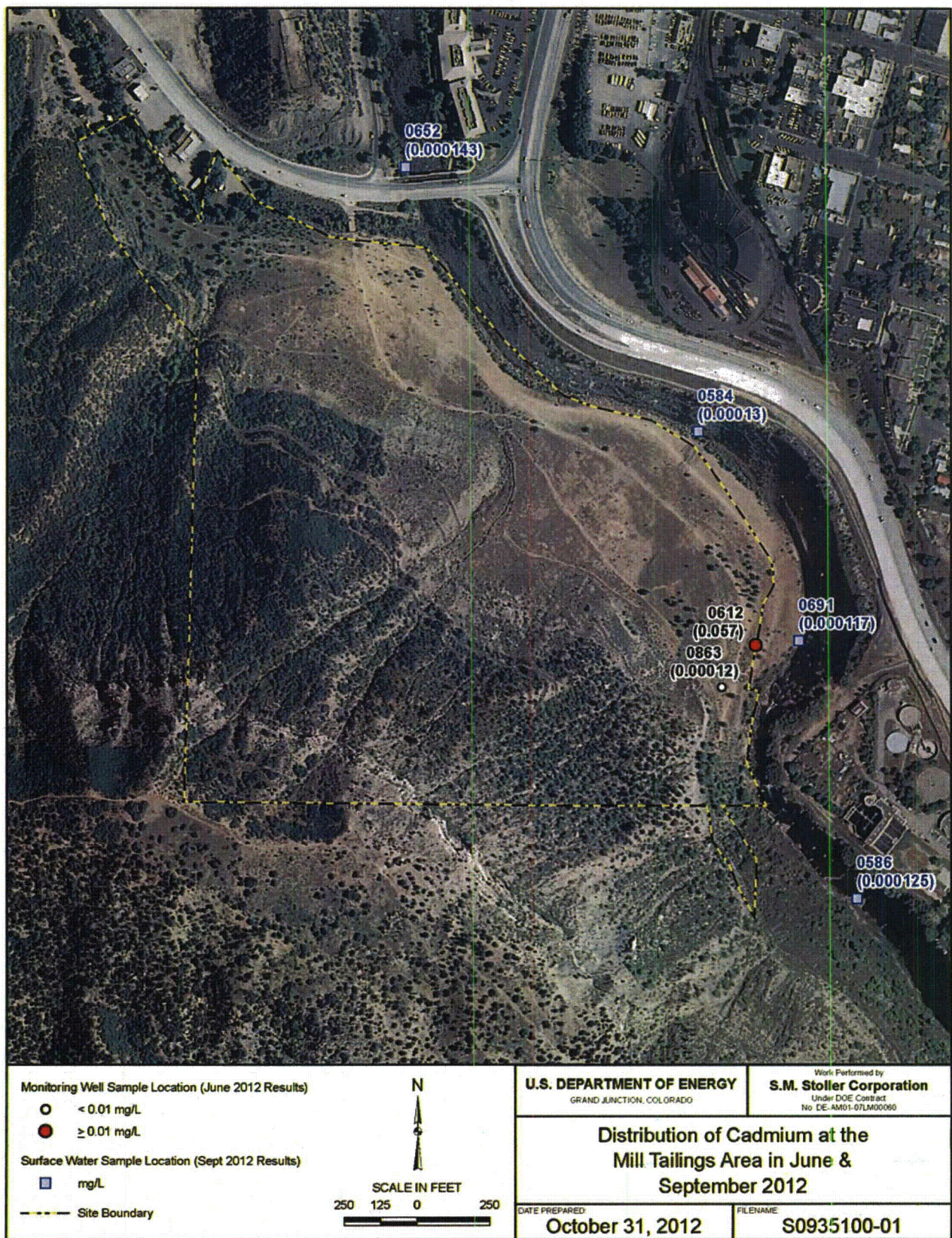
Figure 4. Distribution of Cadmium at the Mill Tailings Area in June and September 2012
