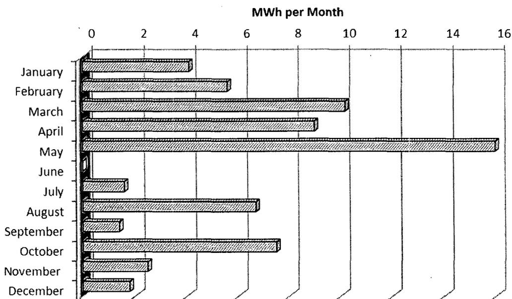
**Figure 1 - Energy generated by the KSU Triga Mark II reactor by month for CY 2012.**
