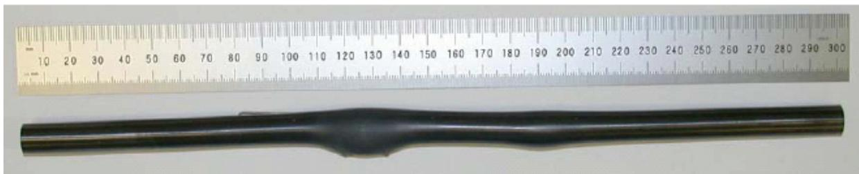
**Figure 18 Ballooned and ruptured region of unirradiated Zircaloy-2 after undergoing LOCA conditions (Figure 217 in Ref. 13)**
