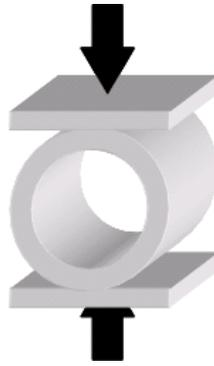
**Figure 23 Diagram of ring-compression test**
