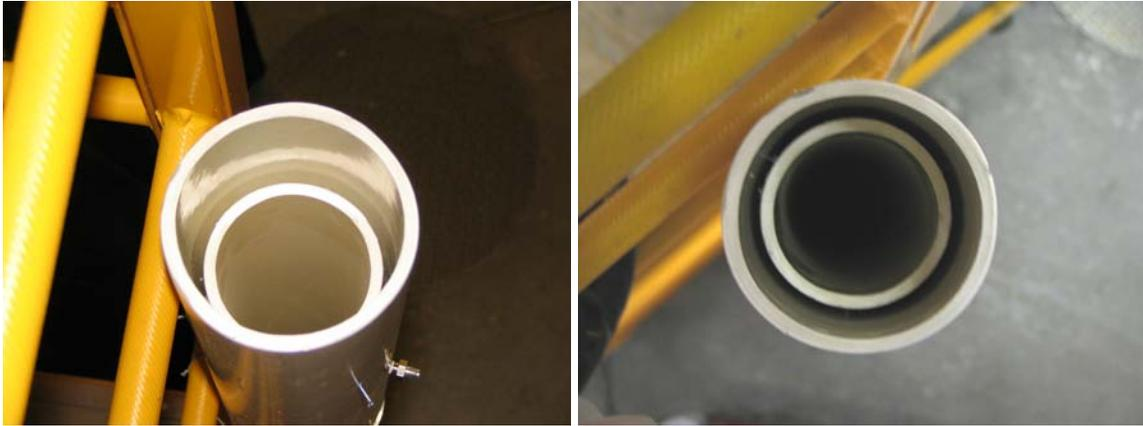
**Figure A.1** Isometric and overhead views of the annular flow path.
