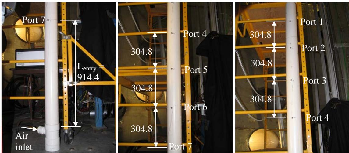
**Figure 2** Photographs of the annular test section. All dimensions are in millimeters.
