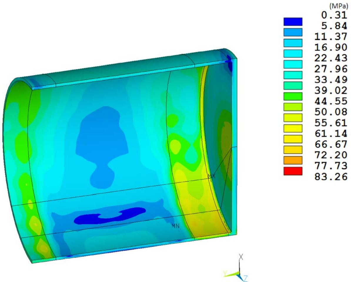
**Figure 8-2. RT-100 Inner Shell NCT Side Drop Stress Intensity Results.**
