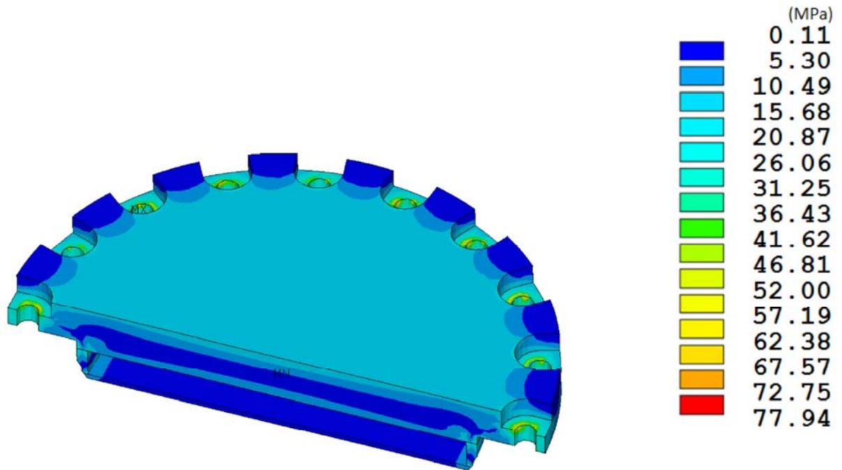
**Figure 8-30. RT-100 HAC Inner Lid Stress Intensity Results.**
