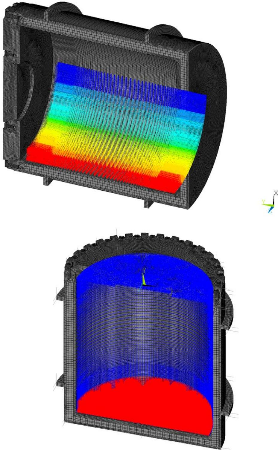
**Figure 7-4. Pressure Distribution used to Simulate the Contents.**
