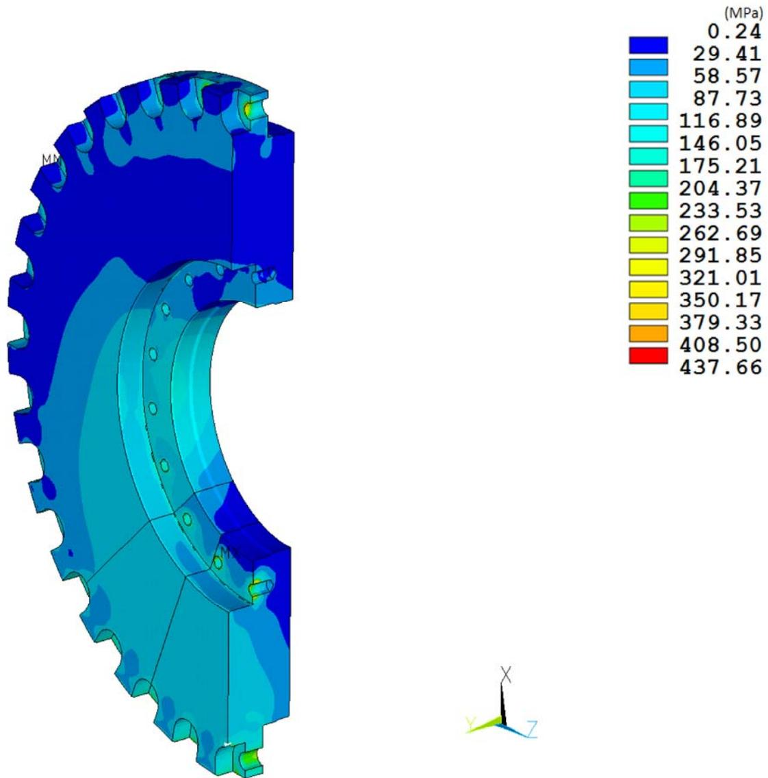
**Figure 8-17. RT-100 Outer Lid HAC Side Drop Stress Intensity Results.**
