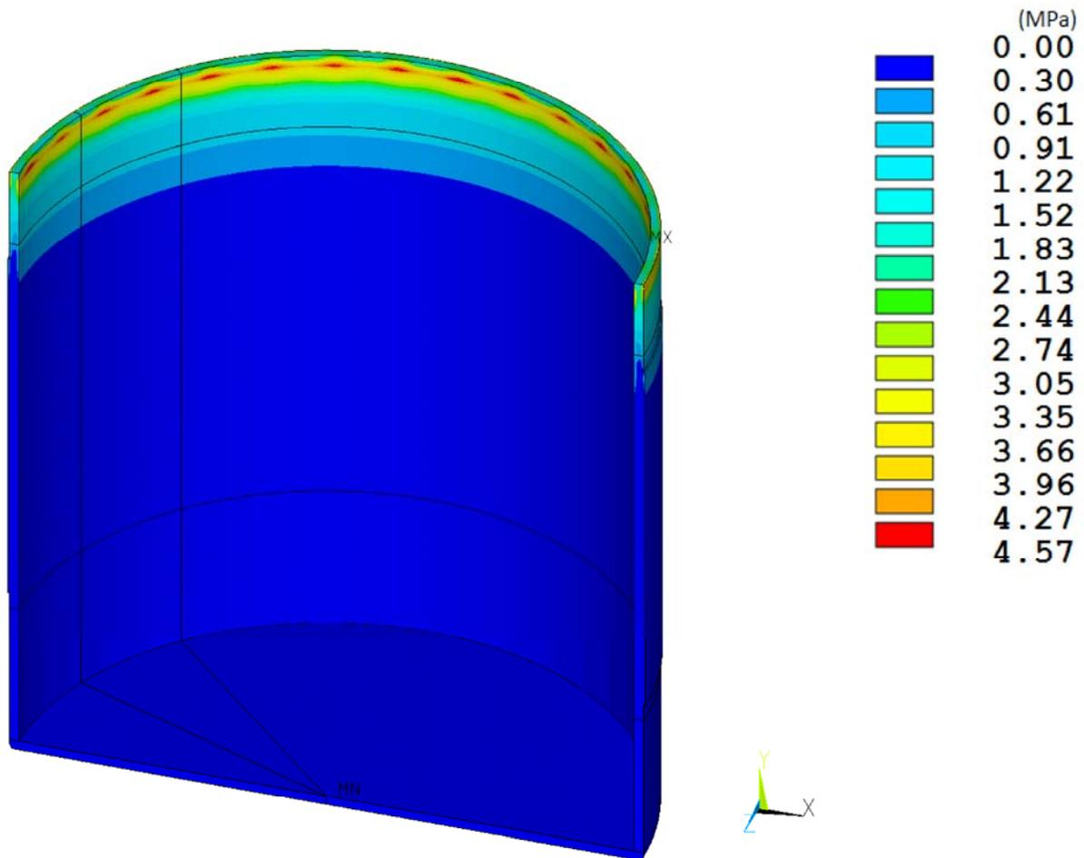
**Figure 8-27. RT-100 HAC Outer Shell Pressure Stress Intensity Results.**
