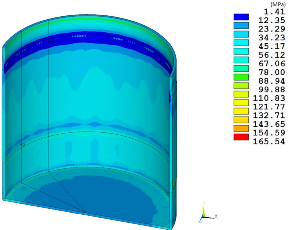
**Figure 8-21. RT-100 Outer Shell HAC End Drop Stress Intensity Results.**
