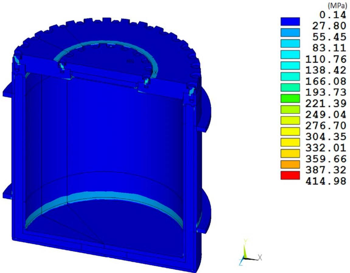
**Figure 8-19. RT-100 HAC End Drop Stress Intensity Results.**
