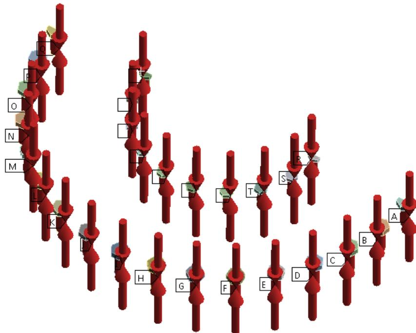
**Figure 7-5. Bolt Pre-load using ANSYS Pre-Tension Elements (PRETS179).**
