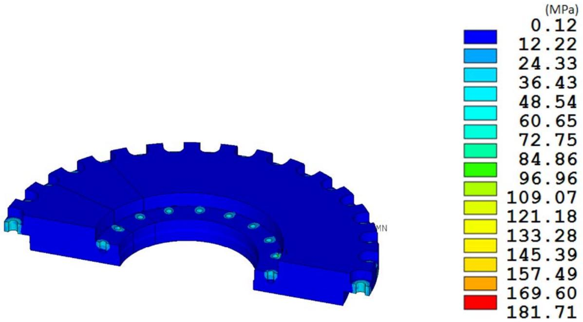
**Figure 8-11. RT-100 Outer Lid NCT End Drop Stress Intensity Results.**
