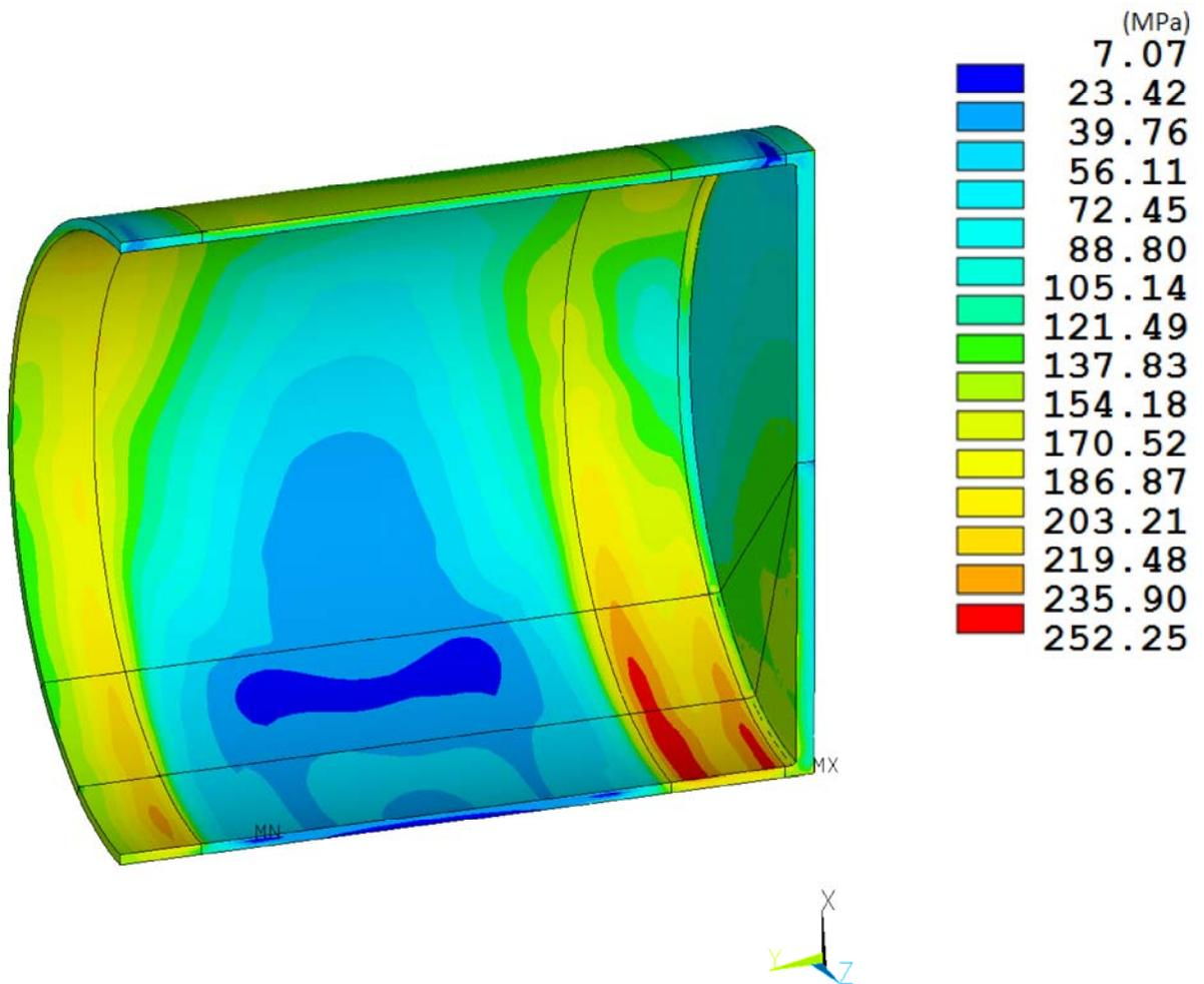
**Figure 8-14. RT-100 Inner Shell HAC Side Drop Stress Intensity Results.**
