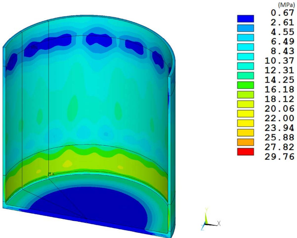
**Figure 8-8. RT-100 Inner Shell NCT End Drop Stress Intensity Results.**
