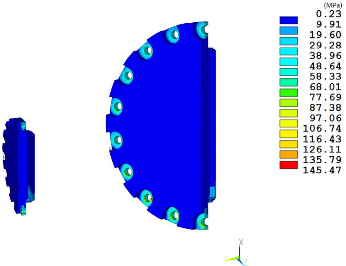
**Figure 8-6. RT-100 Inner Lid NCT Side Drop Stress Intensity Results.**
