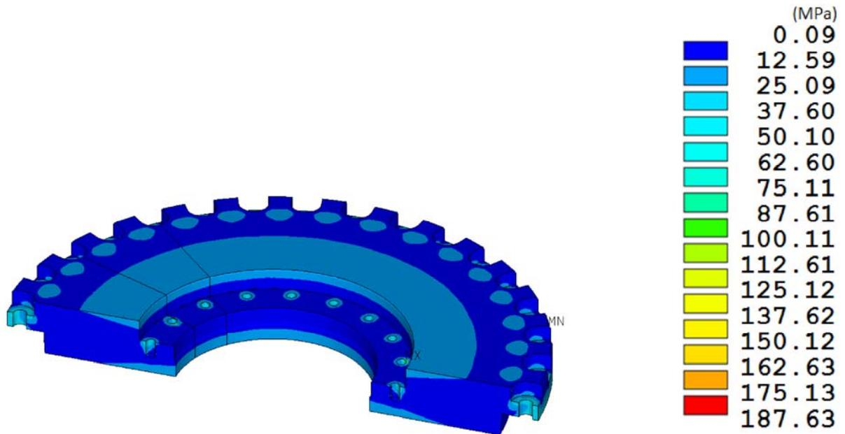
**Figure 8-29. RT-100 HAC Outer Lid Stress Intensity Results.**
