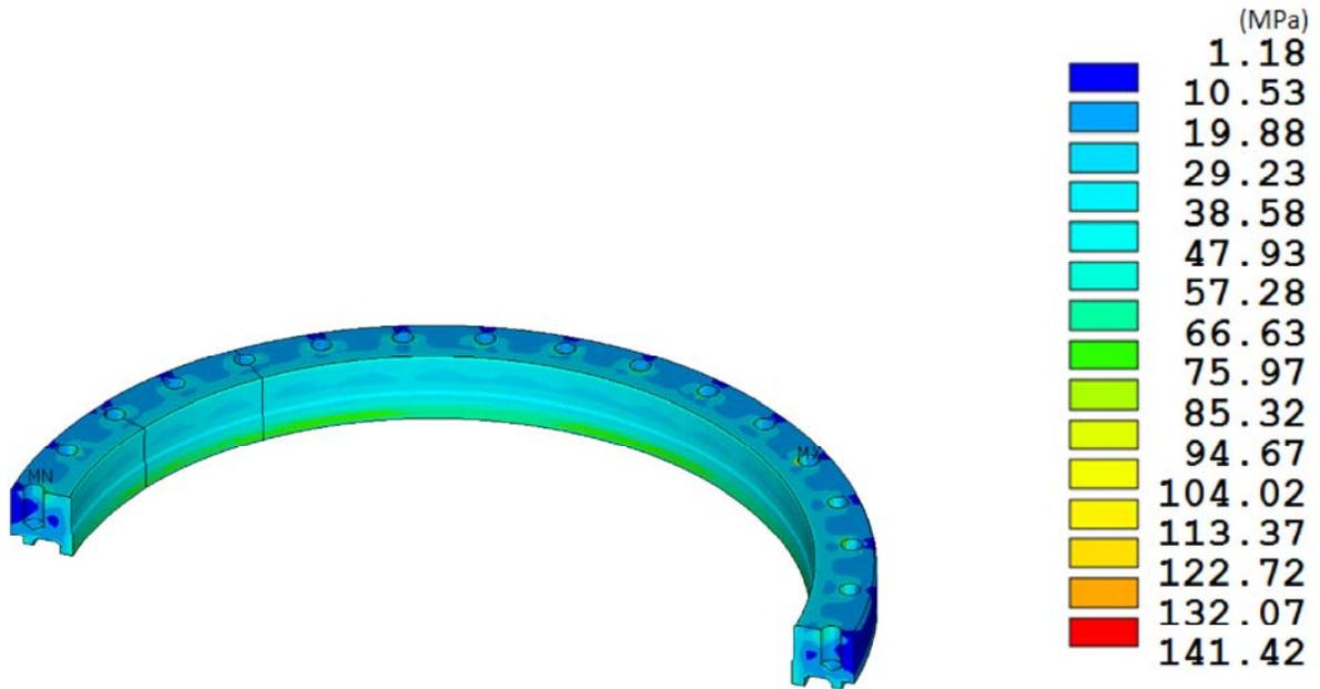
**Figure 8-22. RT-100 Flange HAC End Drop Stress Intensity Results.**
