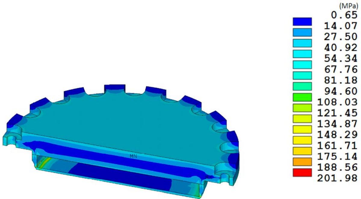
**Figure 8-24. RT-100 Inner Lid HAC End Drop Stress Intensity Results.**
