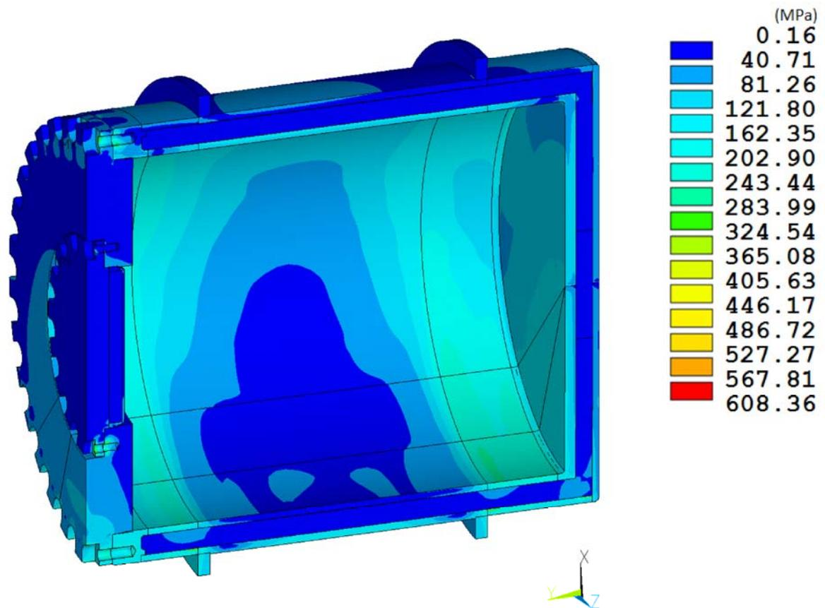
**Figure 8-13. RT-100 HAC Side Drop Stress Intensity Results.**
