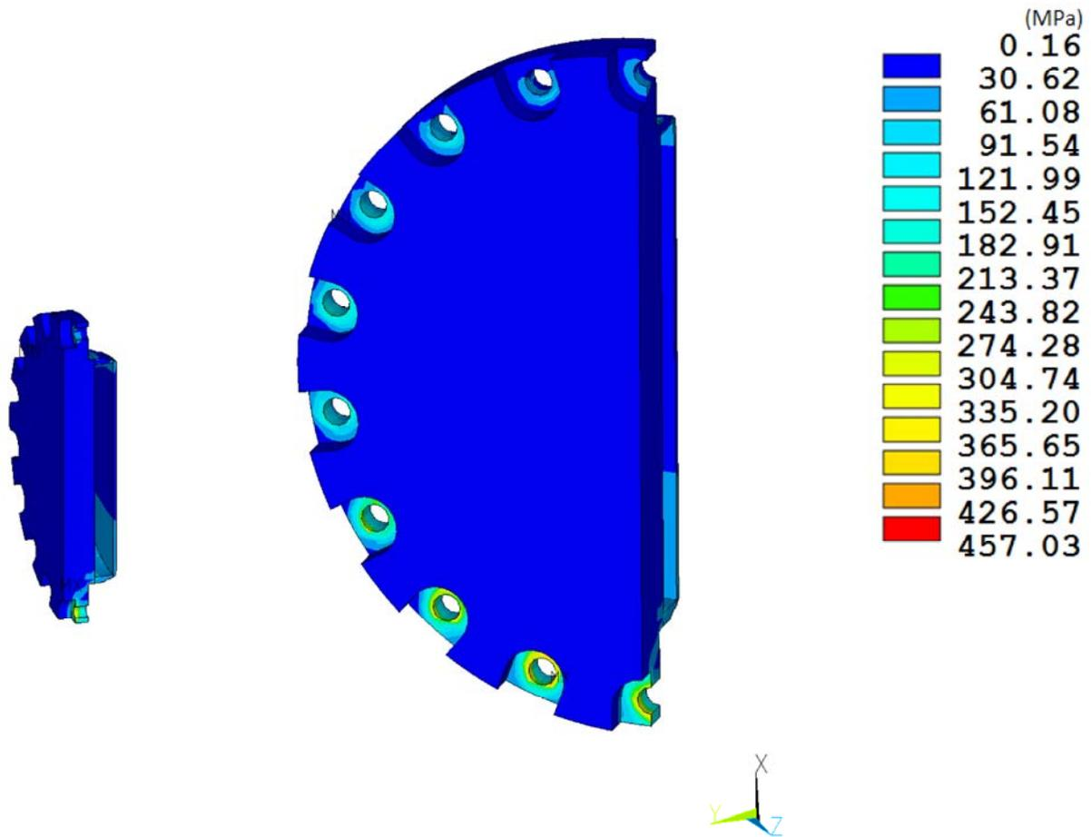
**Figure 8-18. RT-100 Inner Lid HAC Side Drop Stress Intensity Results.**
