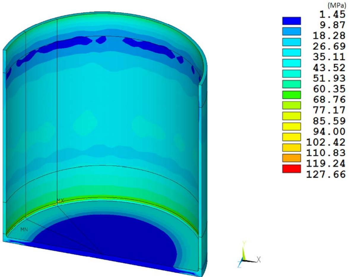
**Figure 8-20. RT-100 Inner Shell HAC End Drop Stress Intensity Results.**
