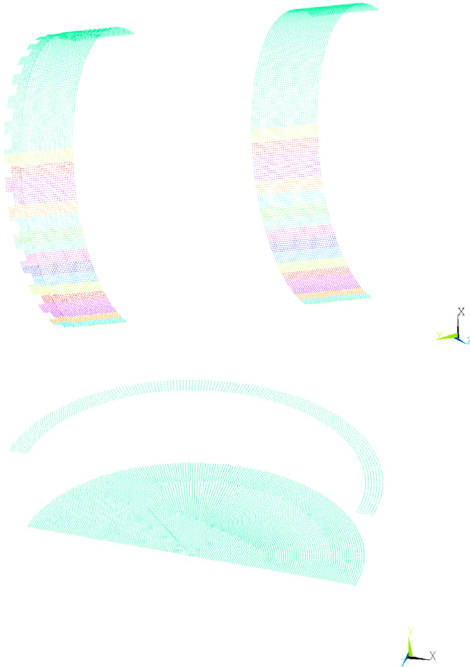
**Figure 7-3. Gap Elements used to Represent the Impact Limiters for side and end drop configurations.**
