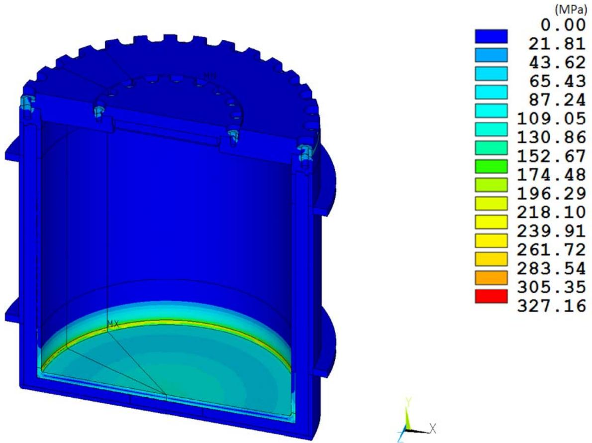
**Figure 8-25. RT-100 HAC Pressure Stress Intensity Results.**
