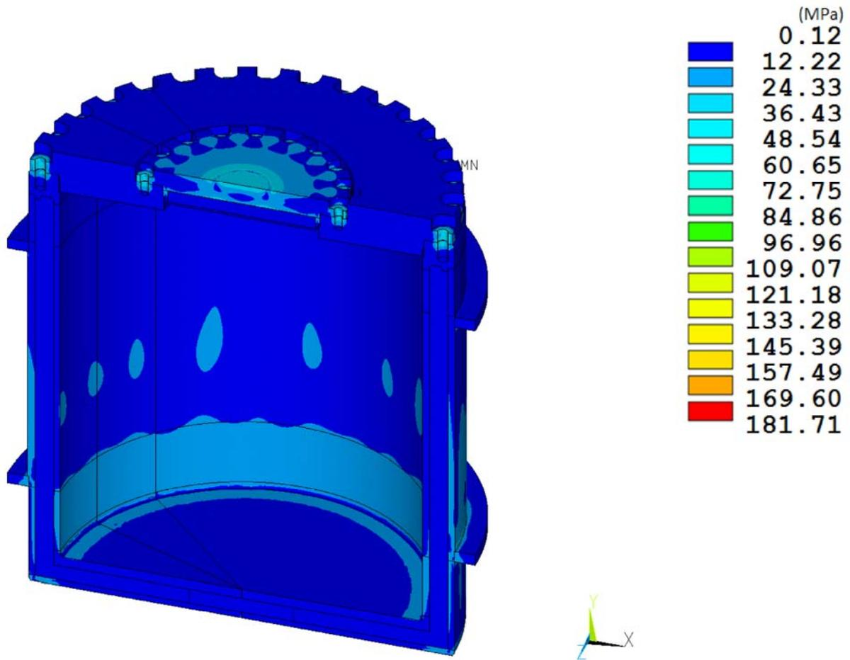
**Figure 8-7. RT-100 NCT Bottom Drop Stress Intensity Results.**
