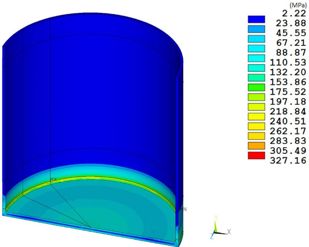
**Figure 8-26. RT-100 HAC Inner Shell Pressure Stress Intensity Results.**
