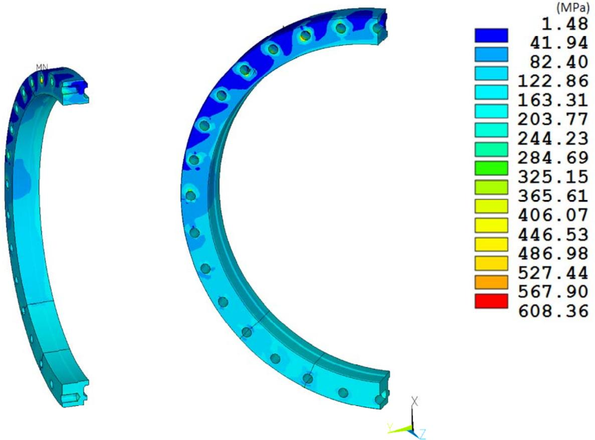
**Figure 8-16. RT-100 Flange HAC Side Drop Stress Intensity Results.**
