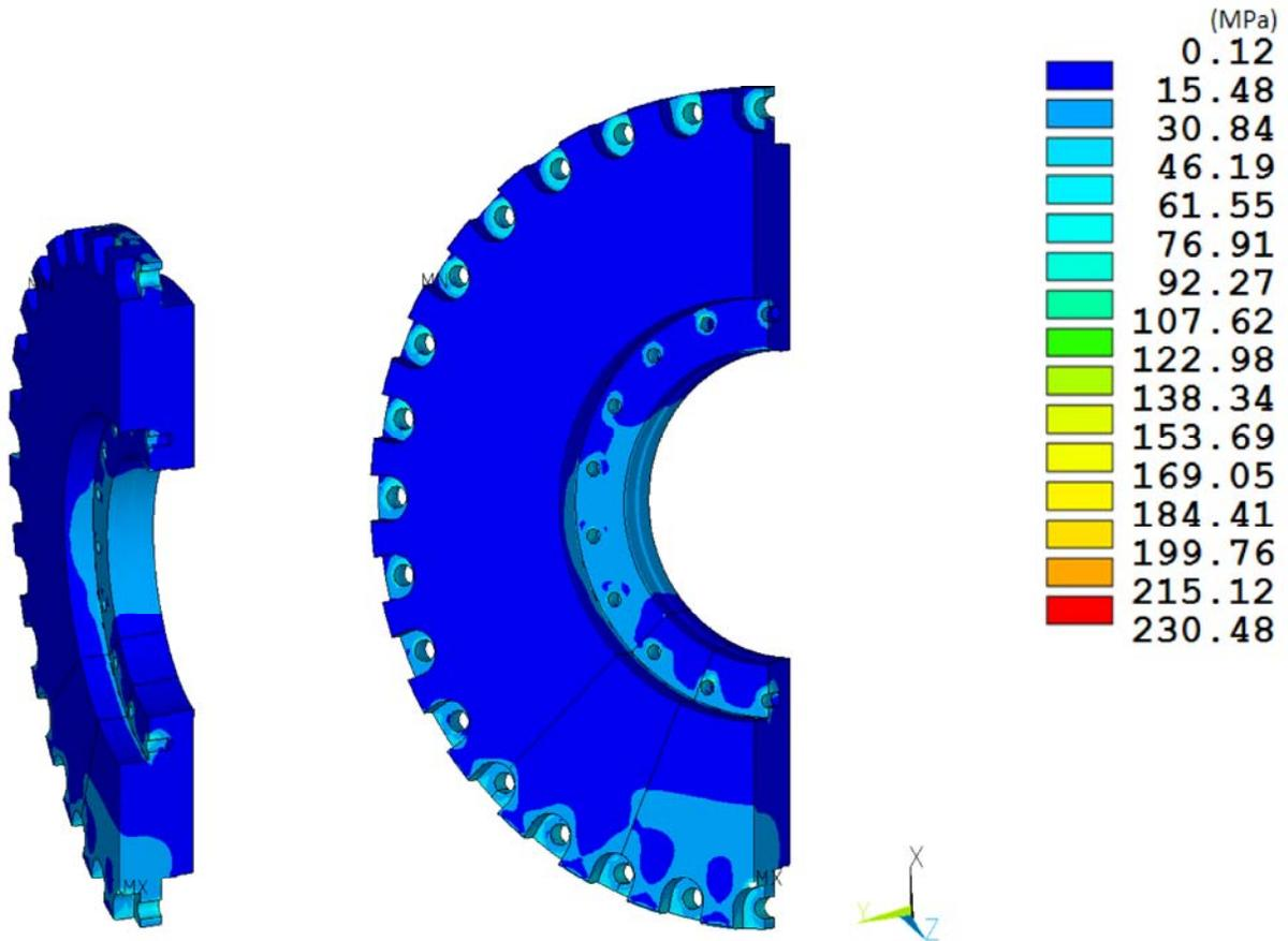
**Figure 8-5. RT-100 Outer Lid NCT Side Drop Stress Intensity Results.**
