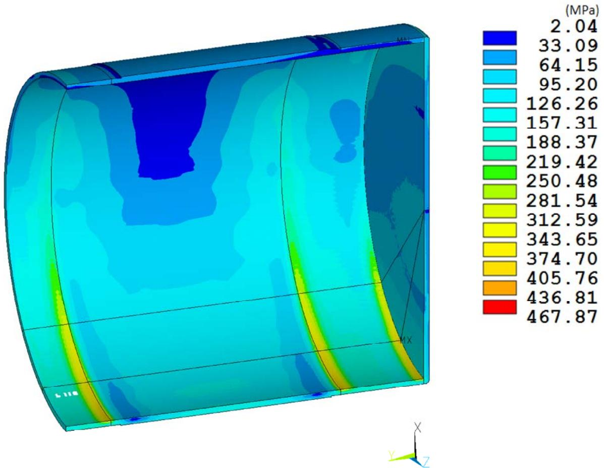
**Figure 8-15. RT-100 Outer Shell HAC Side Drop Stress Intensity Results.**
