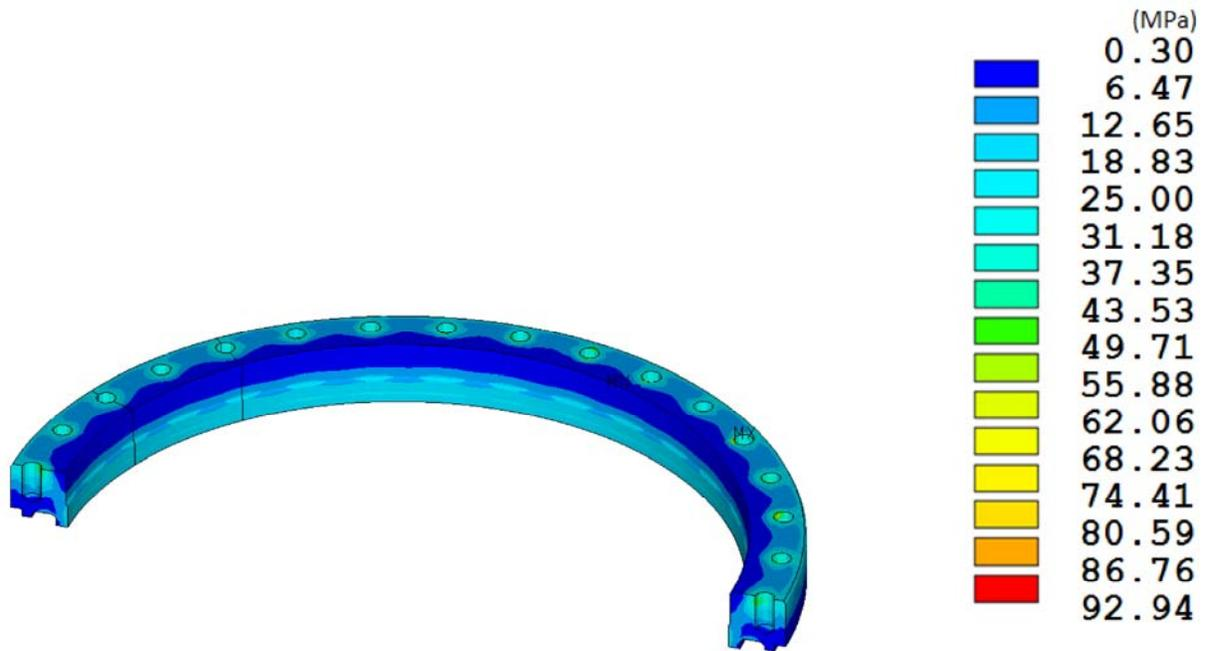
**Figure 8-28. RT-100 HAC Flange Pressure Stress Intensity Results.**
