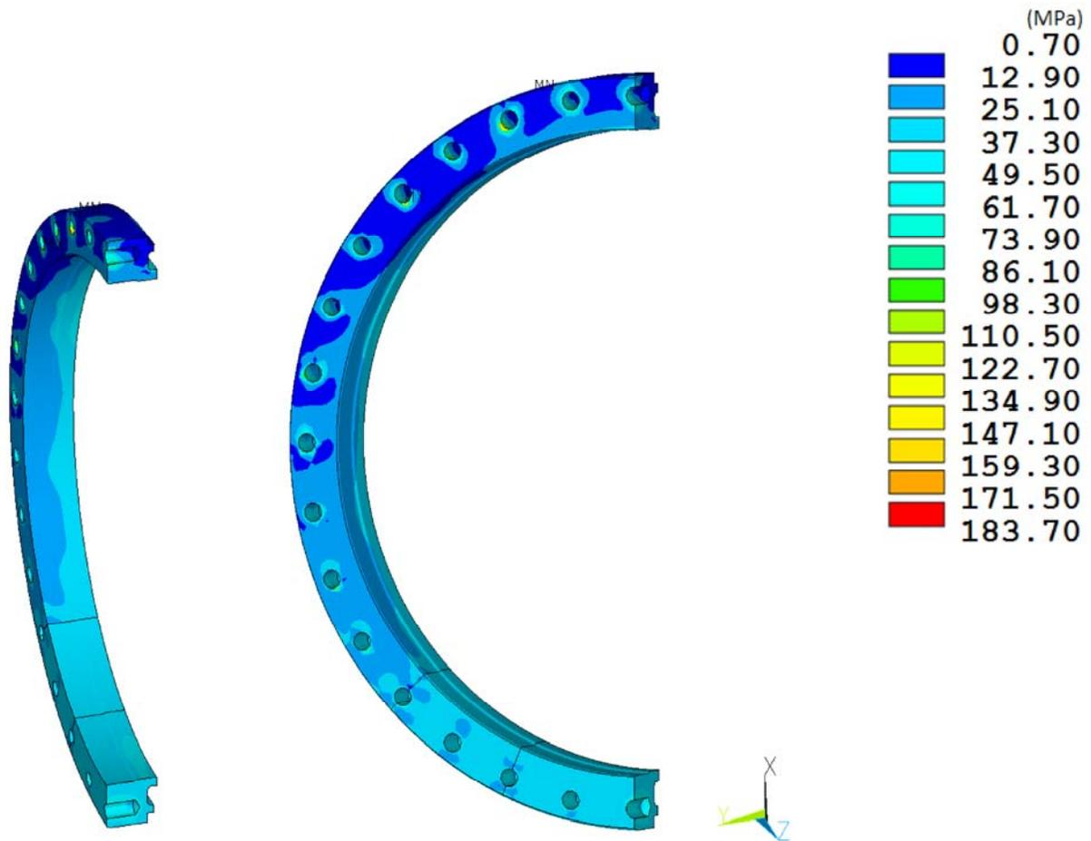
**Figure 8-4. RT-100 Flange NCT Side Drop Stress Intensity Results.**
