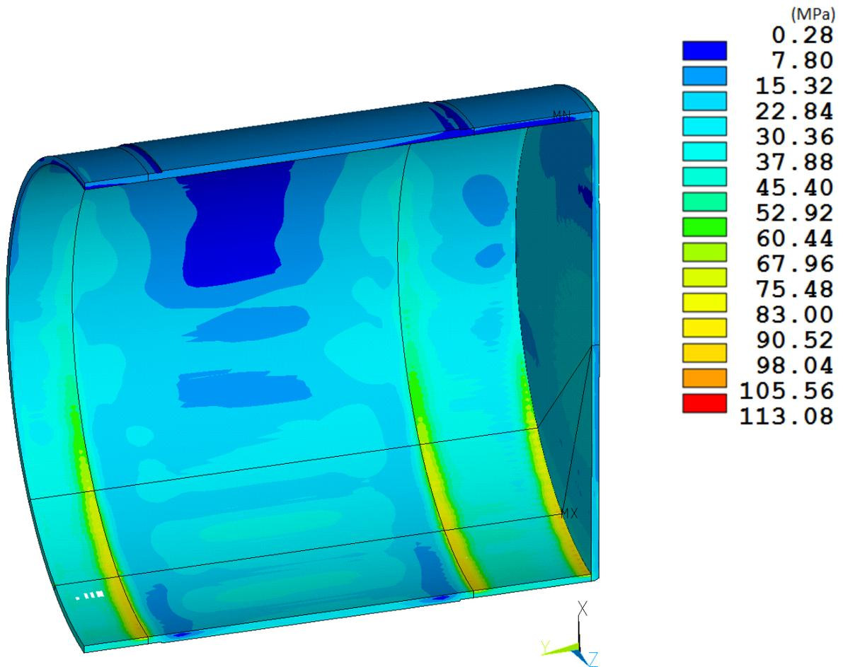
**Figure 8-3. RT-100 Outer Shell NCT Side Drop Stress Intensity Results.**
