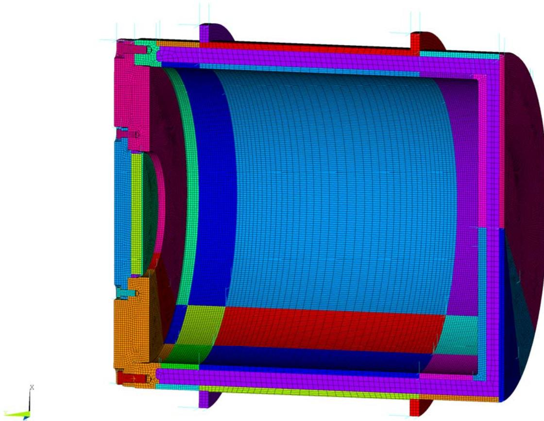
**Figure 7-2. RT-100 ANSYS Finite Element Model.**
