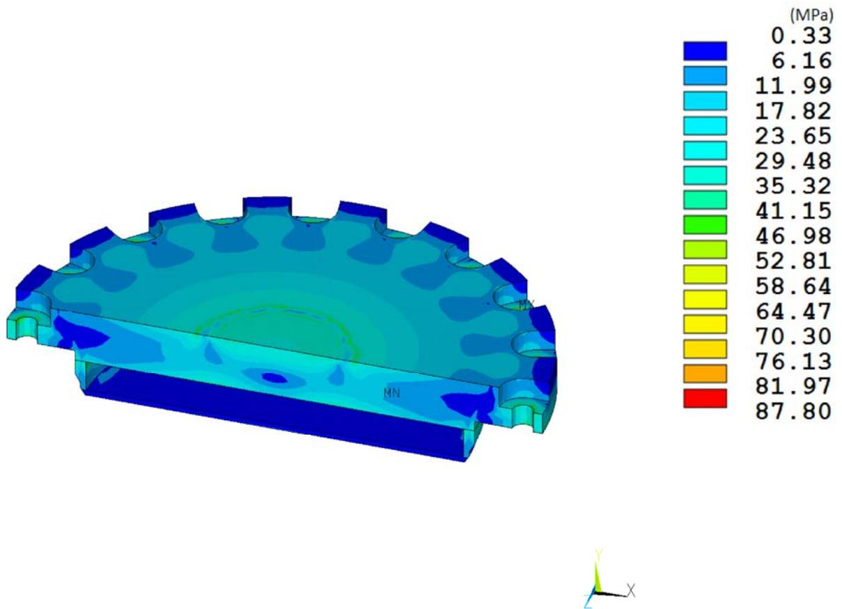
**Figure 8-12. RT-100 Inner Lid NCT End Drop Stress Intensity Results.**
