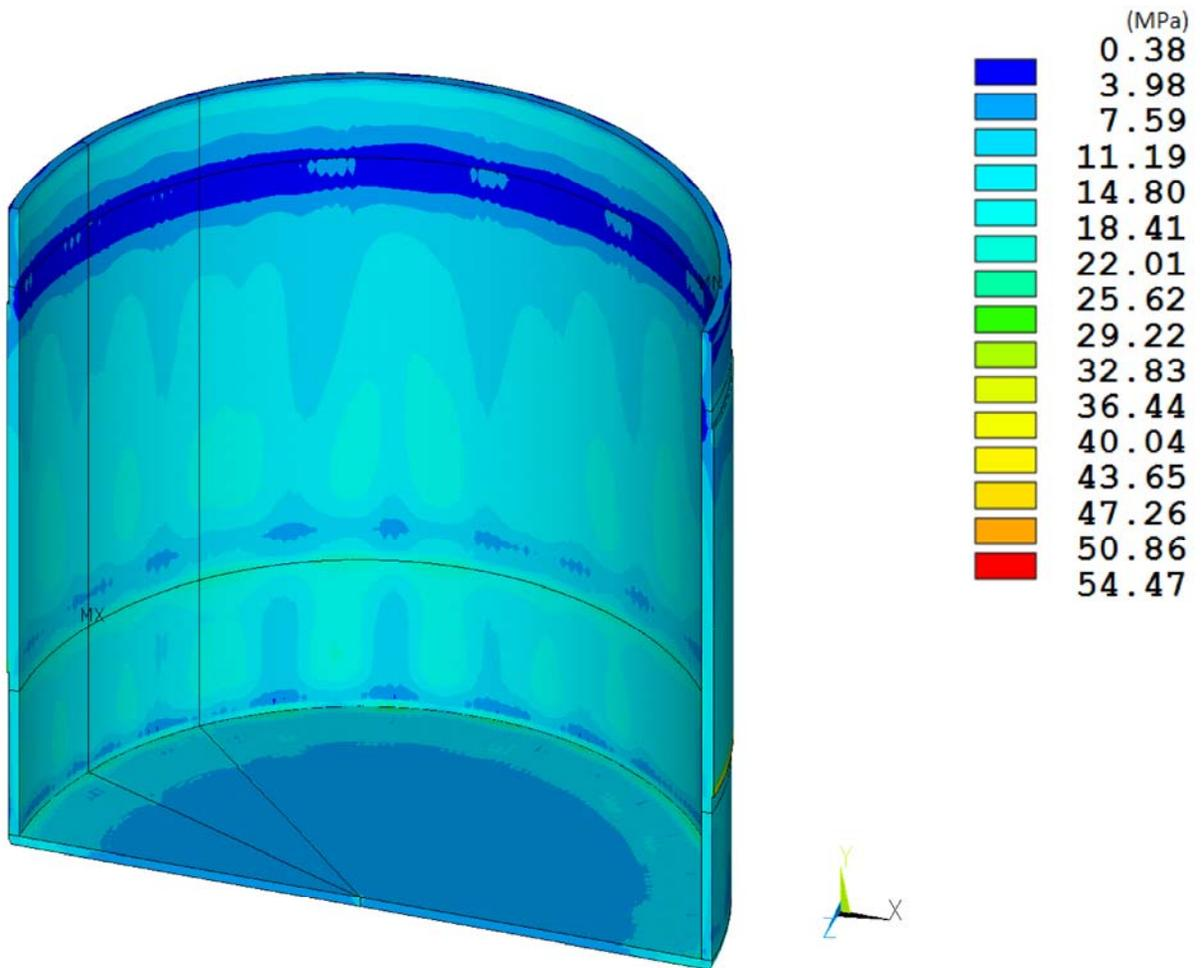
**Figure 8-9. RT-100 Outer Shell NCT End Drop Stress Intensity Results.**
