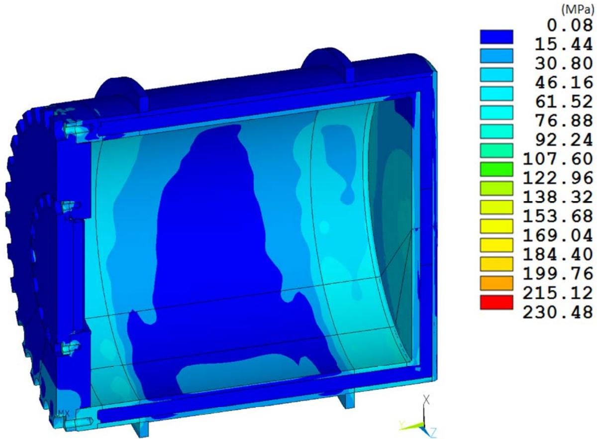
**Figure 8-1. RT-100 NCT Side Drop Stress Intensity Results.**
