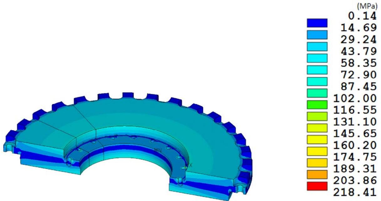
**Figure 8-23. RT-100 Outer Lid HAC End Drop Stress Intensity Results.**
