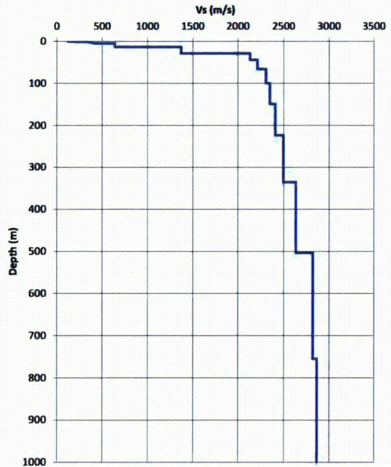
Shear Wave Velocity Profile Determined at Station ET.SWET by SASW Method
