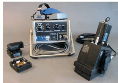
Figure 1. Industrial MOI system for inspection of aging aircrafts. [Shih et al]
