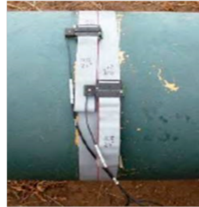
Figure 16. A guided wave sensor that can perform wall thinning inspection of piping [courtesy of G. M. Light, SwRI].
