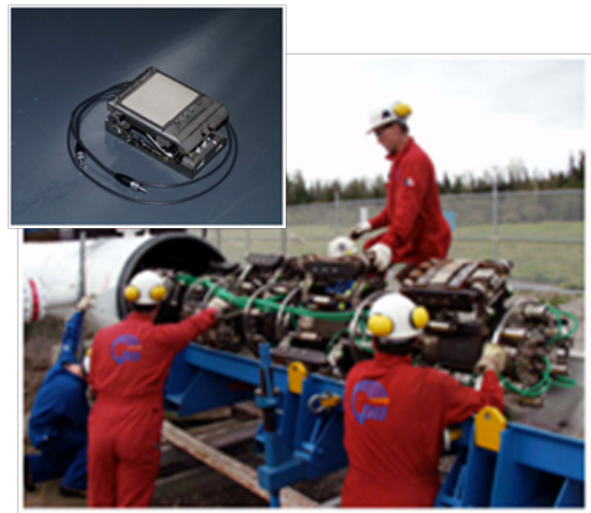
Figure 12. Prototype EmatScan CD pig for inspection of pipelines. Also shown (top corner) is the SH-wave probe in a spring loaded suspension [http://www.ndt.net/article/wcndt2004/pdf/non-contact_ultrasonics/599_salzburger.pdf] .
