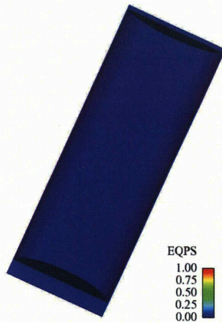
Figure III-16 Plastic strain in the interior welded canister of the Rail-Steel cask from the corner impact at 48 kph (30 mph)
