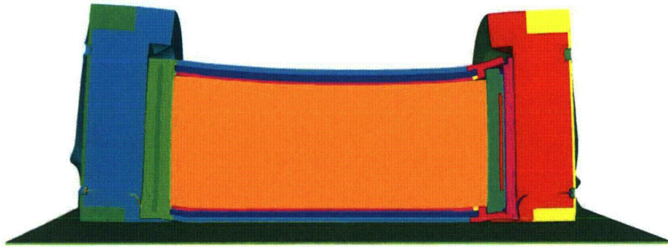
Figure III-40. Rail-Lead cask side impact at 193 KPH (120 MPH)
