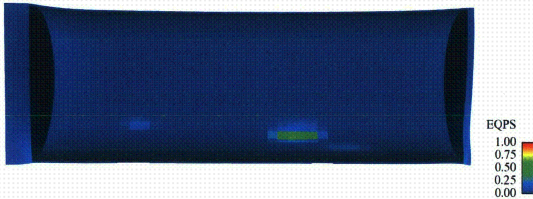
Figure III-23. Plastic strain in the interior welded canister of the Rail-Steel cask from the side impact at 193 KPH (120 MPH)
