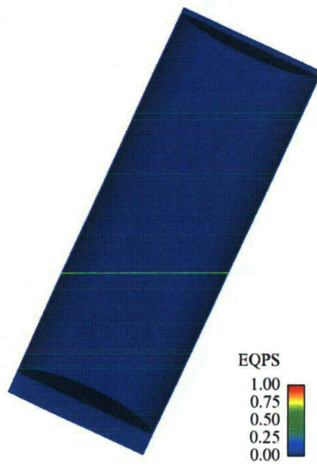
Figure III-16. Plastic strain in the interior welded canister of the Rail-Steel cask from the corner impact at 48 KPH (30 MPH)
