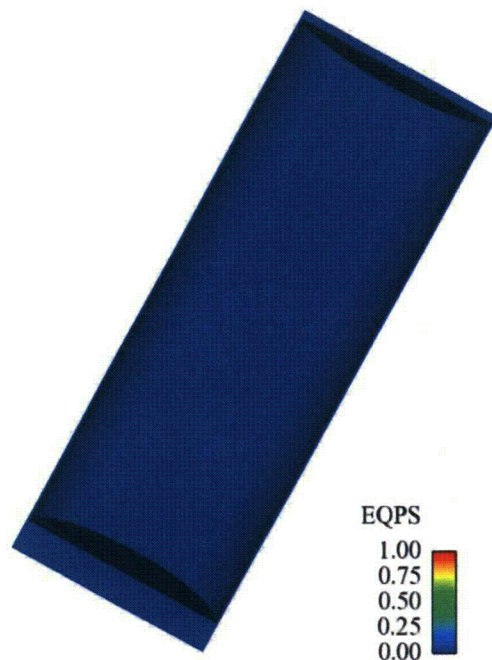
Figure III-17. Plastic strain in the interior welded canister of the Rail-Steel cask from the corner impact at 97 KPH (60 MPH)
