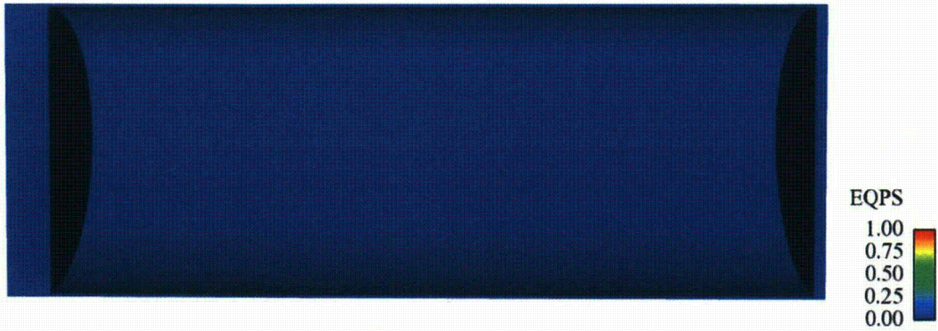
Figure III-21. Plastic strain in the interior welded canister of the Rail-Steel cask from the side impact at 97 KPH (60 MPH)
