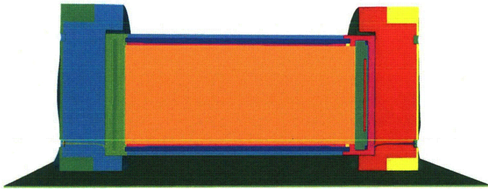
Figure III-37. Rail-Lead cask side impact at 48 KPH (30 MPH)
