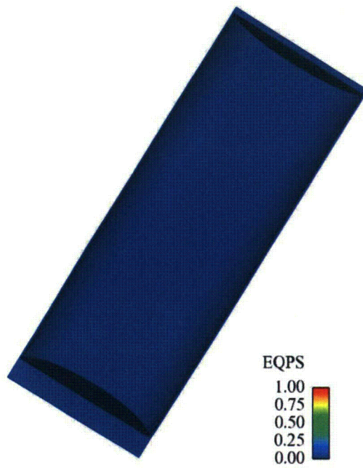
Figure III-18. Plastic strain in the interior welded canister of the Rail-Steel cask from the corner impact at 145 KPH (90 MPH)
