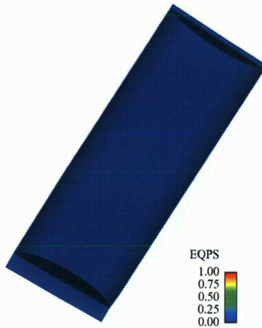
Figure III-19. Plastic strain in the interior welded canister of the Rail-Steel cask from the corner impact at 193 KPH (120 MPH)
