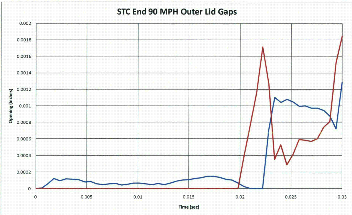
Figure III-46. Gaps in the inner and outer lids of the Rail-Lead cask from the end impact at 145 KPH (90 MPH)
