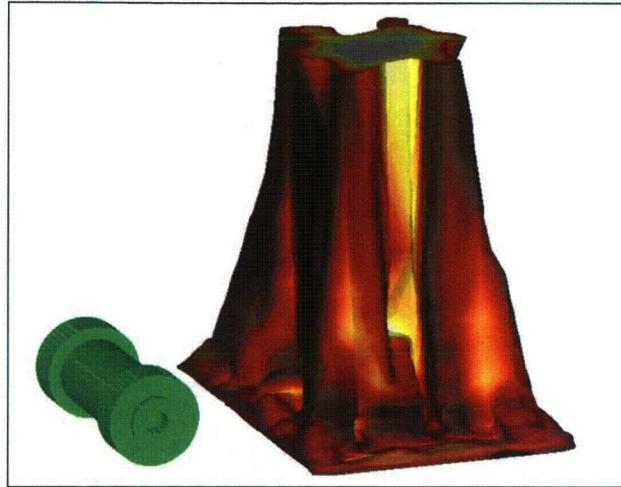
**Figure 4-2. Cask lying on ground 3 meters from pool fire**
