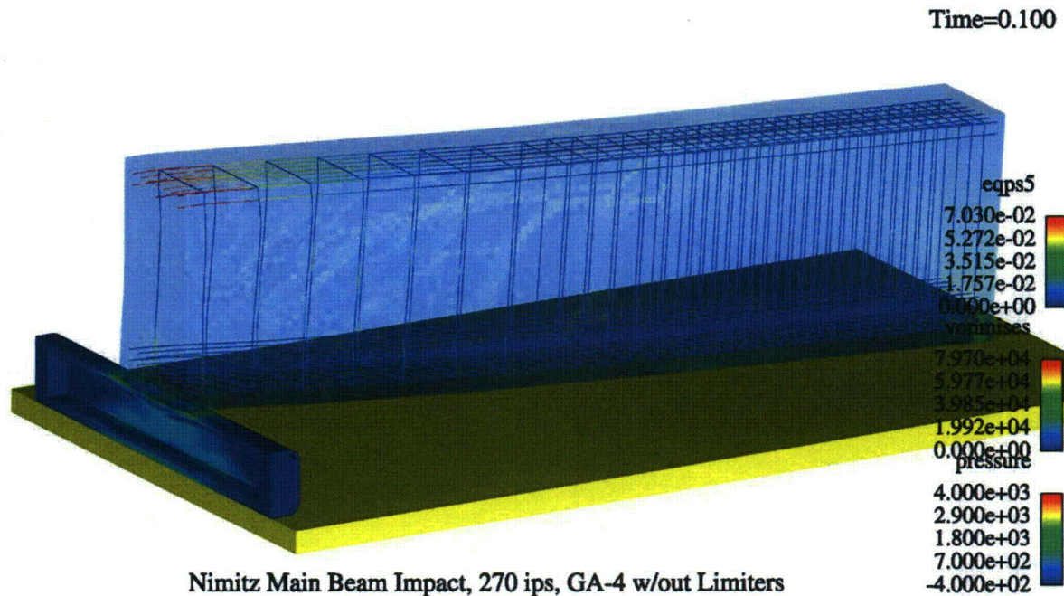
Figure 3-19. Results of a finite element simulation of an elevated freeway collapse onto a GA-4 spent fuel cask (from Ammerman and Gwinn 2004)
