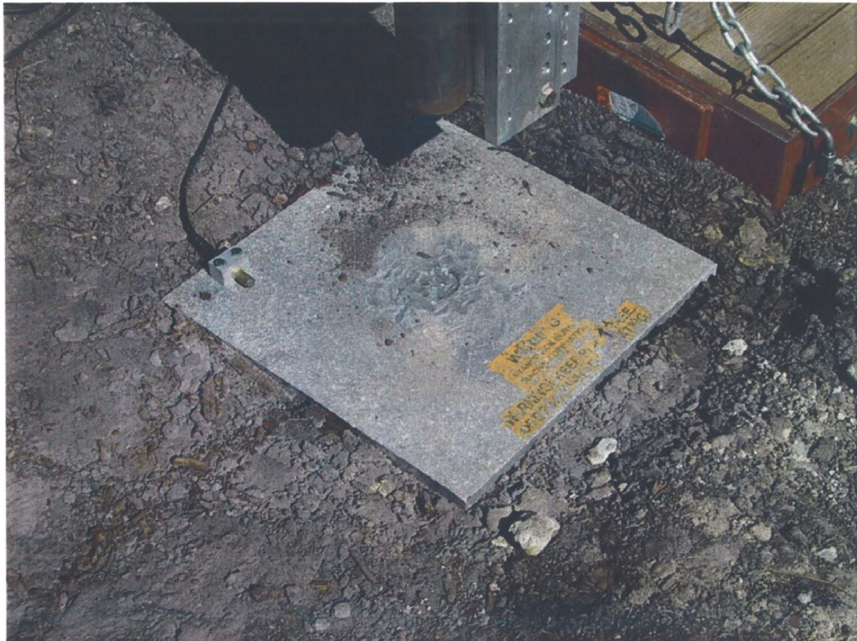
Figure 3: Downhole P-wave striking plate with hammer switch
