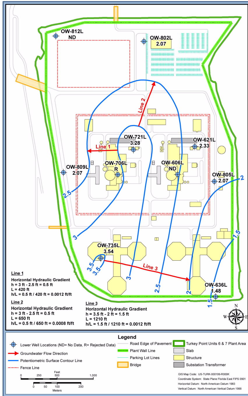
Figure 2.4.12-226 Biscayne Aquifer Potentiometric Surface Map, Lower Monitoring Interval, October 5, 2008 (Sheet 1 of 2) High Tide
