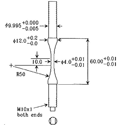
Cylindrical 12-mm diameter smooth, test specimens
