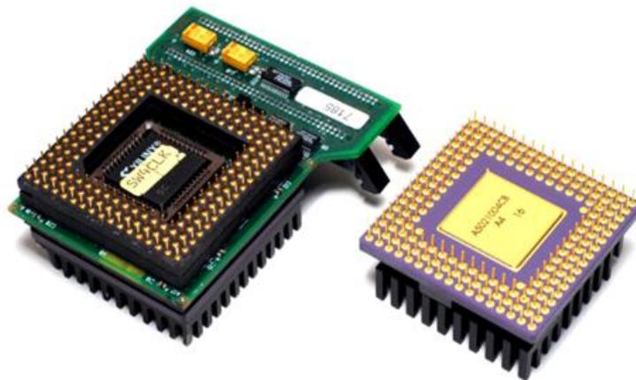
Figure 7-2 In-circuit Emulator (ICE) pod
