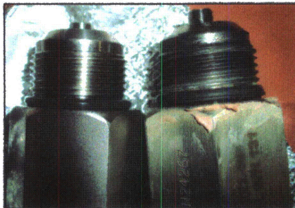
New unfired explosive (left) and the failed explosive (right)
