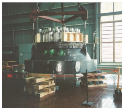
Replacement Reactor Vessel Head for R.E. Ginna Nuclear Power Plant post-Davis-Besse
