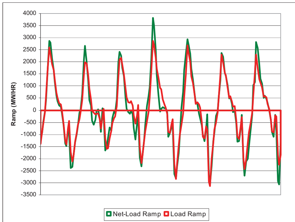
Figure 5.21: 2018 Hourly Net-Load Ramps VS Load Ramps for the Week of the Peak Load
