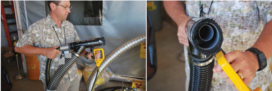
Figure 2-1. Blast N'Vac as assembled for testing (left). Close-up of Blast N'Vac vacuum head (right).
