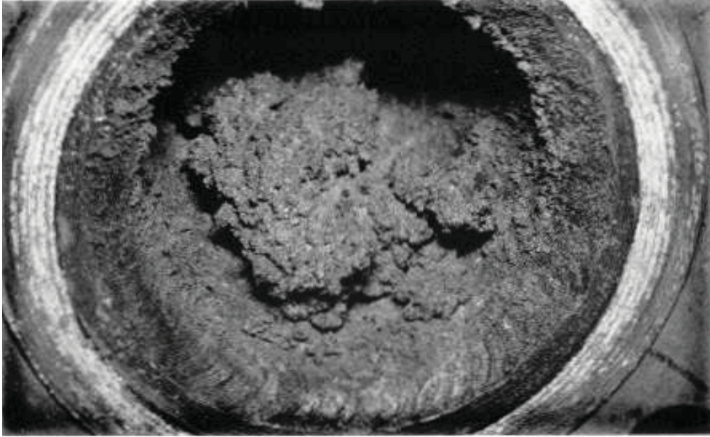
Figure D-7 Test LA3C, downstream end of pipe section 5 showing large bend deposit
