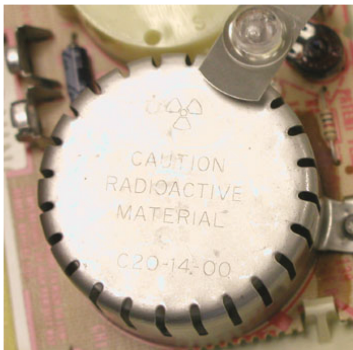
Figure 6.2 Am-241 Smoke Detector Source
