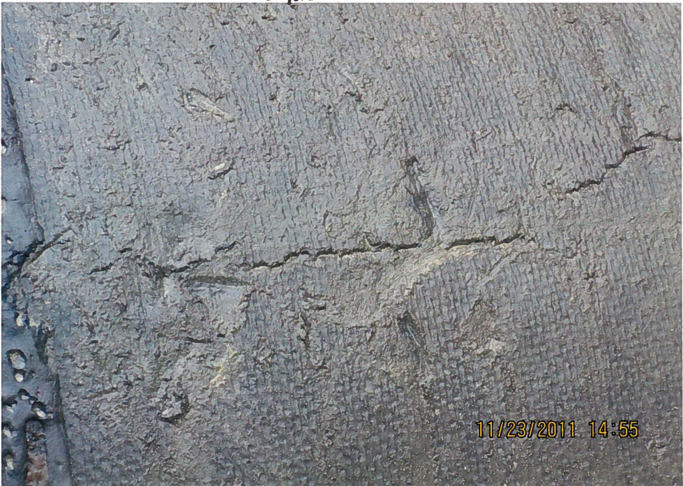
FINE CRACKS IN TOP LAYER OF WRAP ↓
