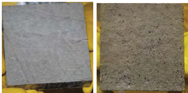
Figure 5-1. Test coupon surfaces before (left) and after (right) treatment with the Blast N'Vac.
