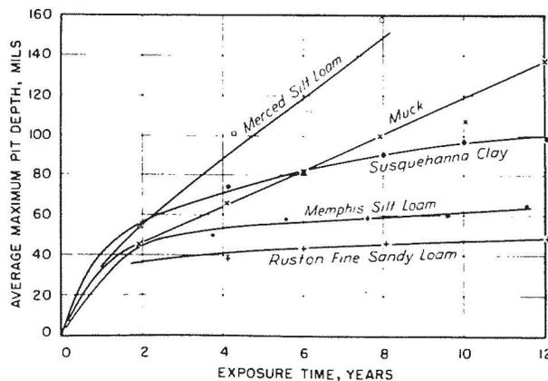
FIGURE 11. Pit-depth-time curves for wrought ferrous pipe.
