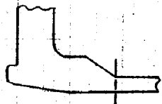
RADIAL GRADIENT AT THIN SECTION OF OUTLET NOZZLE WHERE TAPER ENDS PLANT UNLOADING
