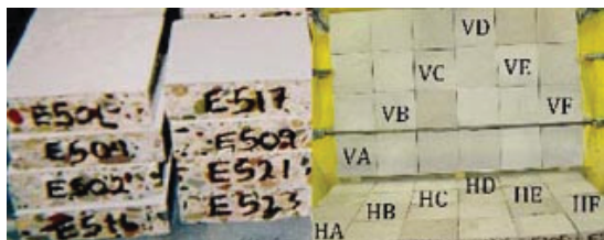
Figure 2. Concrete Coupons (left) and Test Stand With Contaminated Coupons (right) - H and V indicate horizontal and vertical orientation, respectively, and A–F indicate the surface positions
