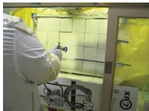
Figure 1. Applying the Coating with a Sprayer
