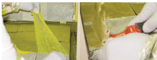
Figure 3. Removal of Stripcoat TLC Free™ (left) and Removal of Orion™ SC (right)
