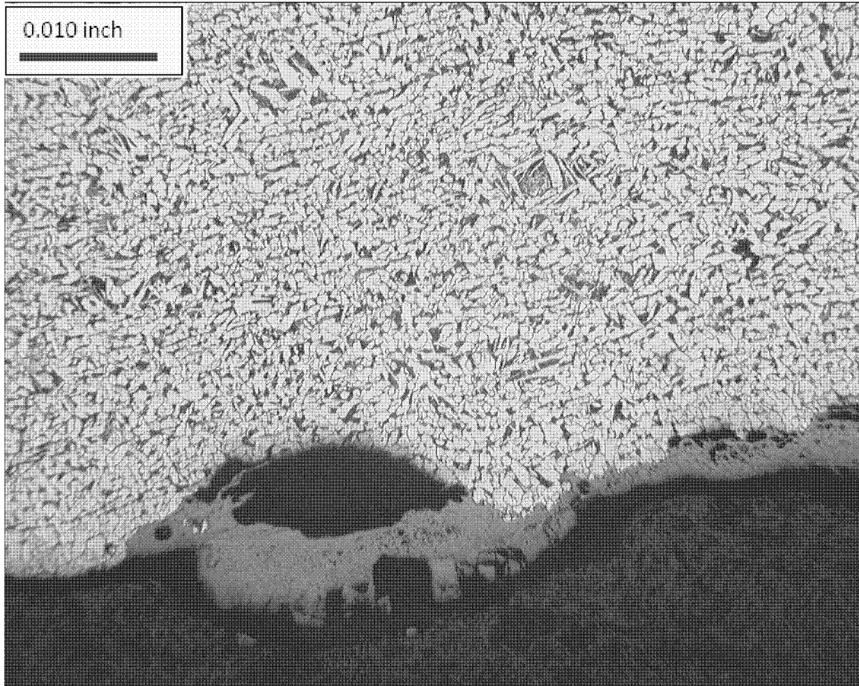
Figure 44 - Microstructure of pipe at inside surface showing blistered corrosion product over a corrosion pit.
