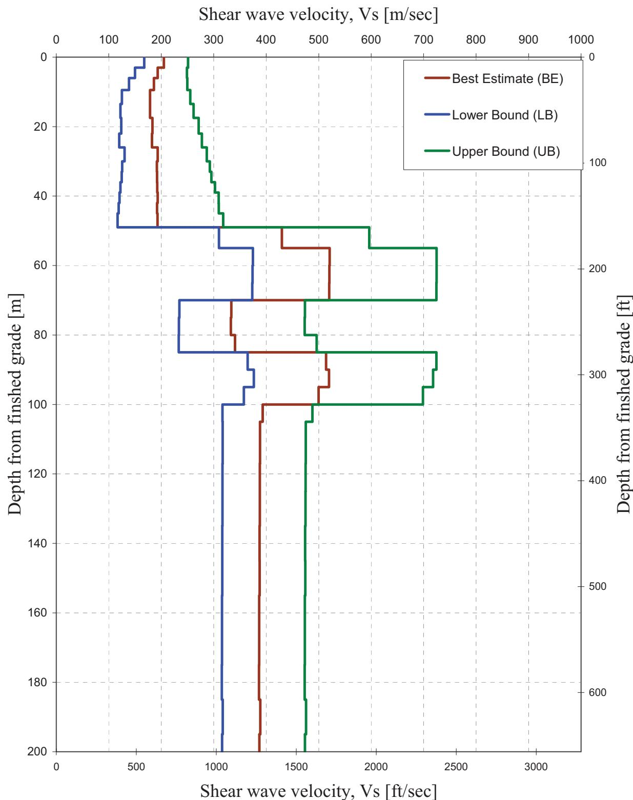
**Figure 2.5-232—{CCNPP Unit 3 Strain - Compatible Profiles for NI Common Basemat Structures - RB26 Soil Column}**
