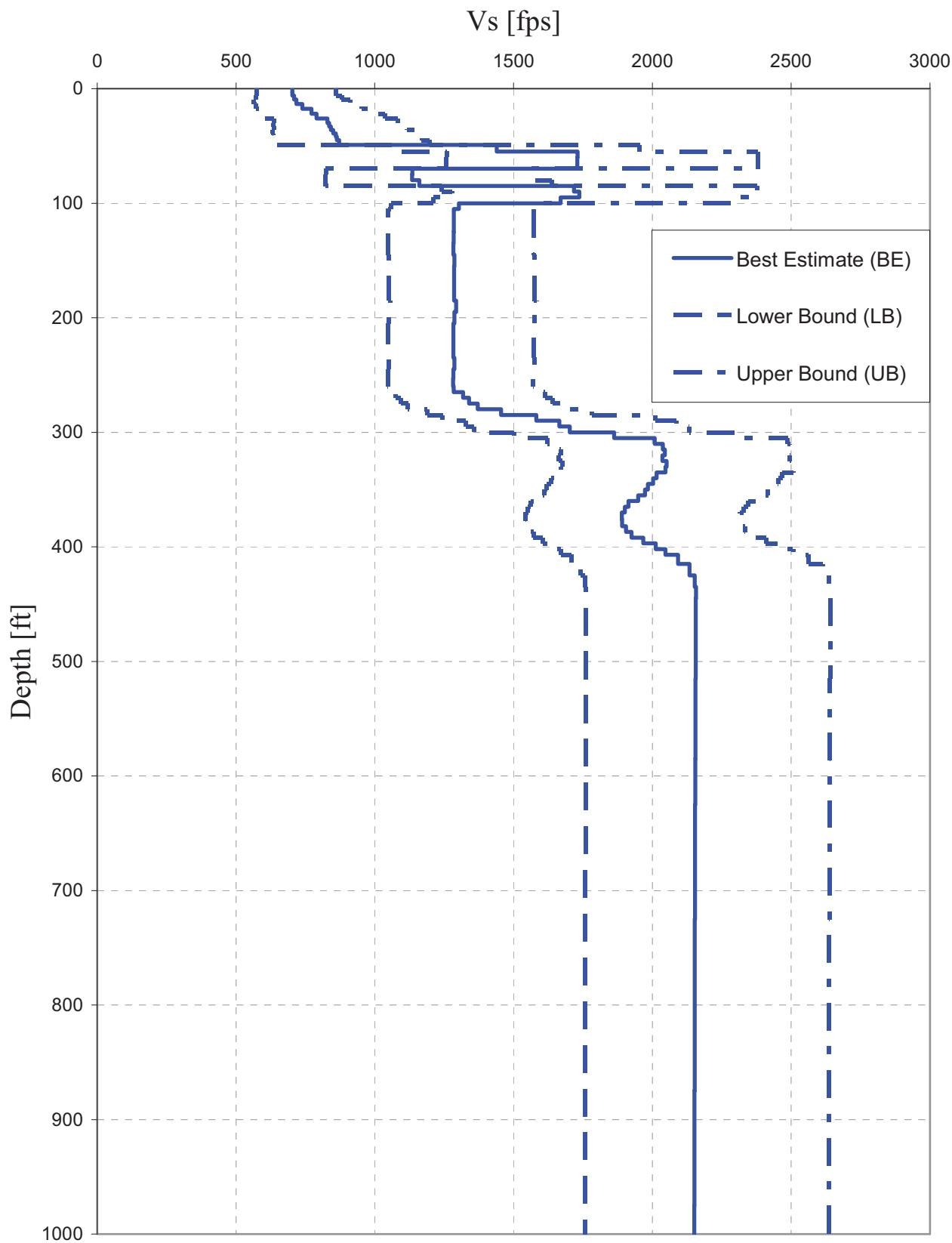
**Figure 2.5-234— {Shear-Wave Velocity Profiles Strain-Compatible with FIRS for the RB26 Soil Column}**
