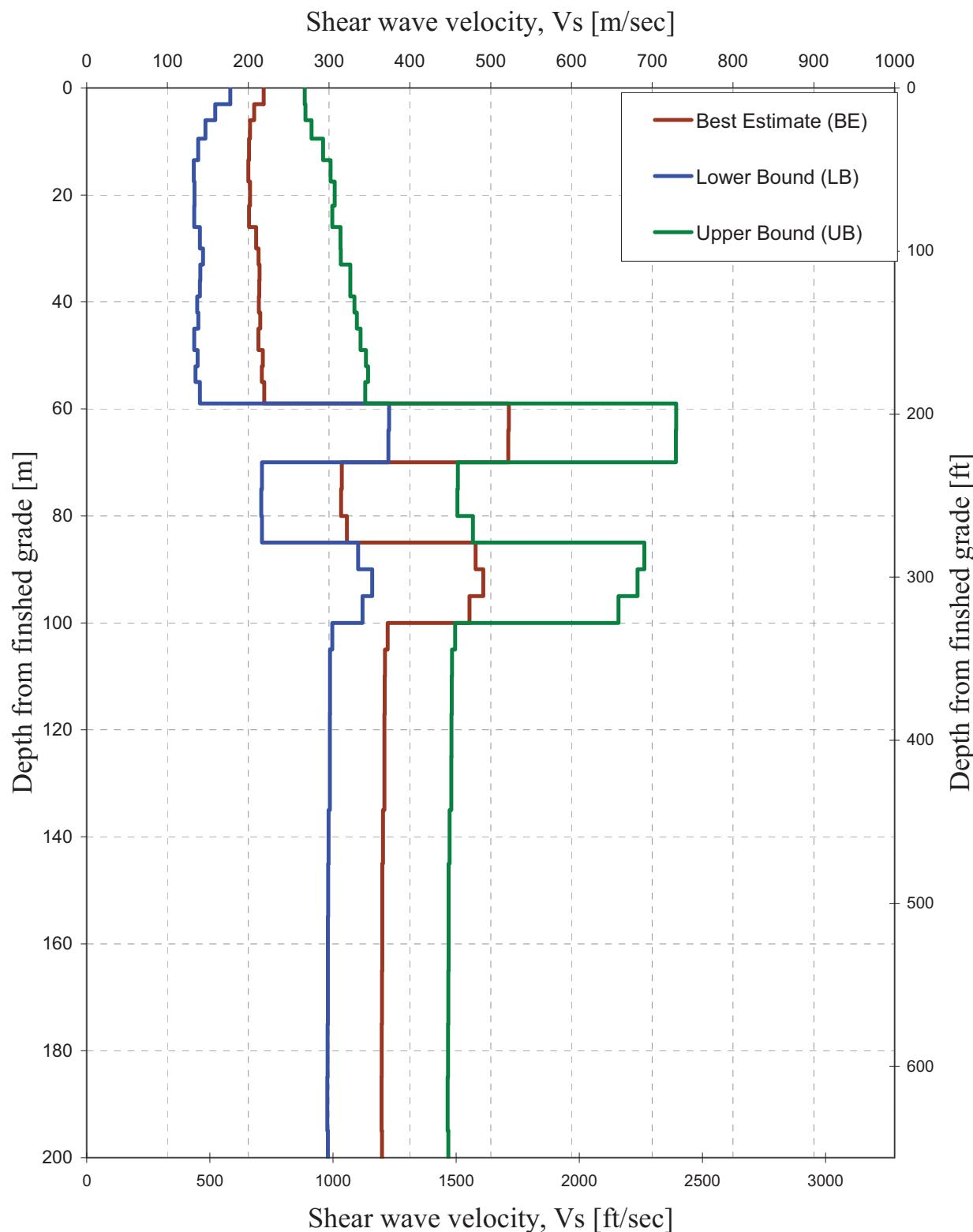
**Figure 2.5-233—{Shear-Wave Velocity Profiles Strain-Compatible with FIRS for the RB36 Soil Column}**
