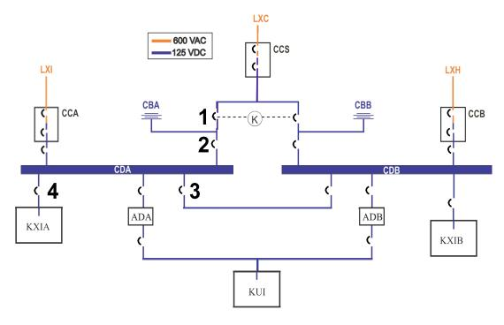
Which ONE of the following describes which of the DC breakers (labeled 1, 2, 3, 4 in the drawing above) will cause an alarm to be received in the Control Room when the breakers OPEN?
