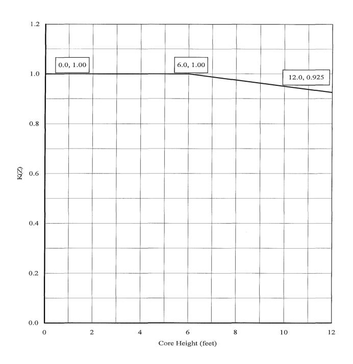
Figure 5.1-3 (Page 1 of 1)  $F_{Q}T \ NORMALIZED \ OPERATING \ ENVELOPE, \ K(Z)$
