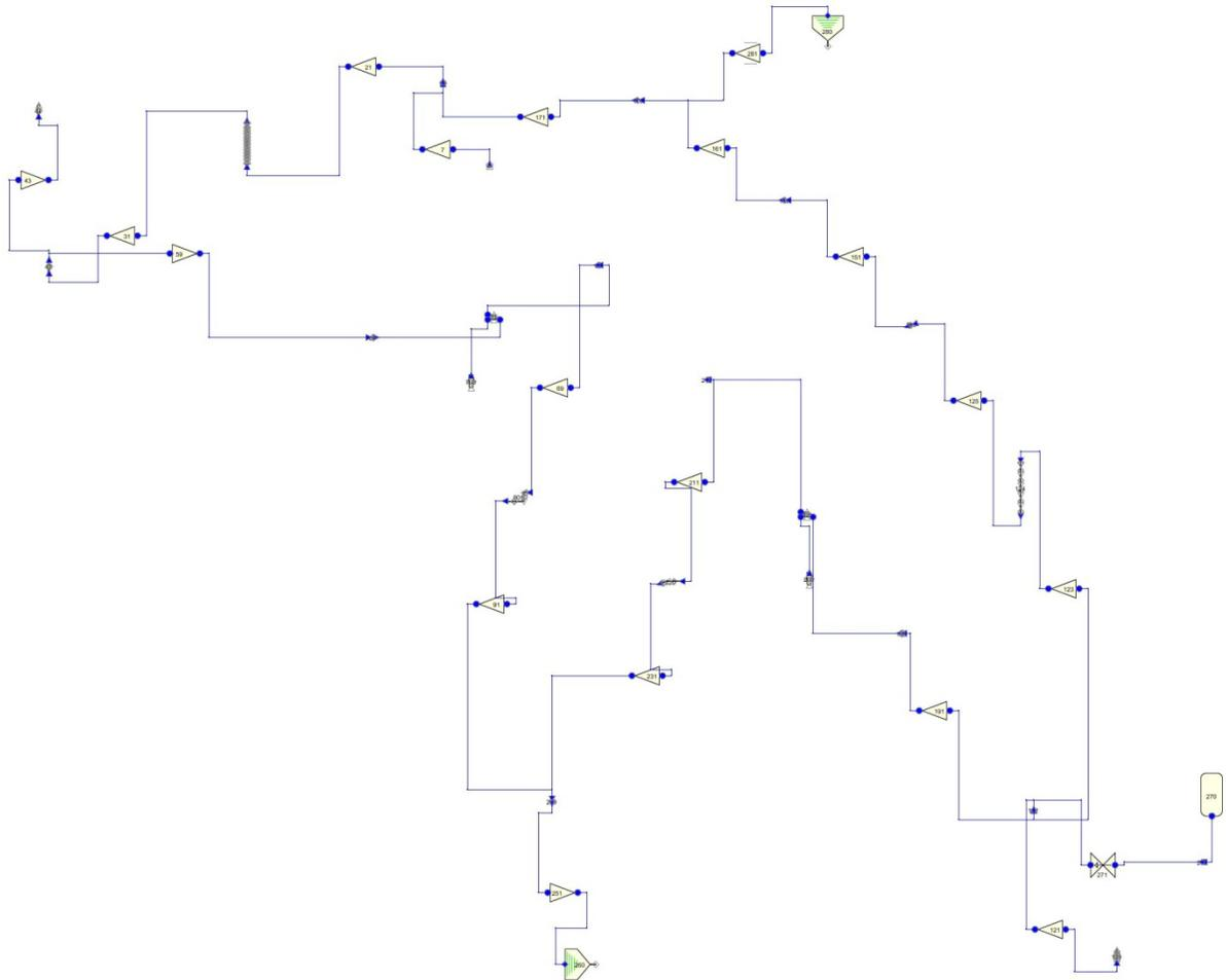
**Figure 7 SNAP hydrodynamic component view for RELAP5 input model of ACHILLES rig - original**
