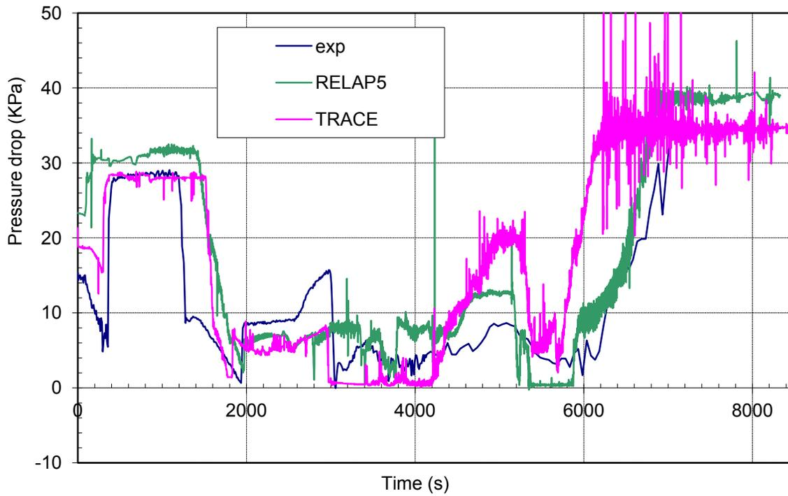
**Figure 31 Loop 1 Seal Downflow Side Differential Pressure**
