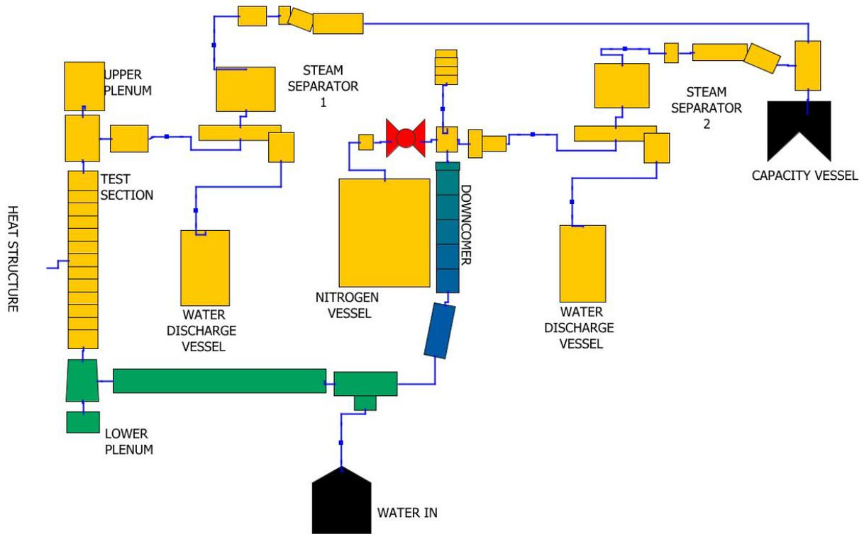
Figure 12 Basic animation model for RELAP5 model of ACHILLES rig
