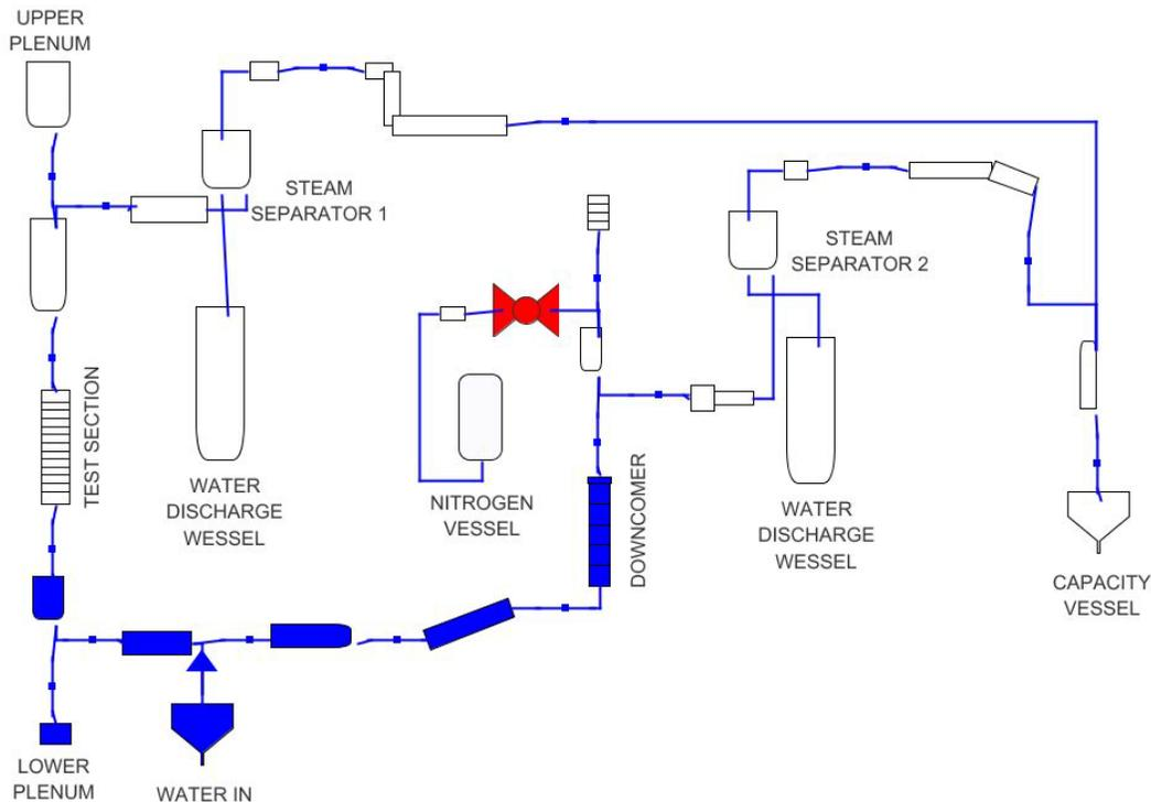
Figure 9 Basic animation model for RELAP5 model of ACHILLES rig
