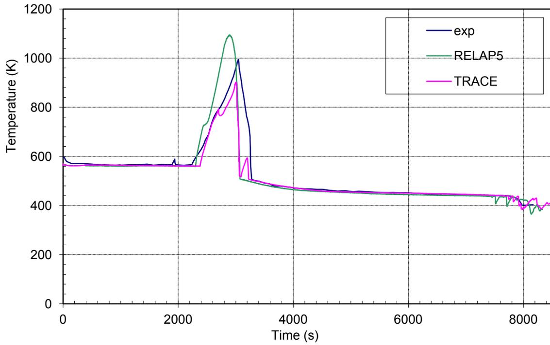
**Figure 29 Maximum heater rod surface temperature – BETHSY 9.1b**
