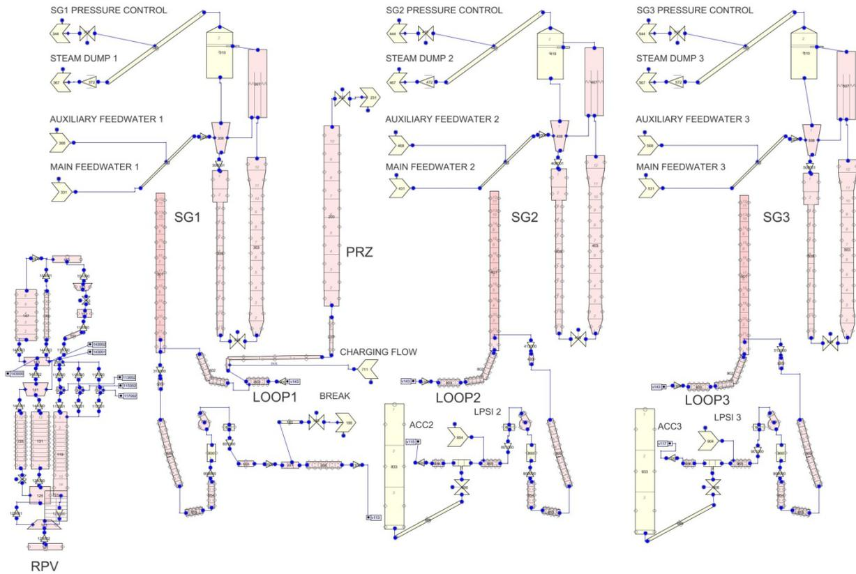
Figure 22 SNAP hydrodynamic component view for converted (and adapted) TRACE input model of BETHSY facility
