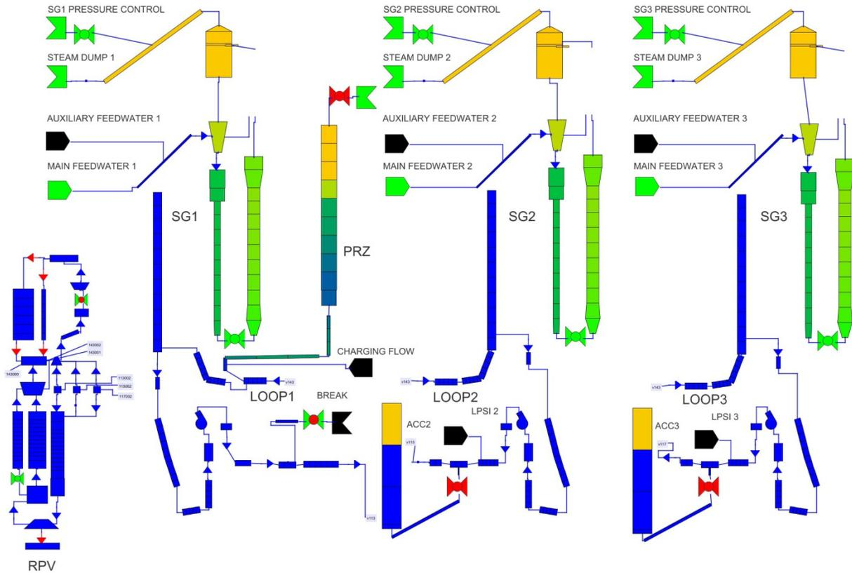
**Figure 24 SNAP basic animation model for TRACE model of BETHSY facility**
