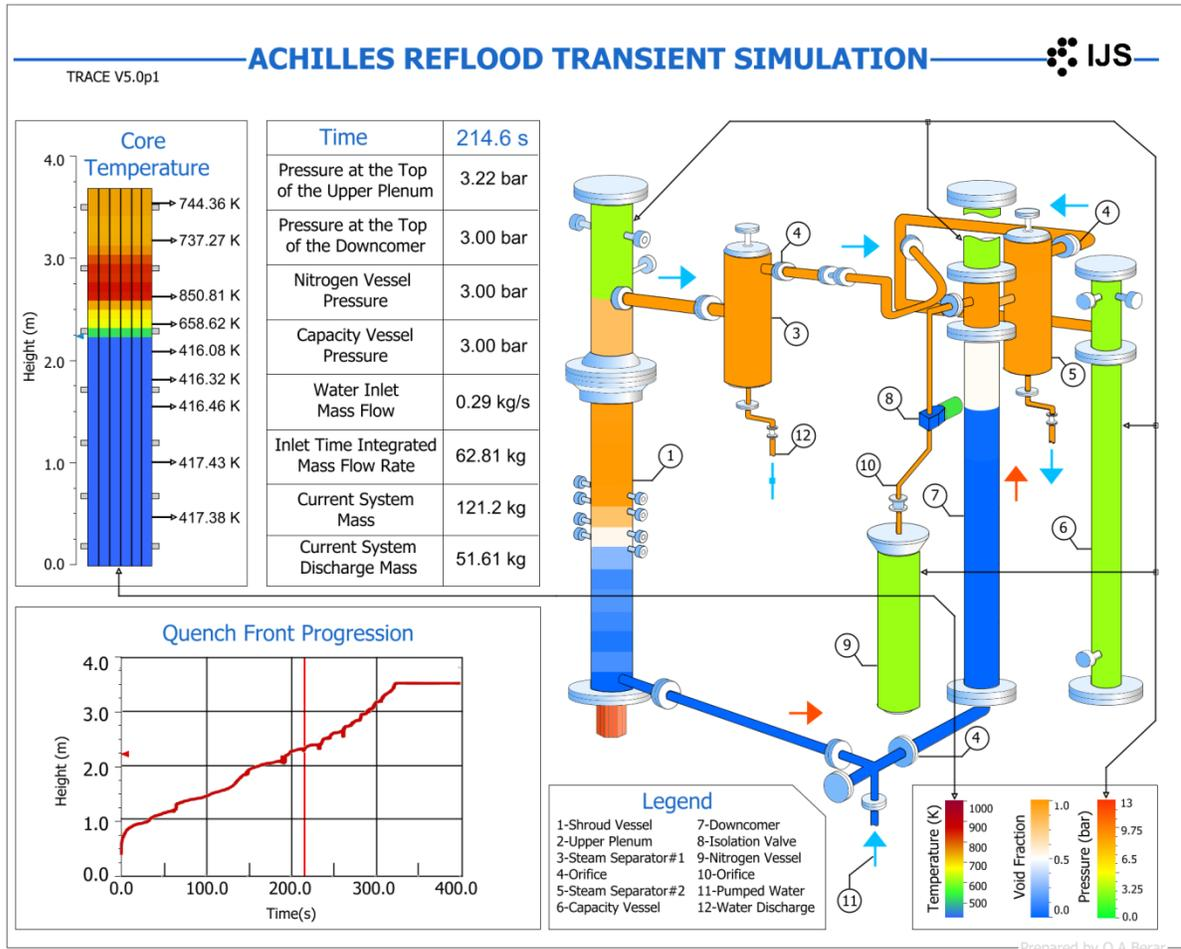
**Figure 13 SNAP additional animation mask for the Achilles TRACE model**
