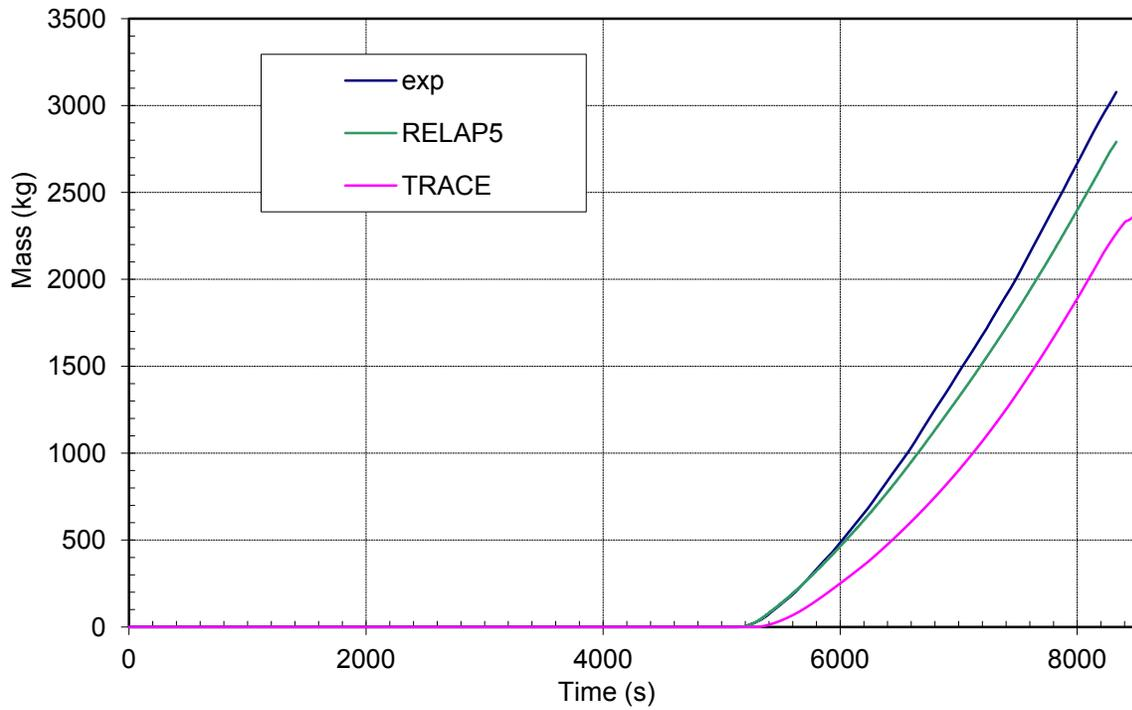
**Figure 33 Integrated low pressure injection system mass – BETHSY 9.1b**
