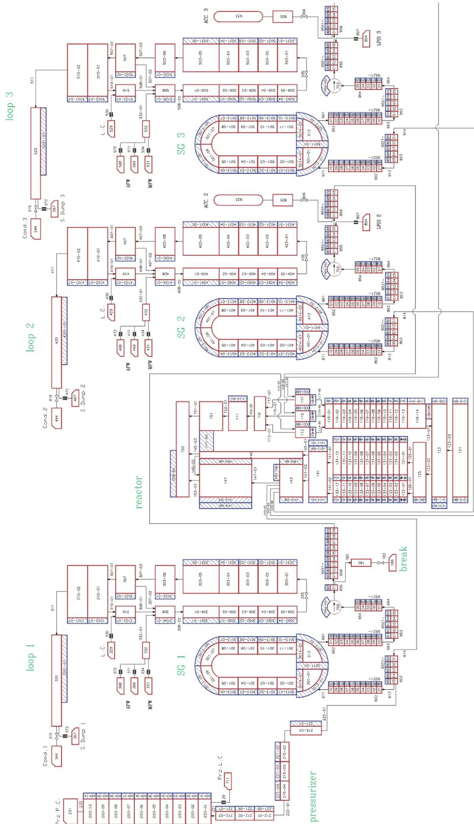
Figure 5 RELAP5/MOD3.1 input model of BETHSY facility.
