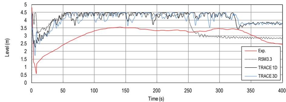
**Figure 18 Downcomer collapsed liquid level**
