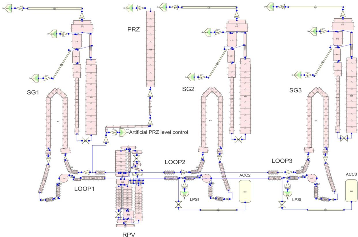
**Figure 20 SNAP hydrodynamic component view for RELAP5 input model of BETHSY facility – arranged**
