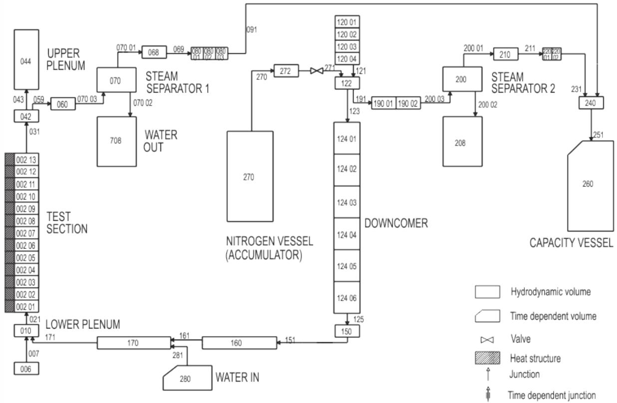
Figure 3 Achilles facility RELAP5 nodalization (Ref. 9)
