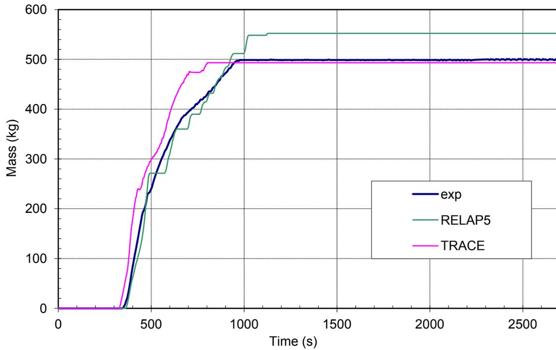
**Figure 46 Integrated accumulators injected mass – BETHSY 6.2TC**
