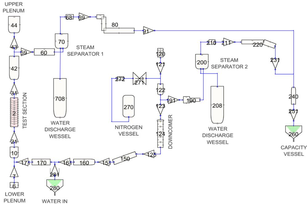
**Figure 8 SNAP hydrodynamic components view for RELAP5 input model of ACHILLES rig – arranged**
