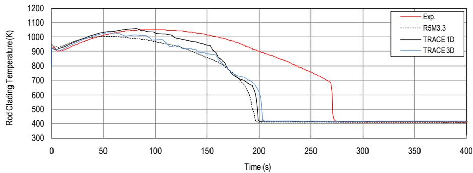
**Figure 14 Peak cladding temperature at 2.13 m elevation**
