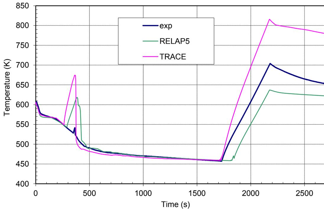
**Figure 40 Heater rod surface temperature at the top of the core – BETHSY 6.2TC**
