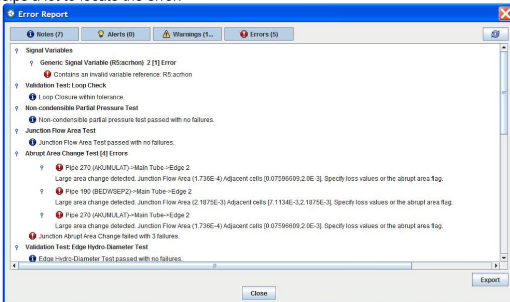
Figure 11 Error report for TRACE model of ACHILLES rig
