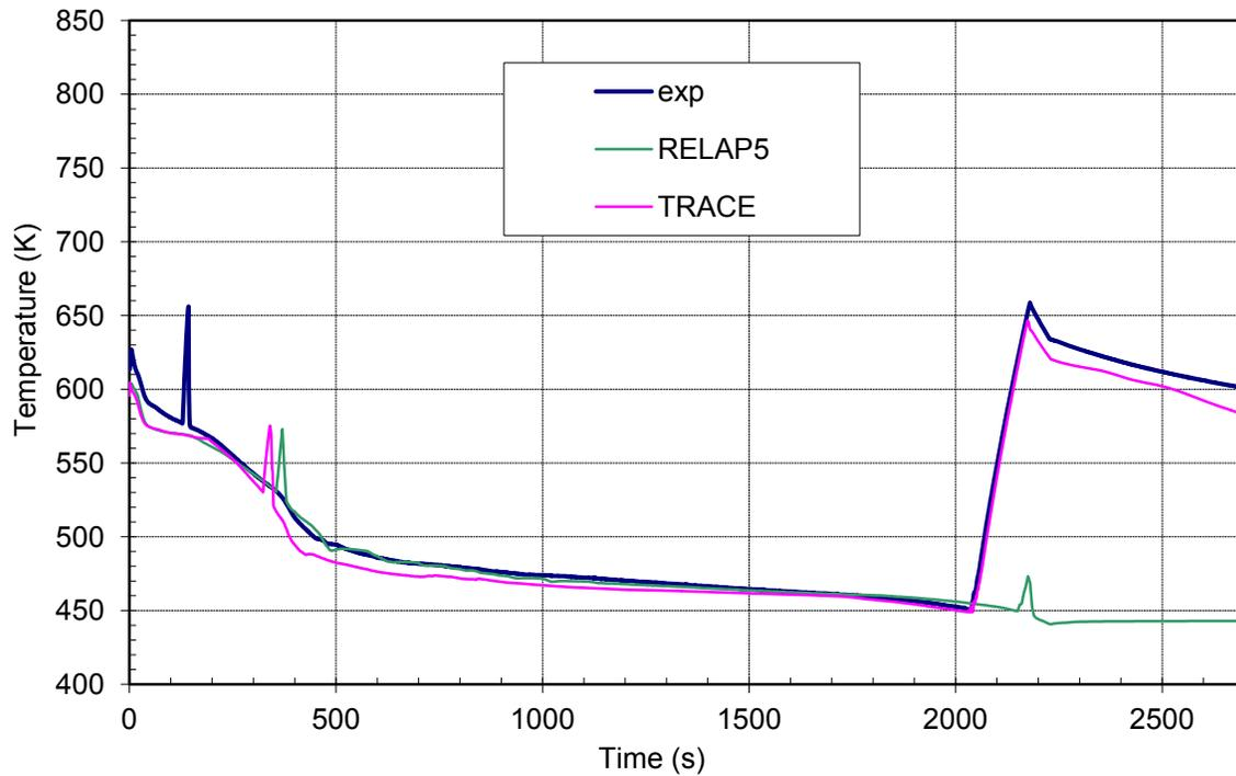
**Figure 39 Heater rod surface temperature at the middle of the core – BETHSY 6.2TC**
