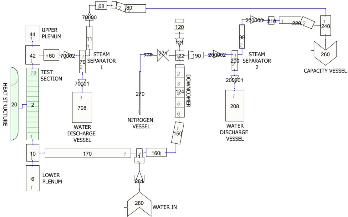
Figure 10 SNAP hydrodynamic components view for TRACE input model of ACHILLES rig
