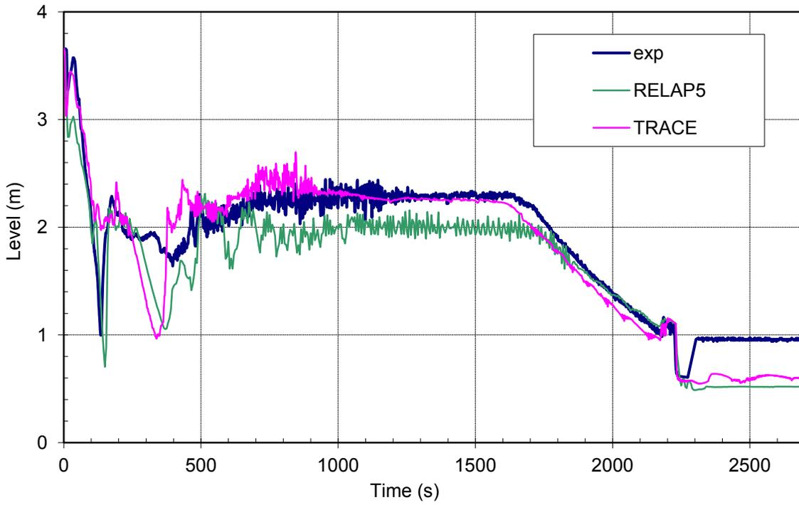
**Figure 41 Core collapsed liquid level – BETHSY 6.2TC**
