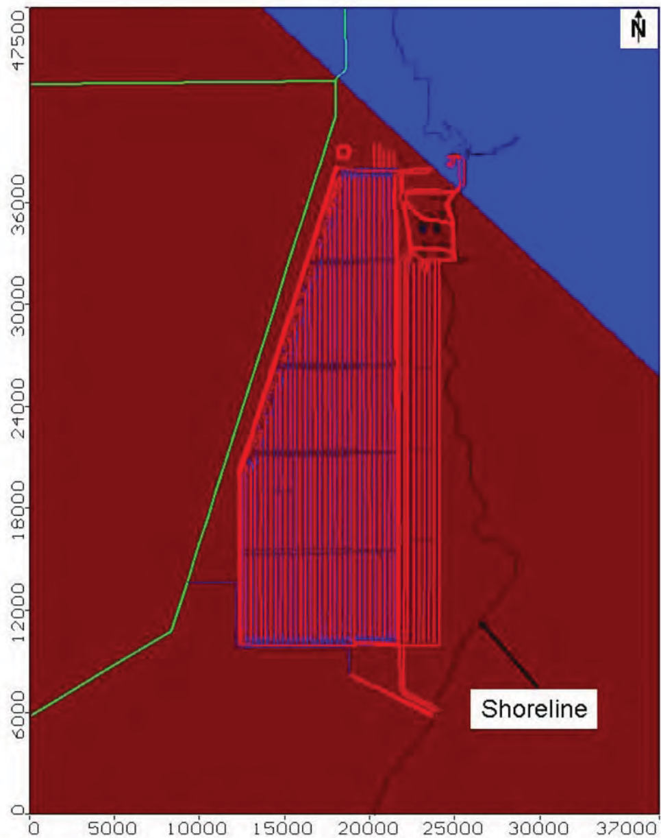
Figure 27. Model Calibration – Delineation of Hydraulic Conductivity Zones in the Key Largo Limestone
