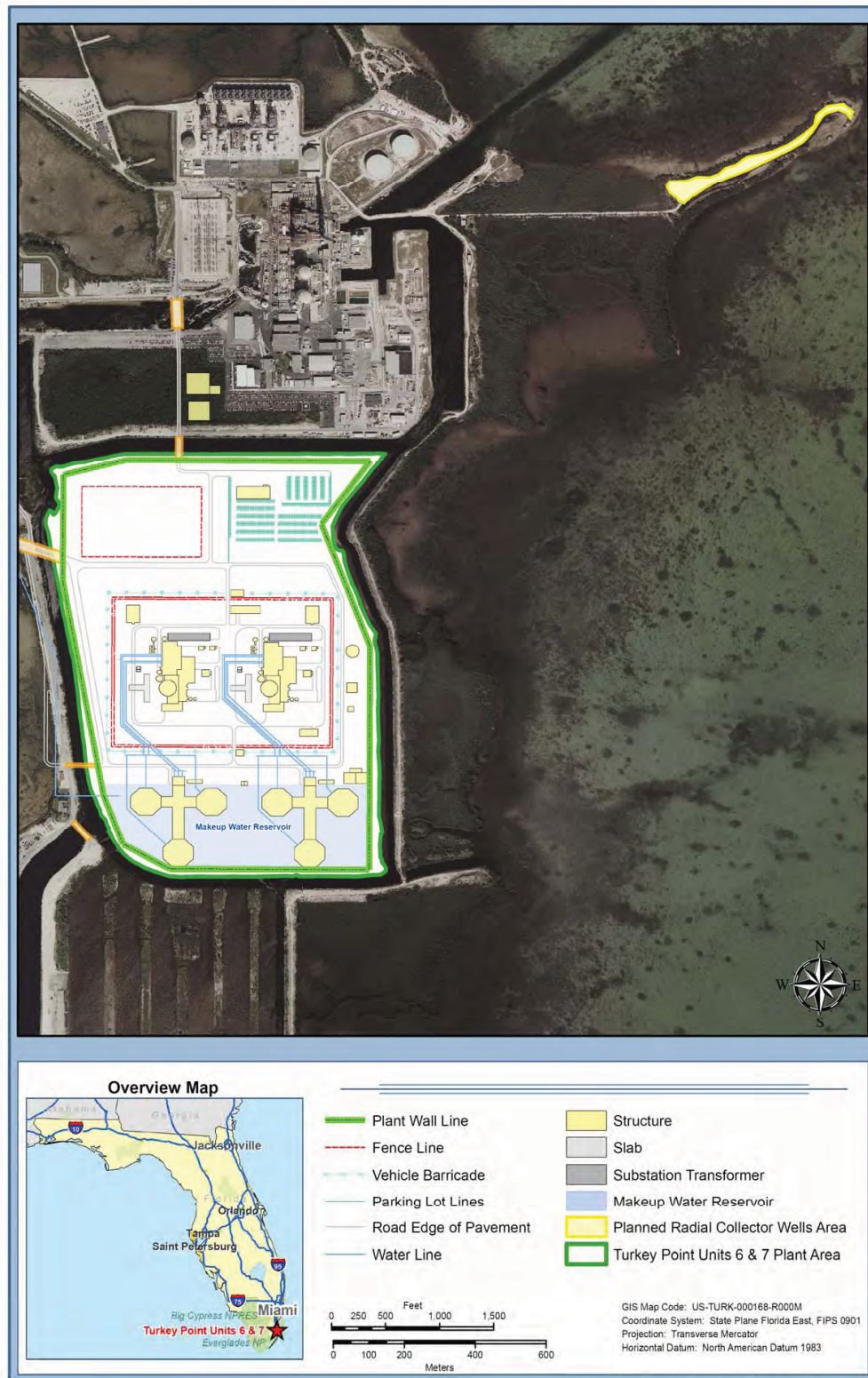
Figure 26. Planned Area of Radial Collector Well Caissons Relative to Plant Site Area
