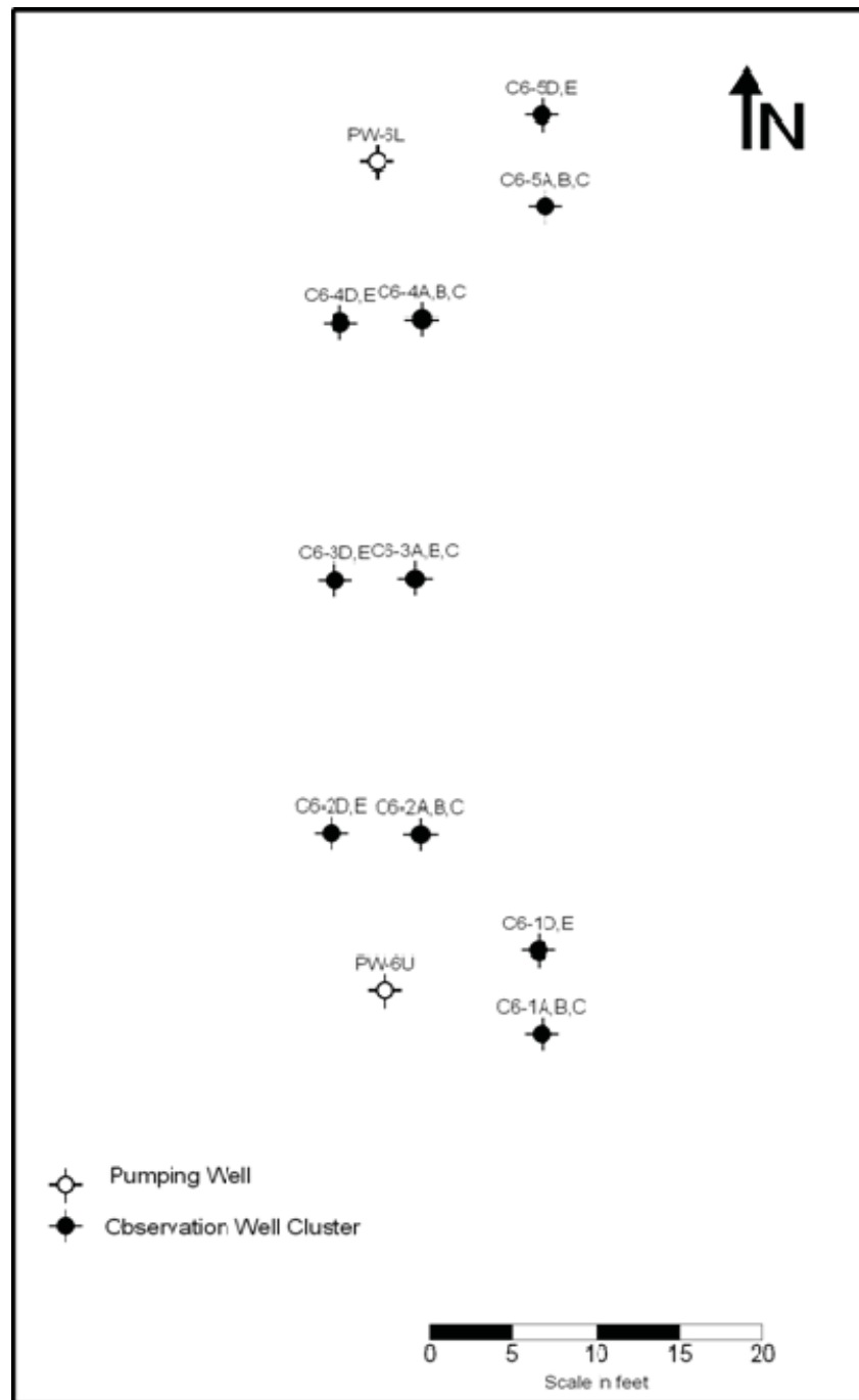
Figure 46. Model Validation – Layout of Pumping and Observation Wells for Pumping Test PW-6U
