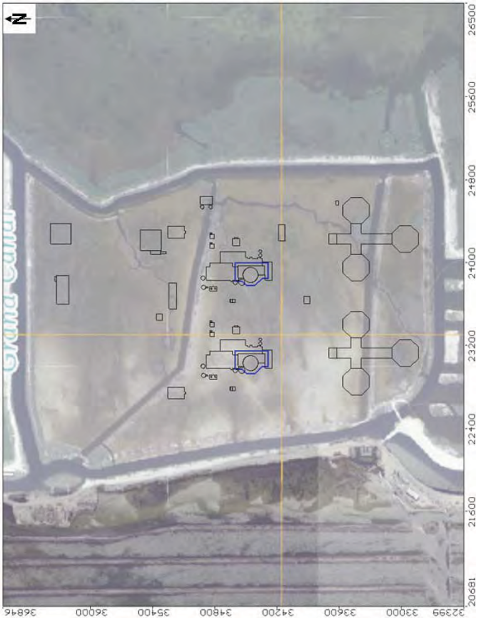
Figure 48. Location of Units 6 & 7 Construction Dewatering Cut-Off Walls
