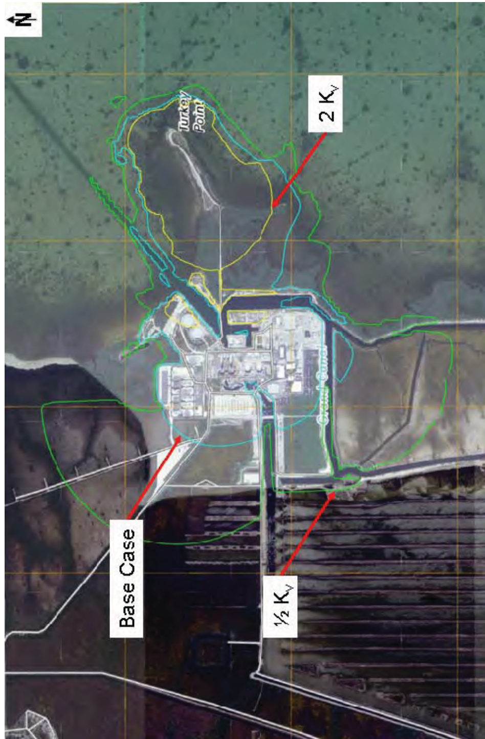
Figure 66. RCW Drawdown within the Top Layer (0.1 Foot Drawdown Contour) – Sensitivity Case Biscayne Bay Vertical Hydraulic Conductivity
