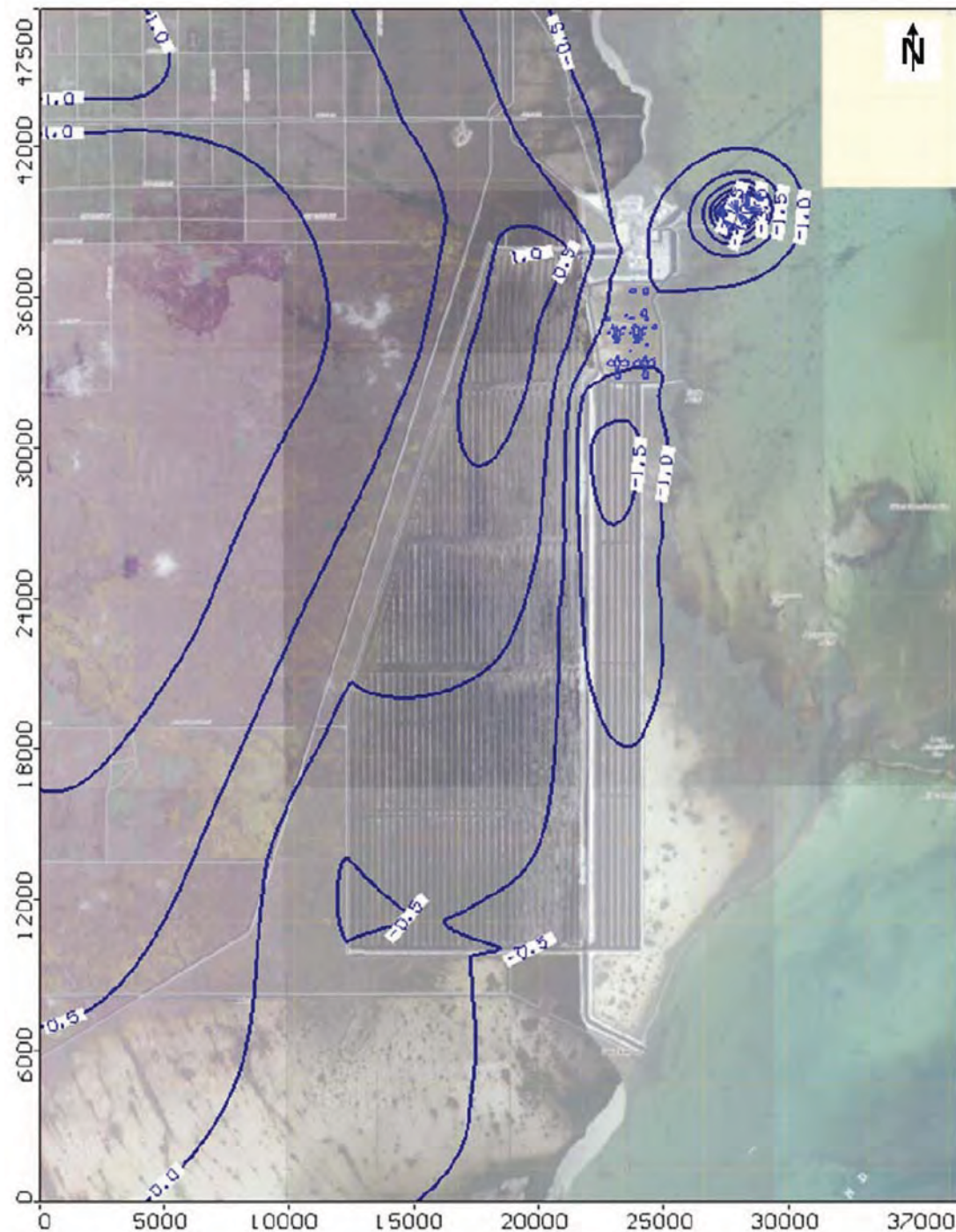
Figure 56. Potentiometric Surface within the Upper Higher Flow Zone during Radial Collector Well Simulations
