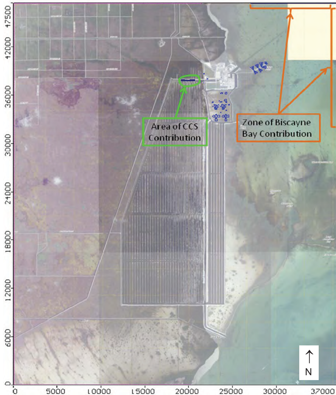
Figure 62. Origin of Flow to the RCW System (Layer 2)
