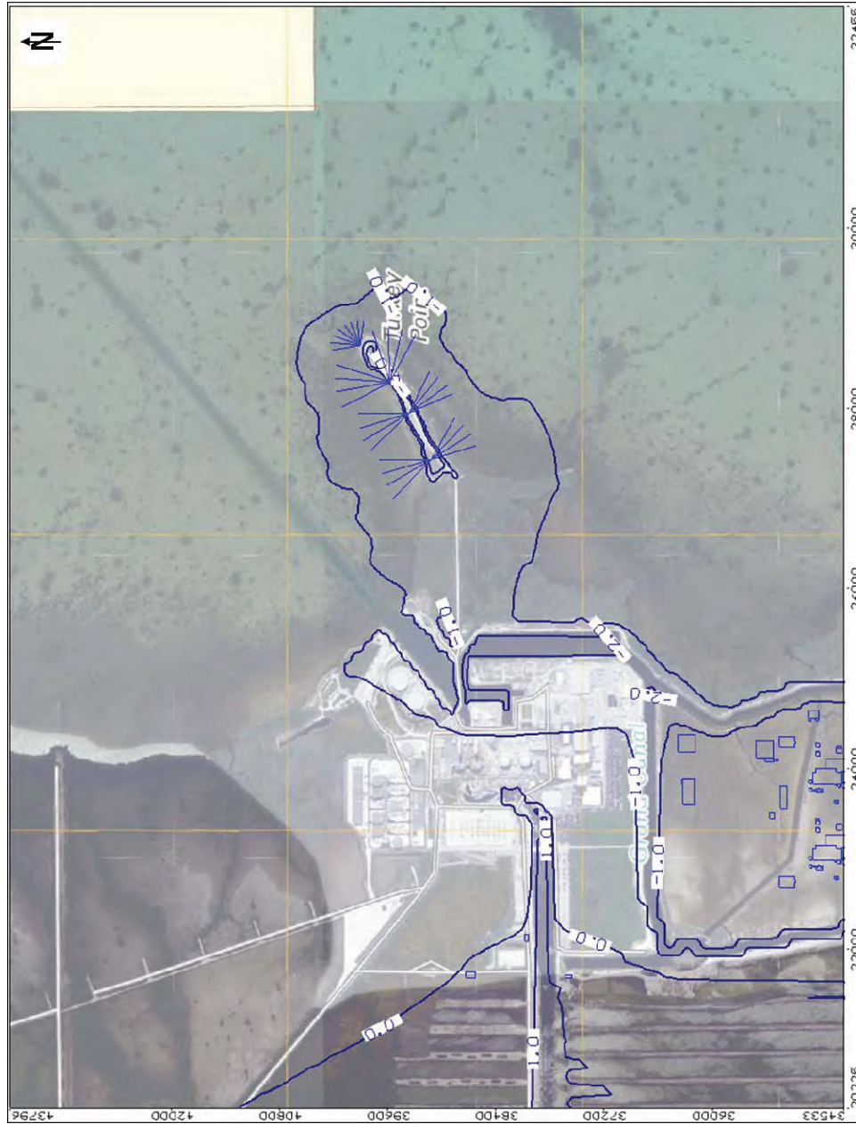
Figure 57. Head Contours in Layer 1 during Radial Collector Well Simulations
