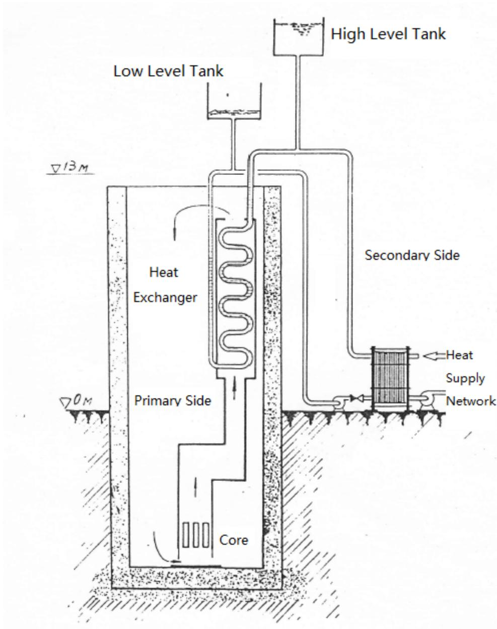
Fig. 1 The Schematic Diagram of Natural Circulation Reactor
