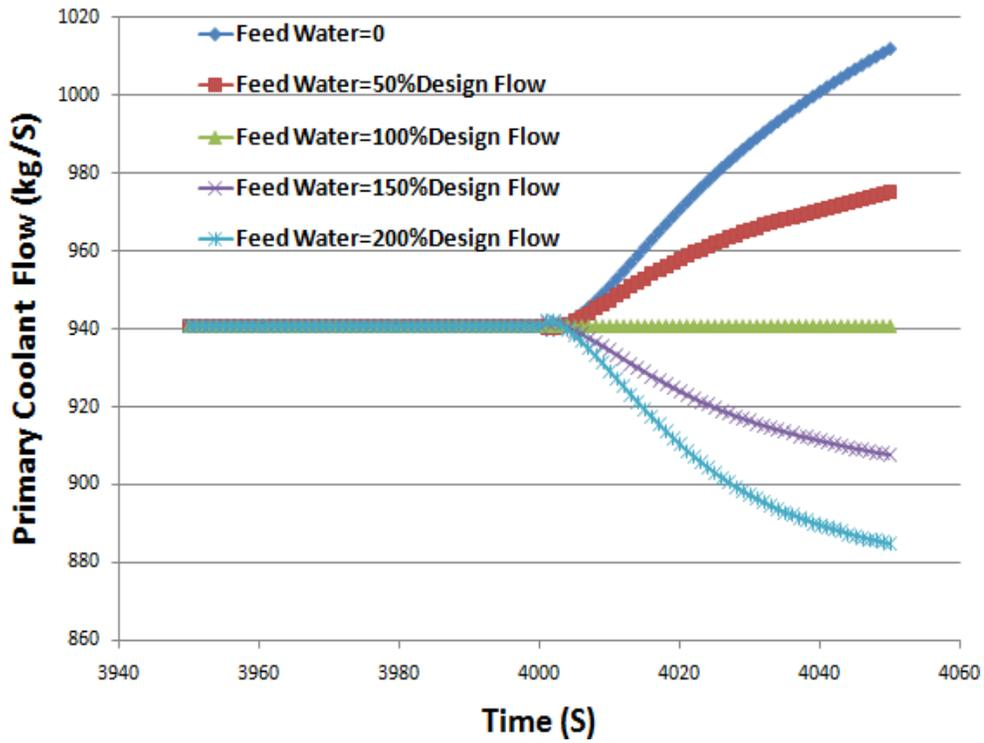
Fig. 19 Feed Water Sensitivity to Natural Circulation Flow
