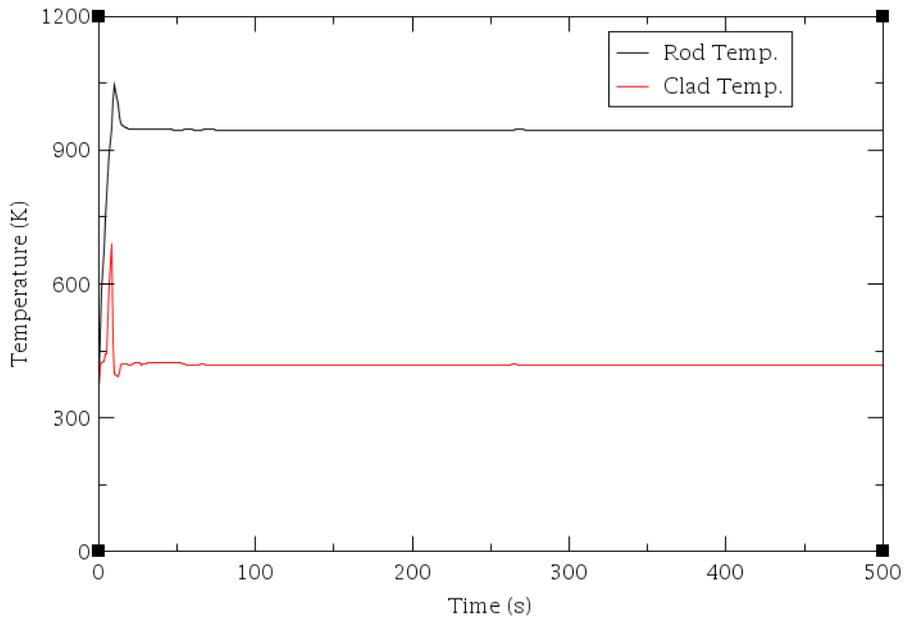
Fig. 12 Rod and Clad Temperature (SS)
