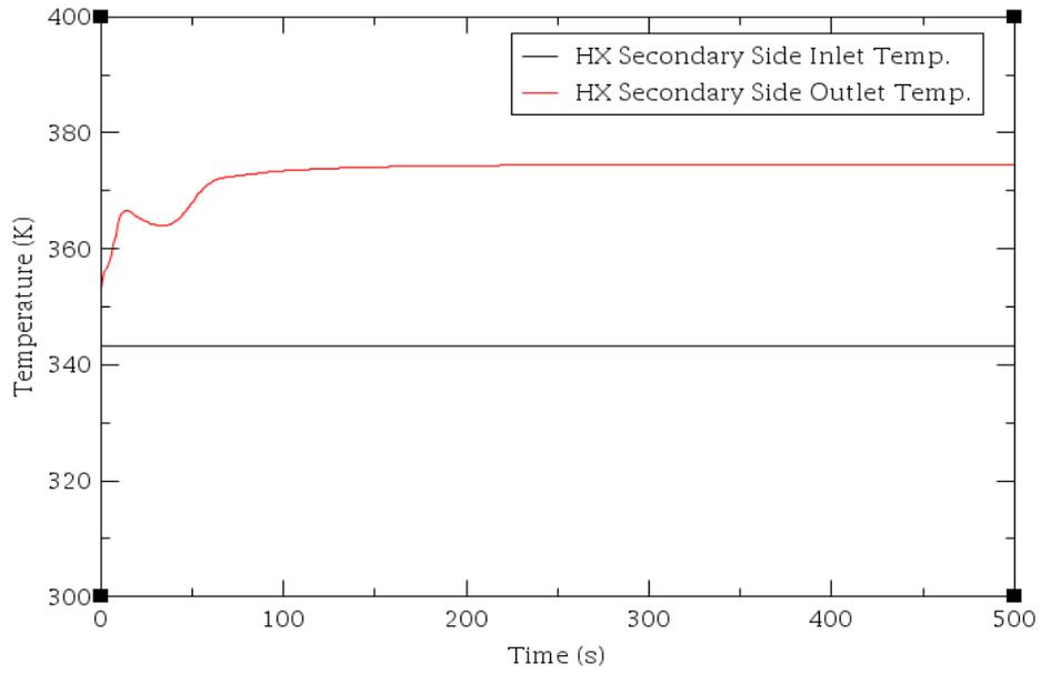
Fig. 14 HX Secondary Side Inlet and Outlet temperature (SS)
