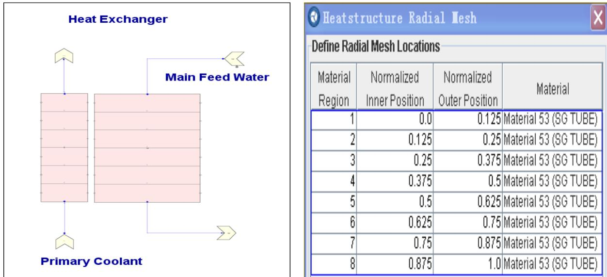
Fig. 5 The TRACE Model of the Heat Exchanger Component for NCR
