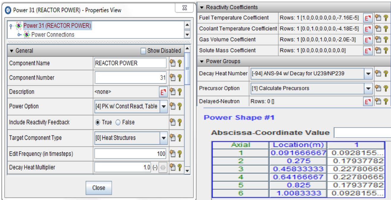
Fig. 4 The TRACE Model of the Power Component for NCR
