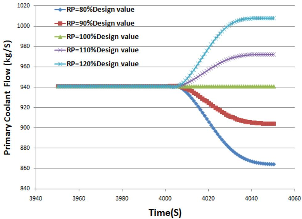
Fig. 20 Reactor Power Sensitivity to Natural Circulation Flow
