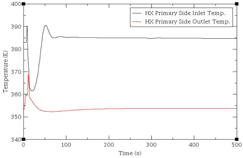
Fig. 13 HX Primary Side Inlet and Outlet Temperature (SS)
