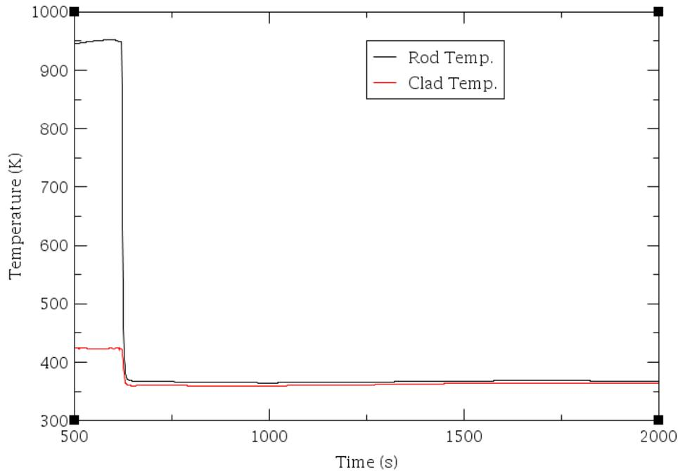
Fig. 18 Rod and Clad temperature (Transient)
