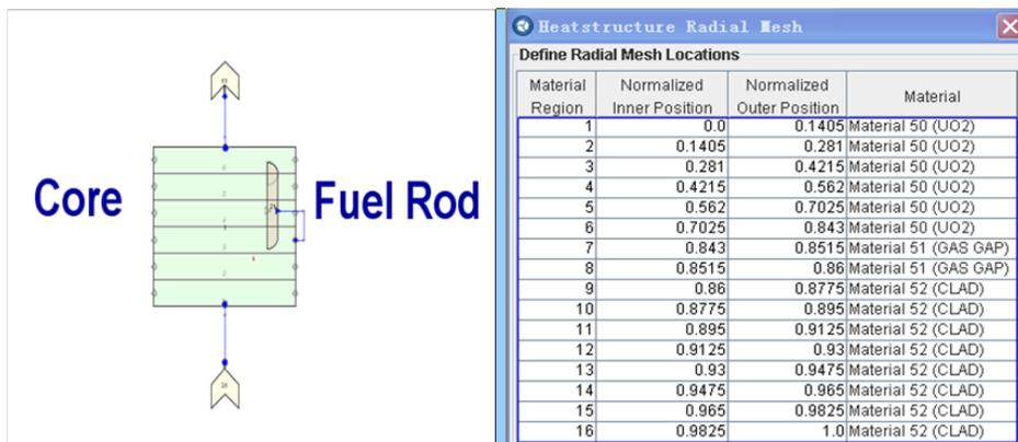
Fig. 3 The TRACE Model of the Core Component for NCR
