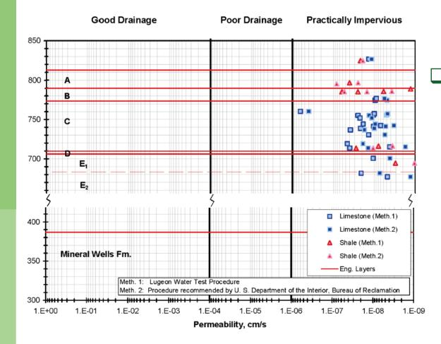
Low hydraulic conductivity values in subsurface materials (Figure from FSAR)
