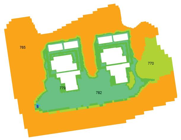
**Color fill contour of bottom of MODFLOW Layer 1**
