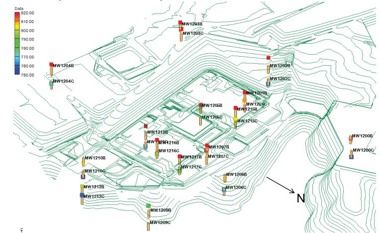
Water levels measured August 2012 in B and C wells – note consistent downward hydraulic gradients
