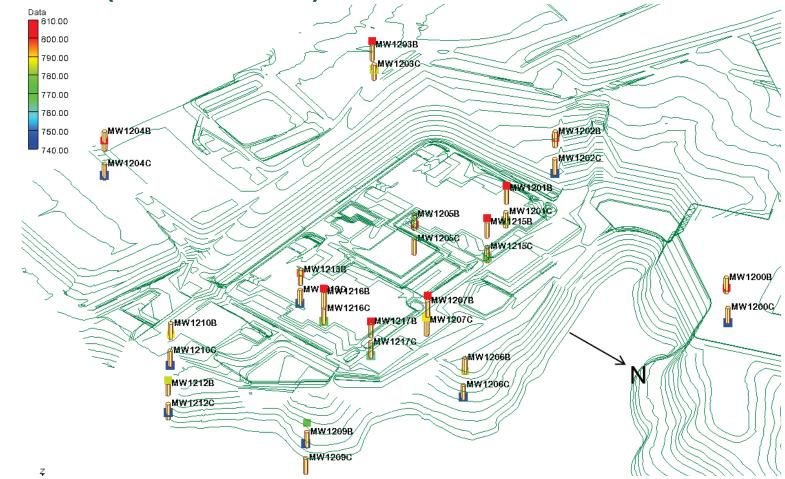
Water levels measured May 2008 in B and C wells – note consistent downward hydraulic gradients
