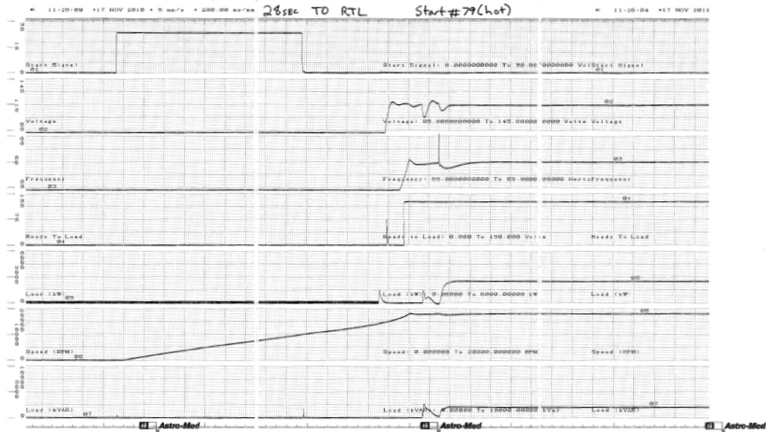
Figure C.1.0-80 Parameter Chart of Start and Load Acceptance Test, No.79, Hot
