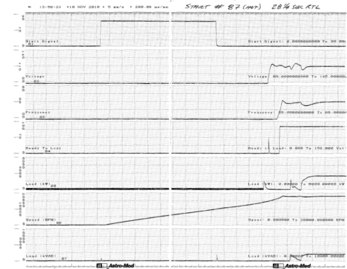
Figure C.1.0-88 Parameter Chart of Start and Load Acceptance Test, No.87, Hot
