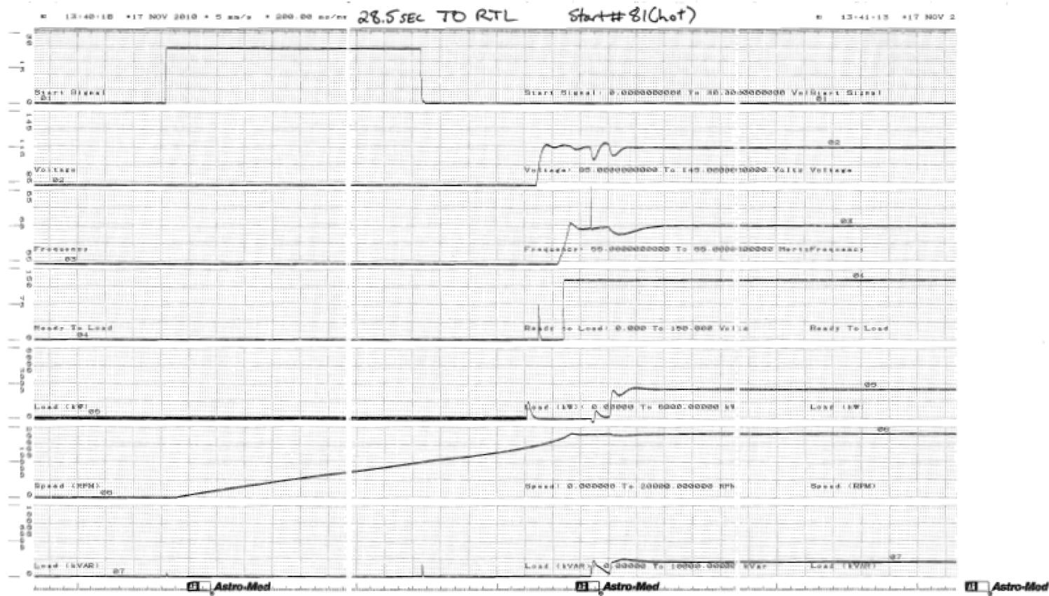
Figure C.1.0-82 Parameter Chart of Start and Load Acceptance Test, No.81, Hot
