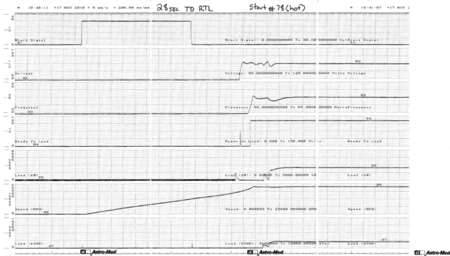
Figure C.1.0-79 Parameter Chart of Start and Load Acceptance Test, No.78, Hot
