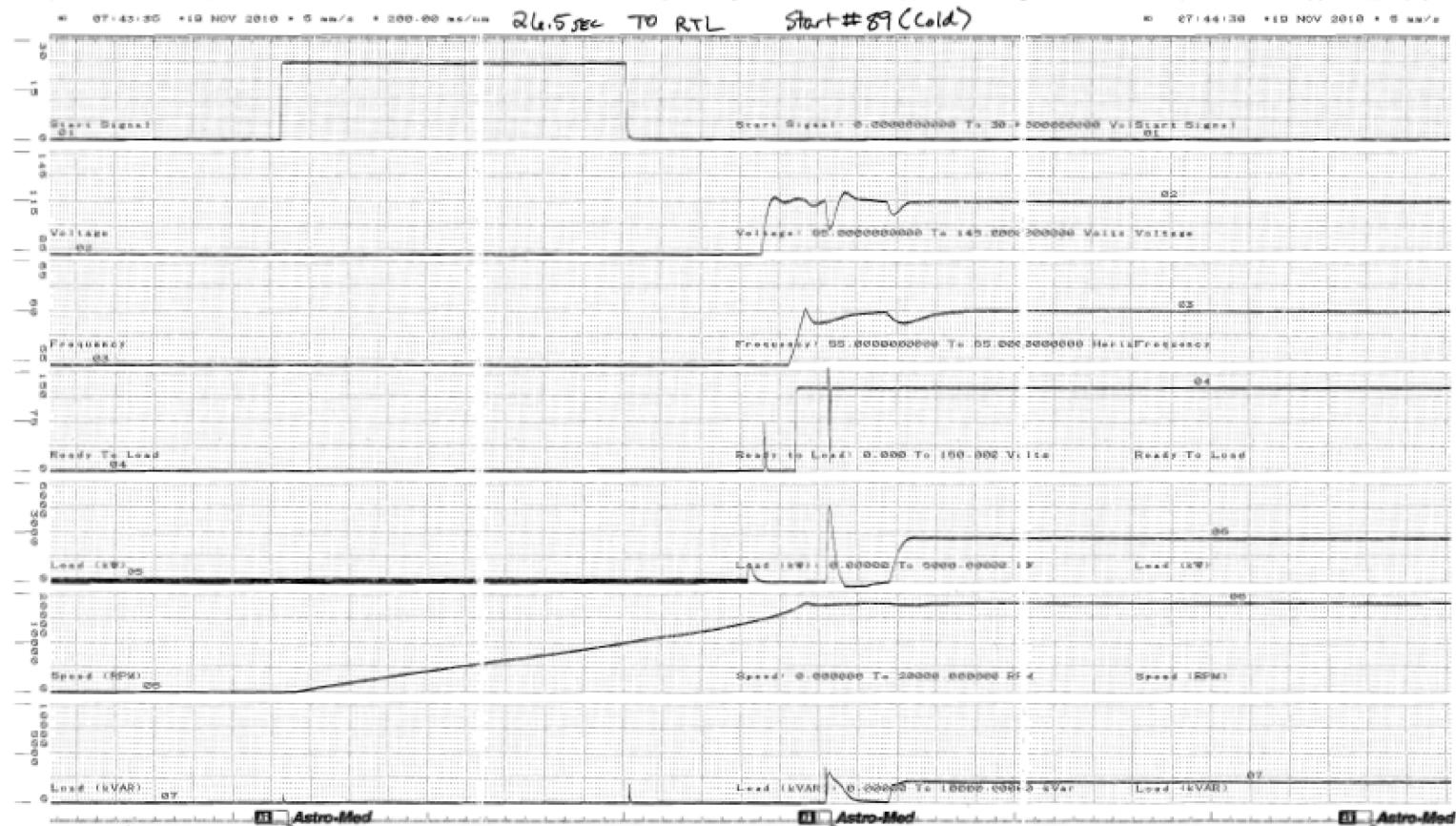
Figure C.1.0-90 Parameter Chart of Start and Load Acceptance Test, No.89, Cold
