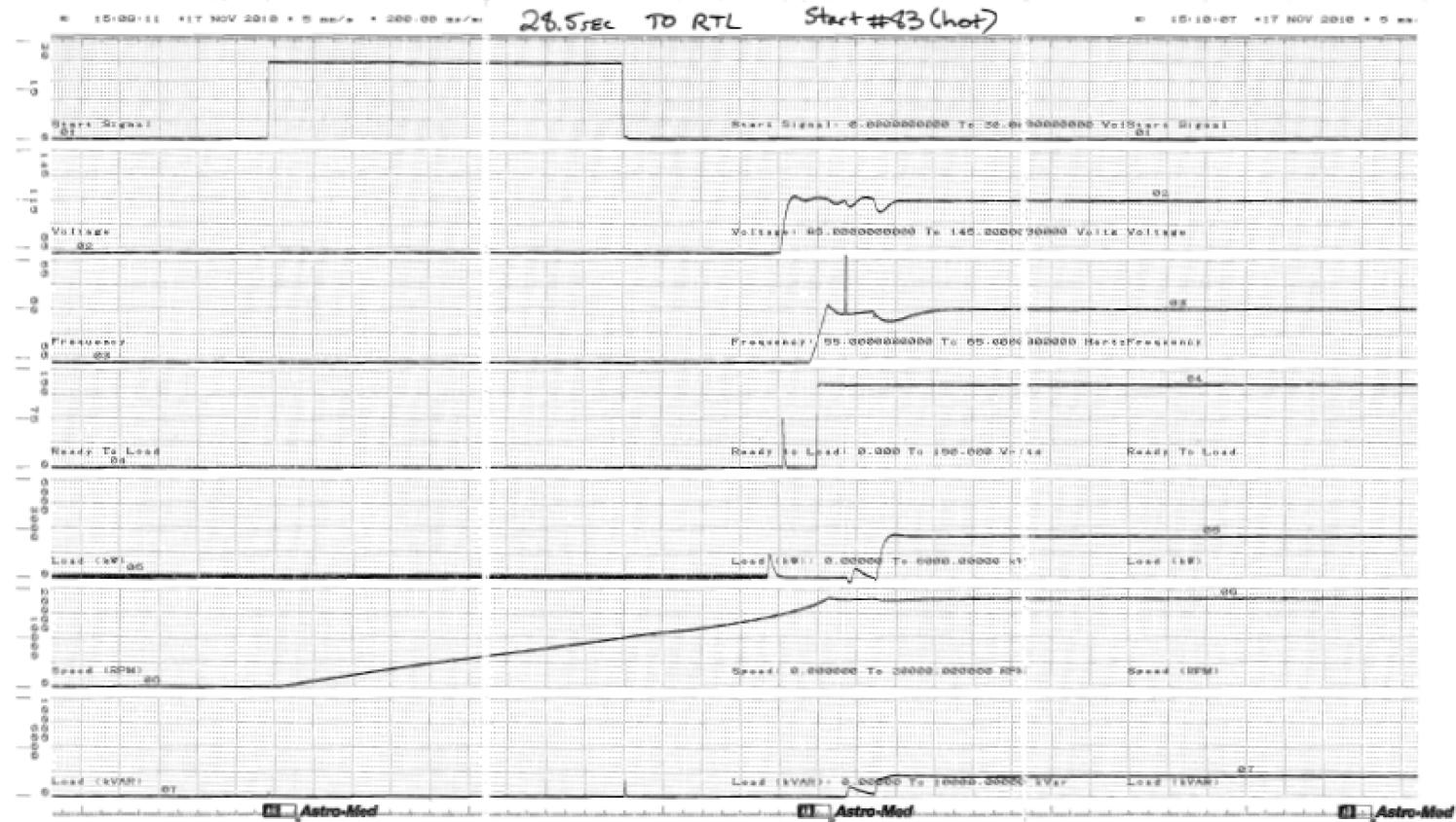
Figure C.1.0-84 Parameter Chart of Start and Load Acceptance Test, No.83, Hot
