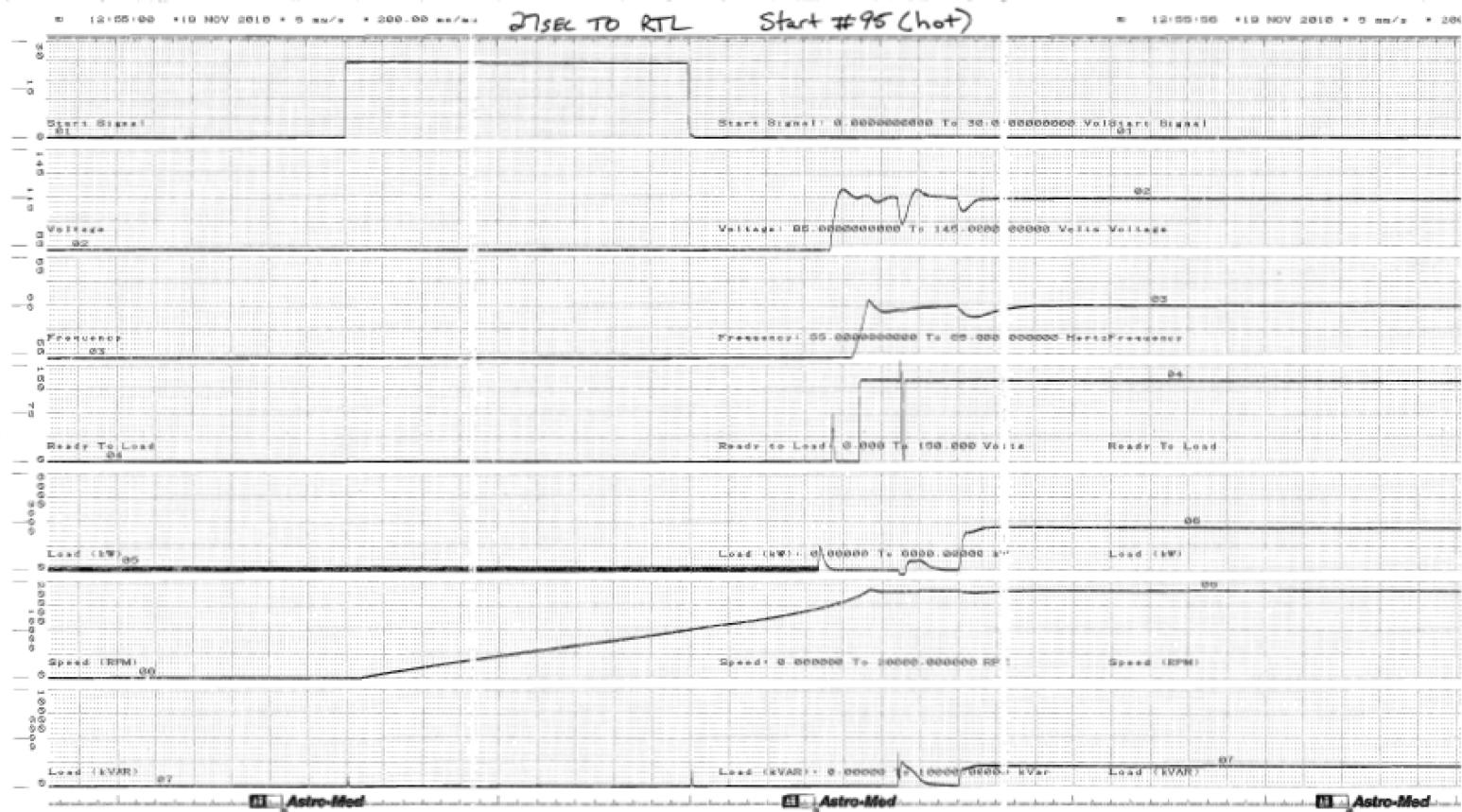
Figure C.1.0-96 Parameter Chart of Start and Load Acceptance Test, No.95, Hot
