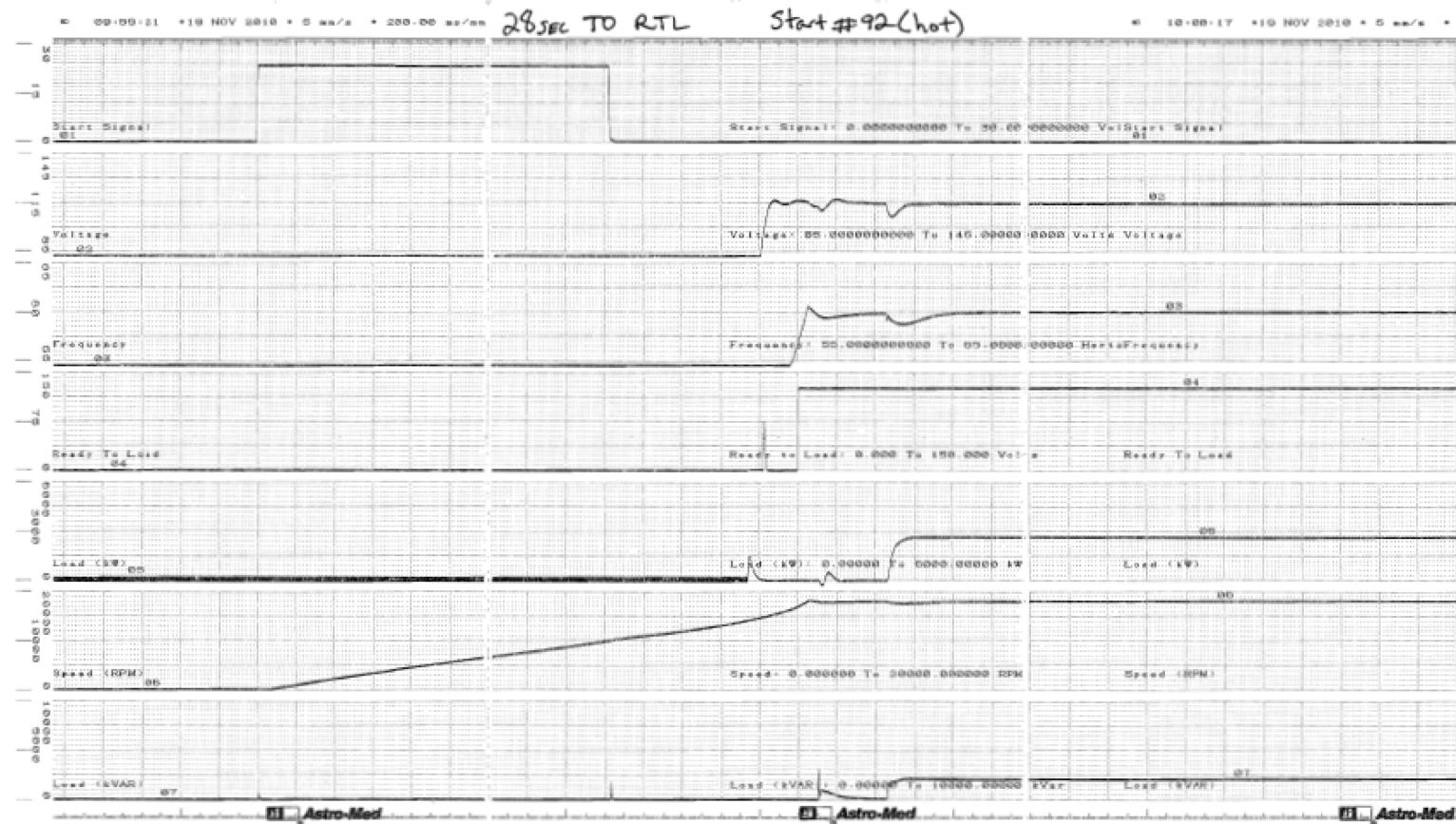
Figure C.1.0-93 Parameter Chart of Start and Load Acceptance Test, No.92, Hot
