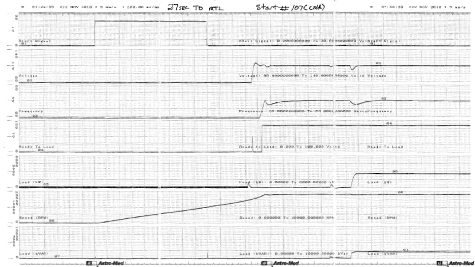
Figure C.1.0-108 Parameter Chart of Start and Load Acceptance Test, No.107, Cold
