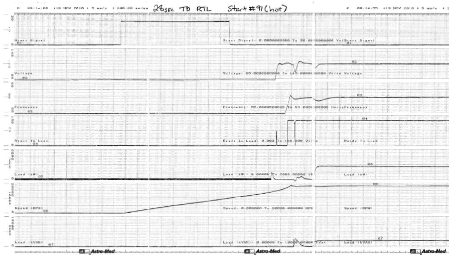
Figure C.1.0-92 Parameter Chart of Start and Load Acceptance Test, No.91, Hot
