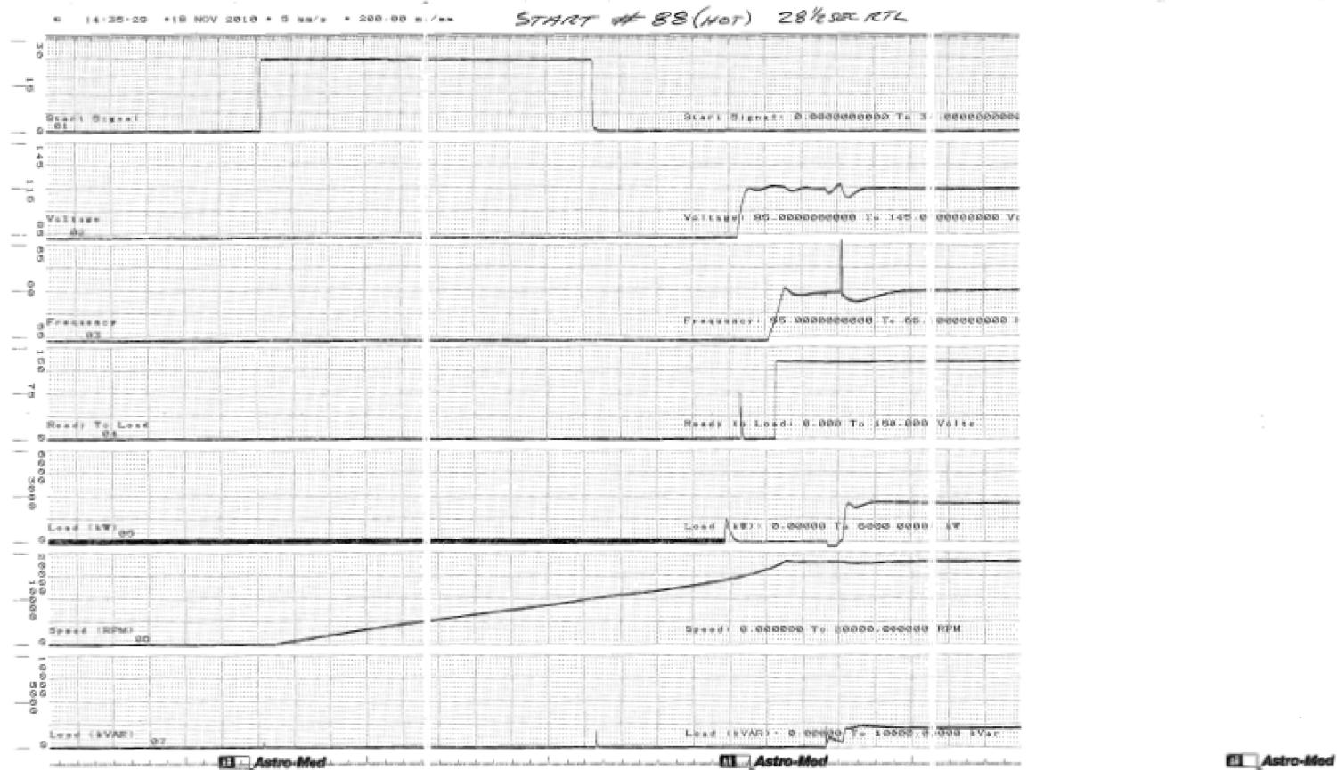
Figure C.1.0-89 Parameter Chart of Start and Load Acceptance Test, No.88, Hot
