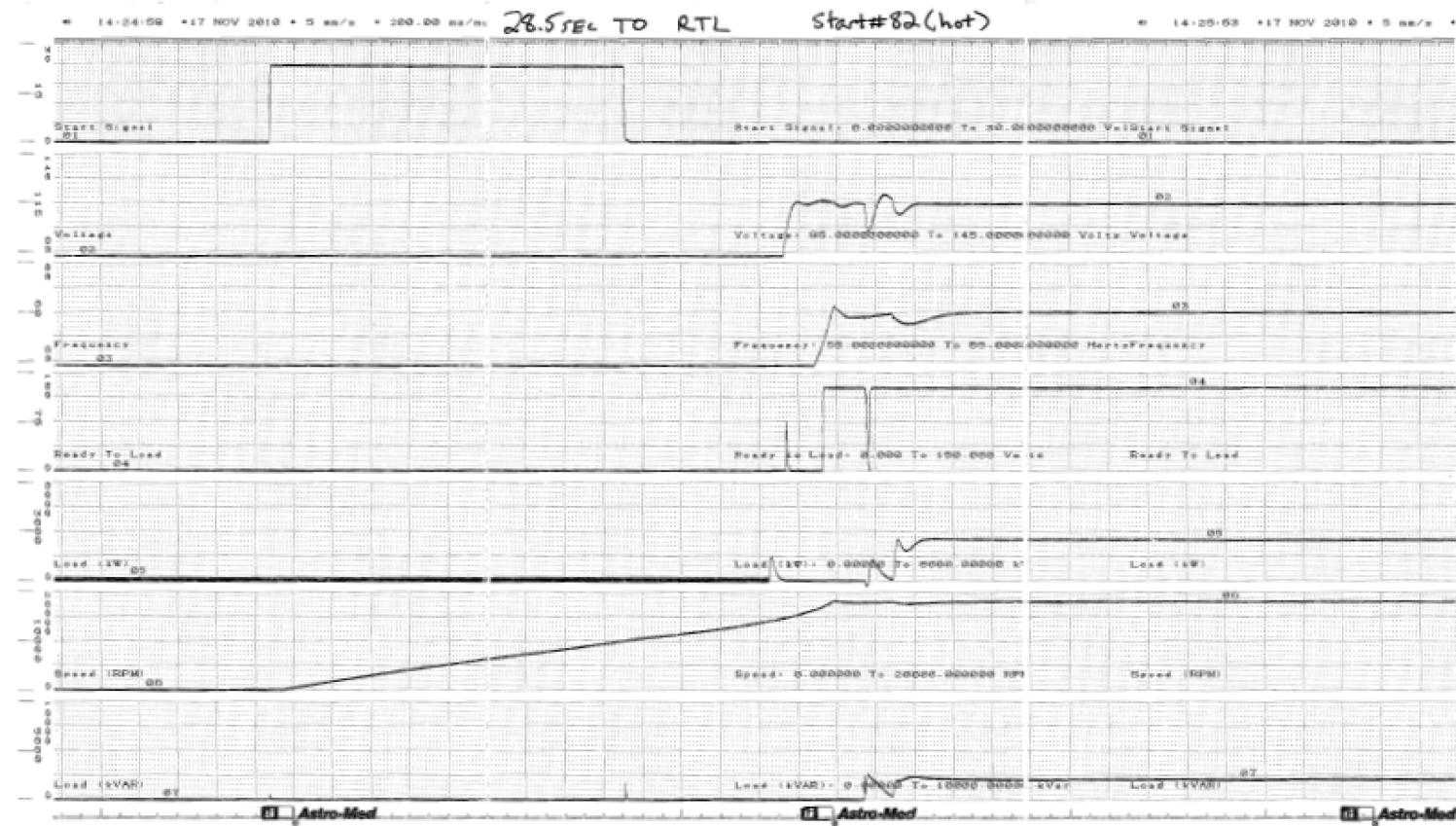
Figure C.1.0-83 Parameter Chart of Start and Load Acceptance Test, No.82, Hot
