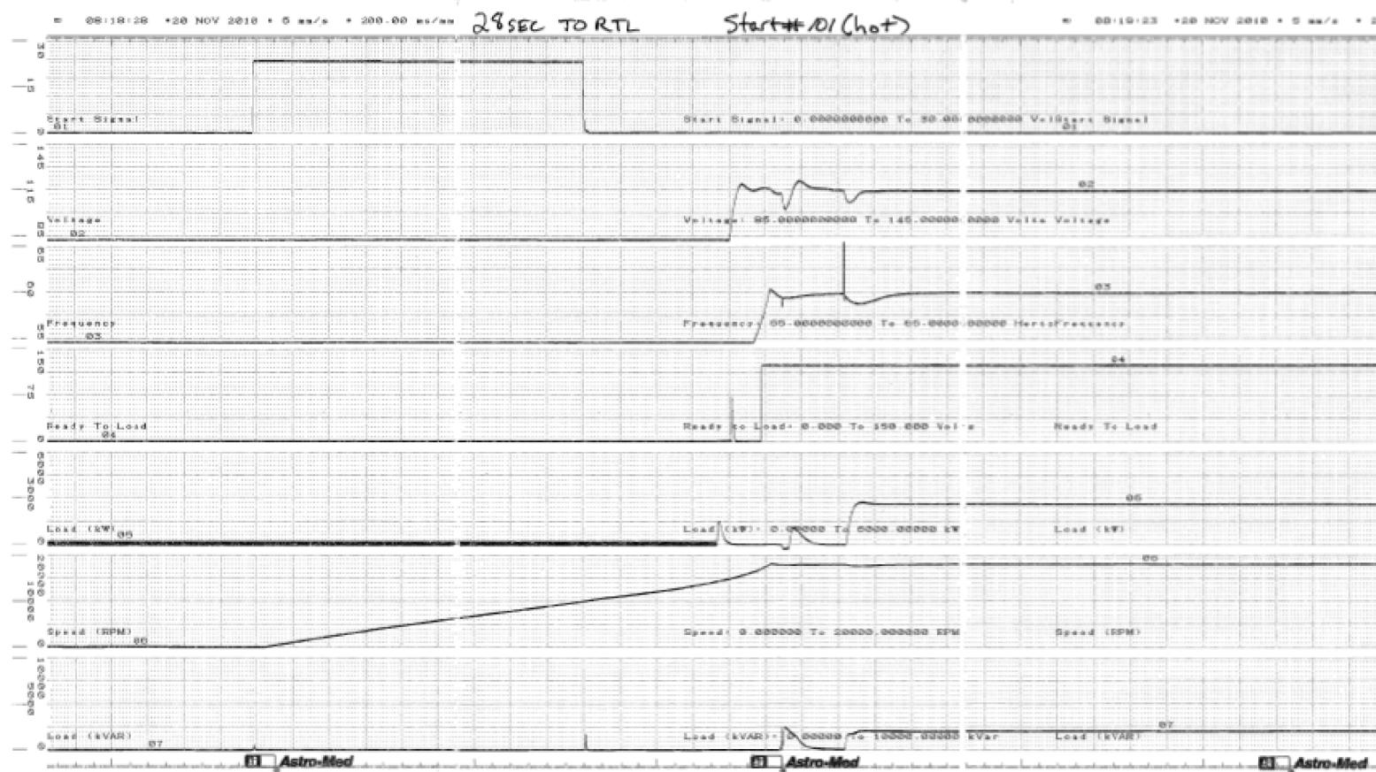
Figure C.1.0-102 Parameter Chart of Start and Load Acceptance Test, No.101, Hot
