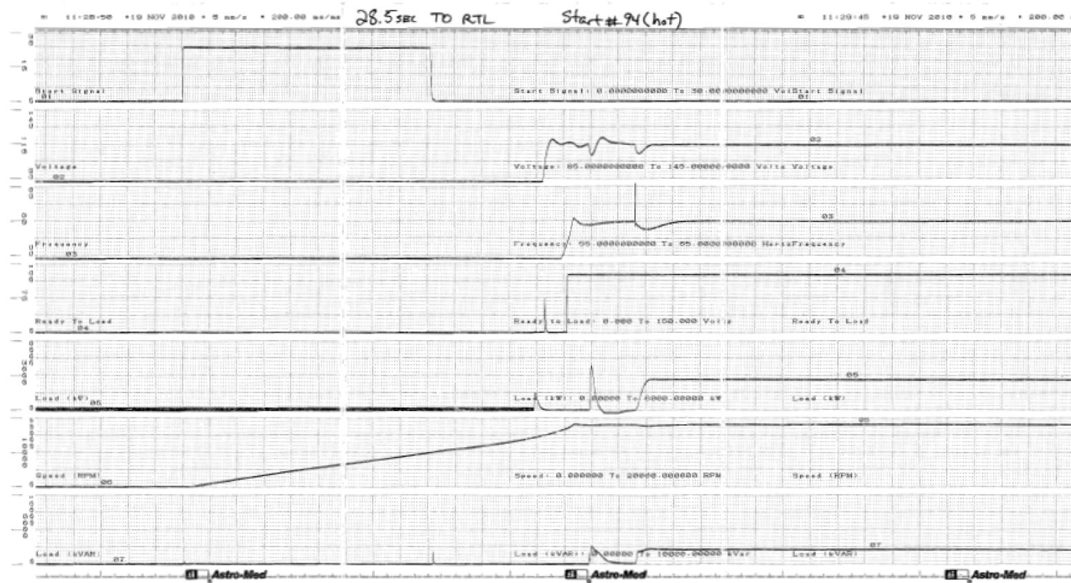
Figure C.1.0-95 Parameter Chart of Start and Load Acceptance Test, No.94, Hot
