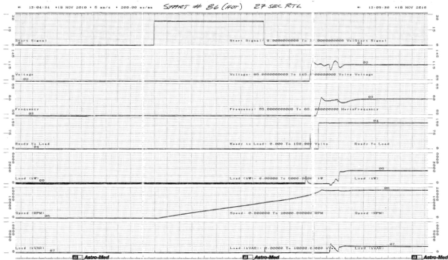
Figure C.1.0-87 Parameter Chart of Start and Load Acceptance Test, No.86, Hot
