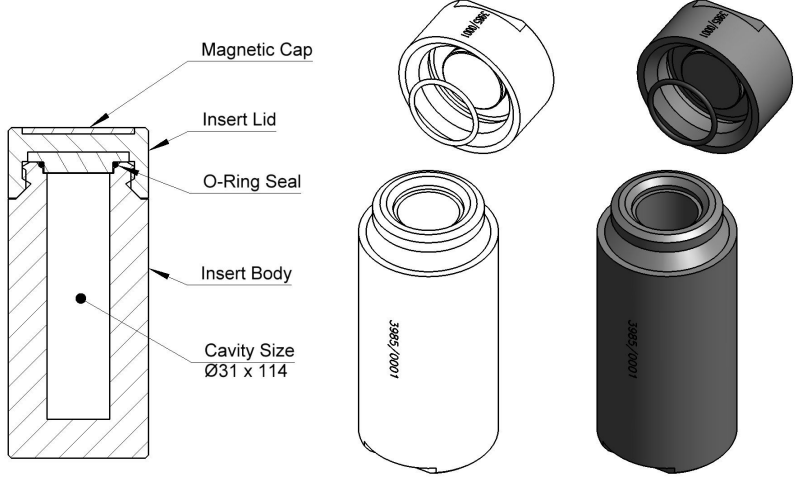
Figure 5: Shielding Insert HS - 31 x 114 -Tu, Design No 3985
