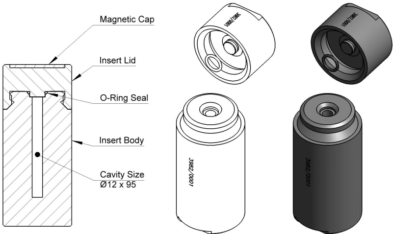
Figure 4: Shielding Insert HS-12 x 95 - Tu, Design No 3982
