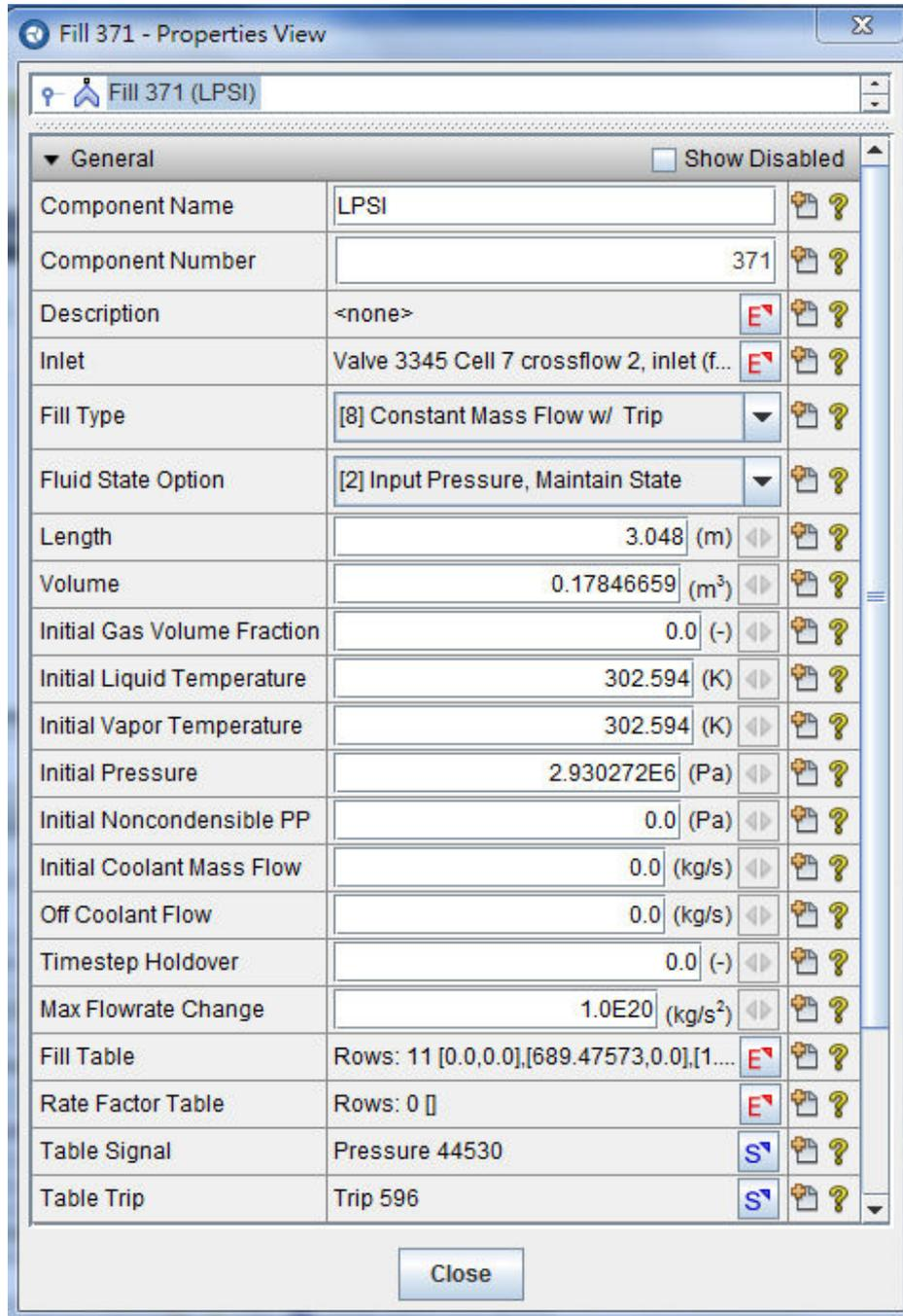
Fig 2.5 The LHSI simulation of TRACE LBLOCA model.
