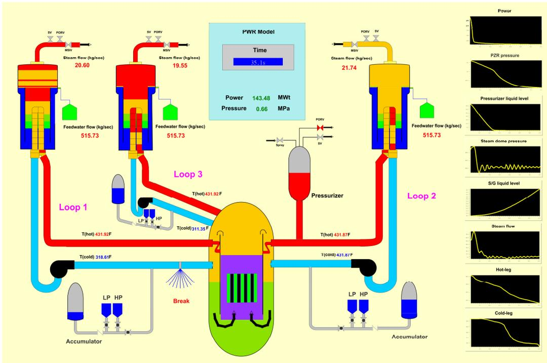
Fig. 4.8 Animation of the TRACE LBLOCA model for Maanshan NPP.
