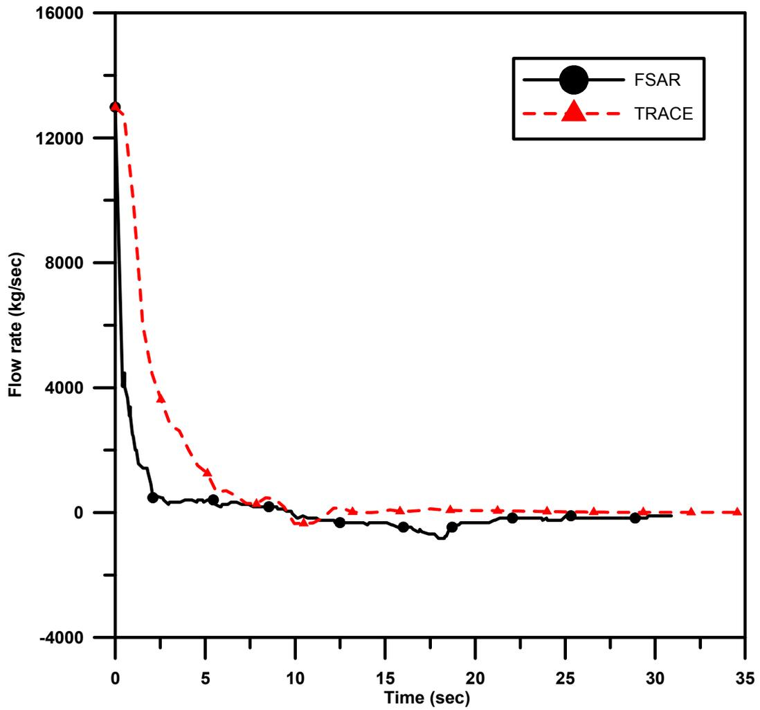
Fig. 4.6 The comparisons of core outlet flow rate between TRACE and FSAR data.
