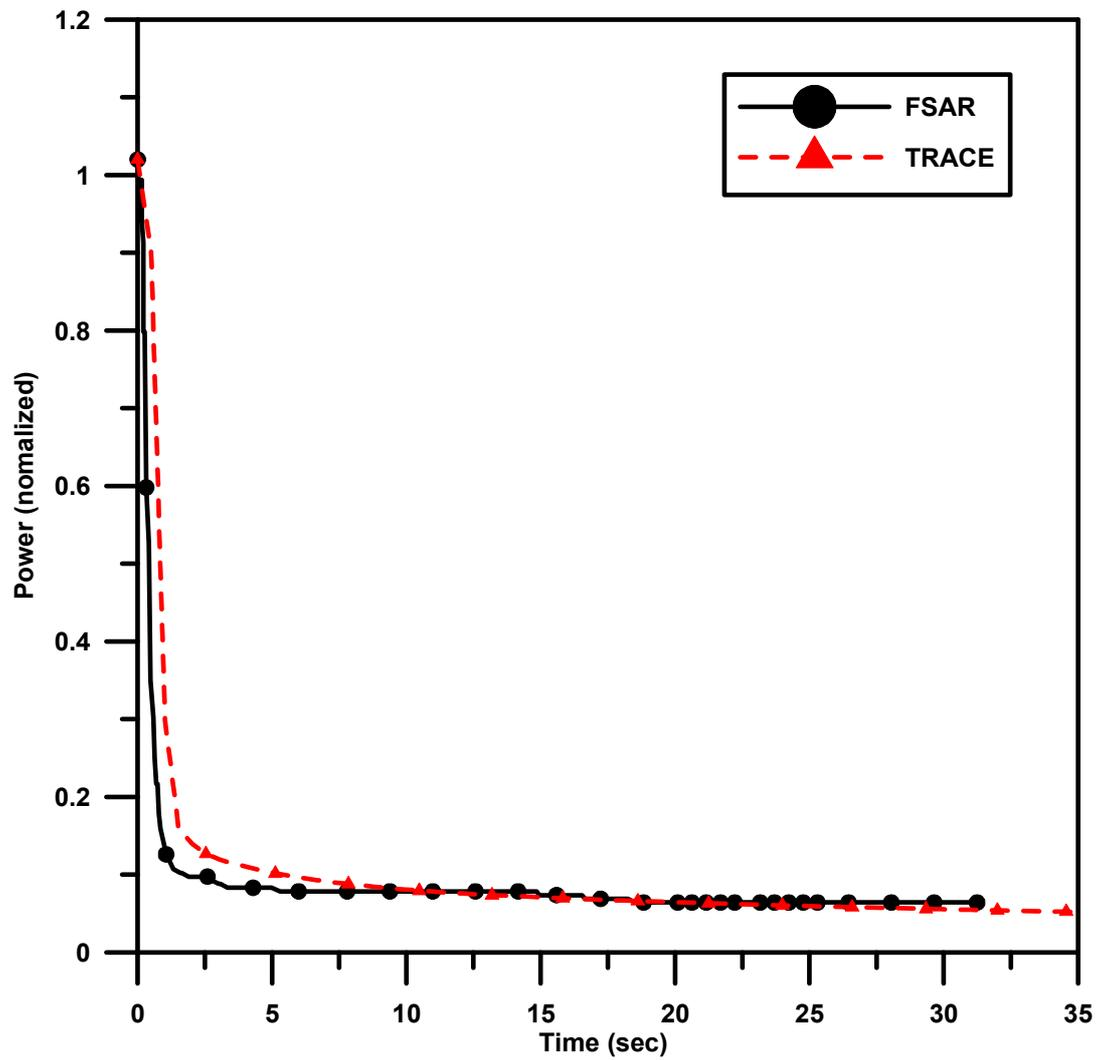
Fig. 4.1 The comparisons of power between TRACE and FSAR data.
