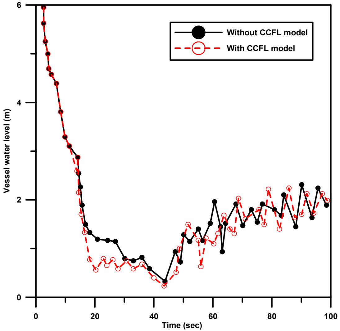
Fig 4.14 The vessel water level results of the CCFL model sensitivity studies.
