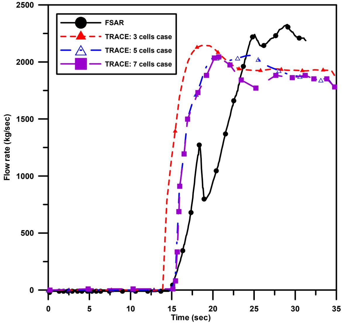
Fig 4.9 The accumulators flow rate results of the accumulators nodalization sensitivity studies.
