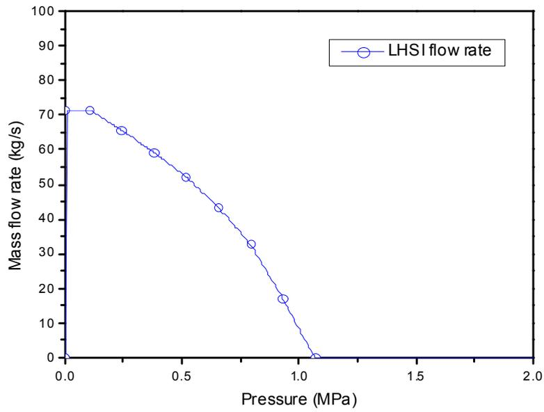
**Fig 2.7 The LHSI flow rate correspond to the RCS pressure.**
