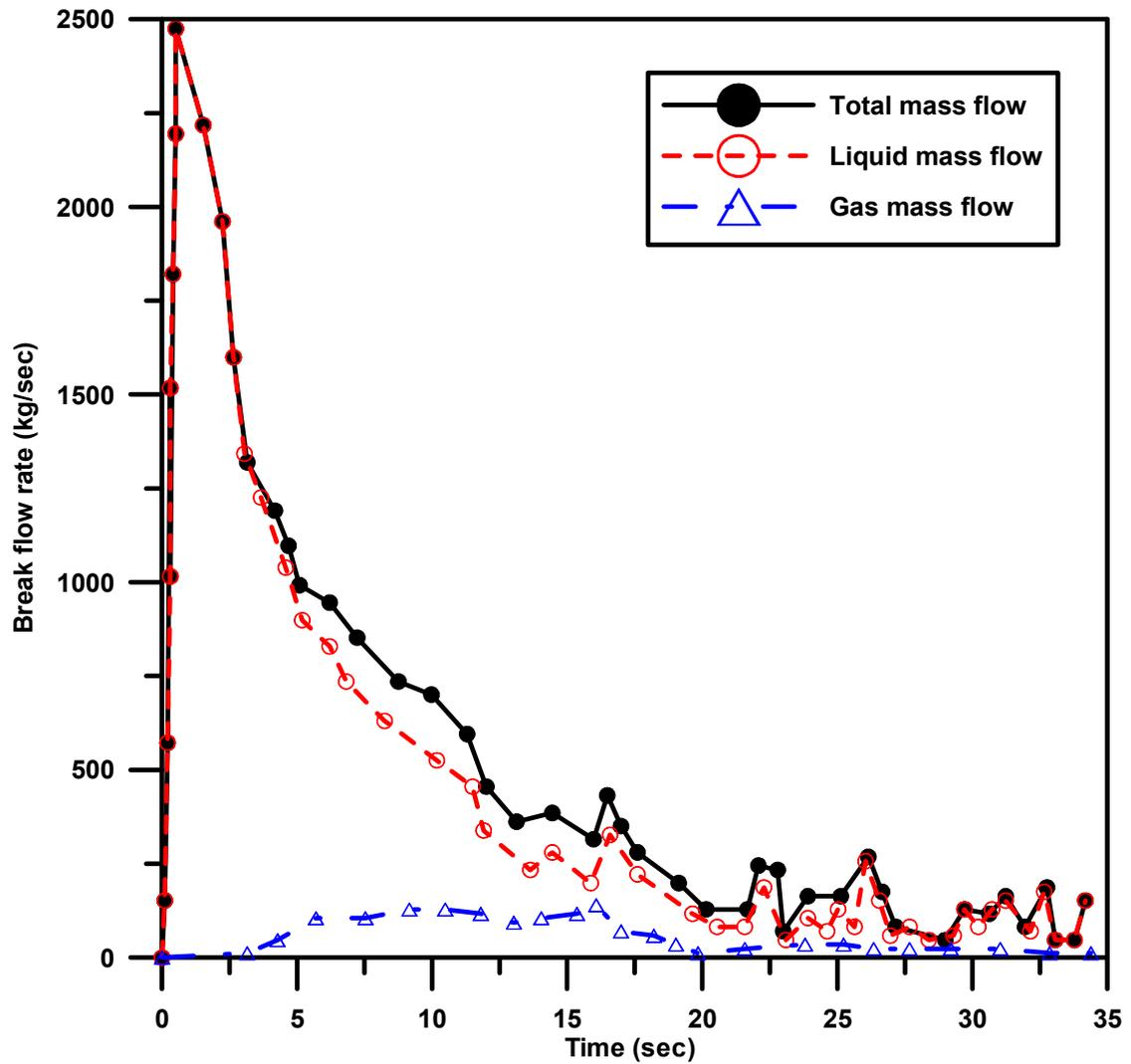
Fig 4.11 The break flow rate result of TRACE.
