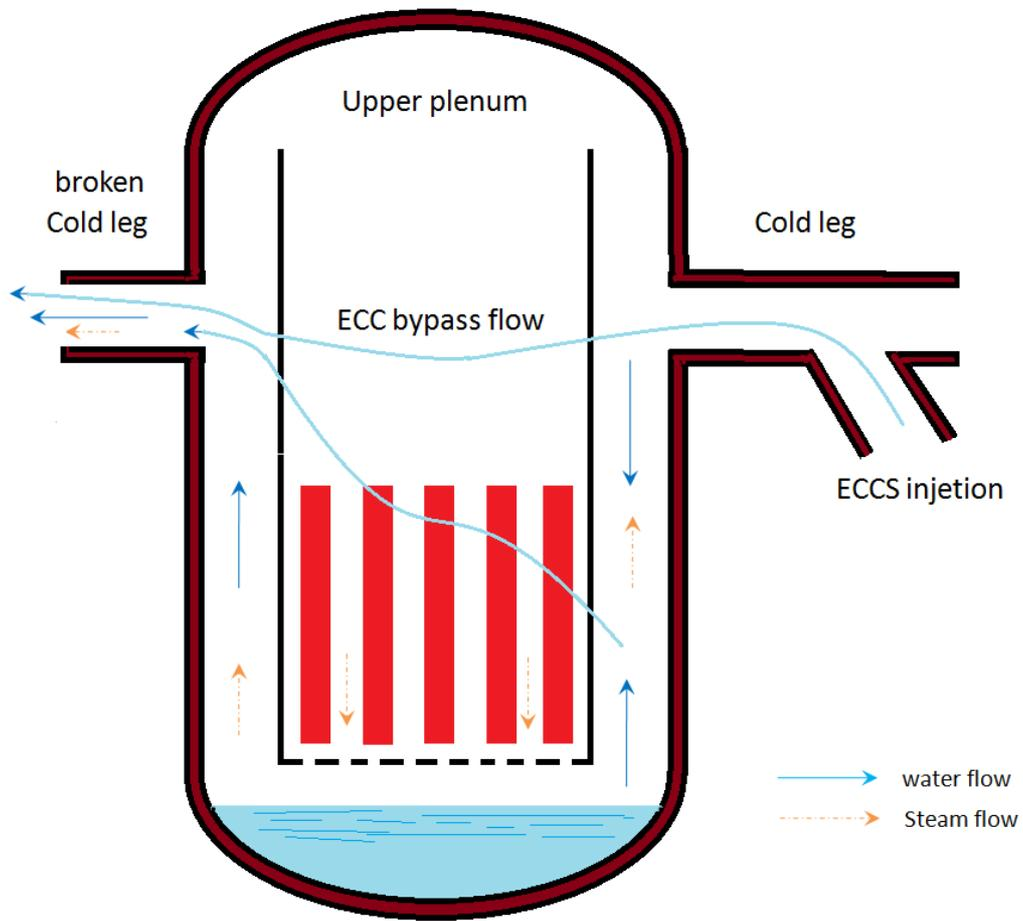
Fig 3.1 The steam and liquid flow phenomena in vessel.
