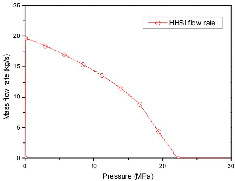
**Fig 2.8 The HHSI flow rate correspond to the RCS pressure.**
