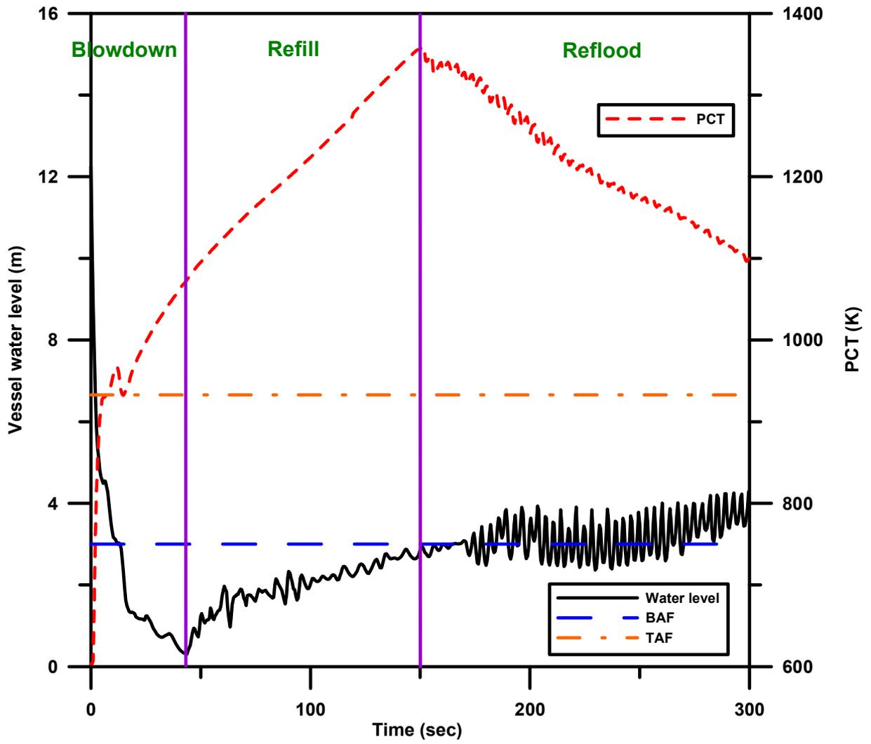
Fig 4.7 The blowdown , refill , and reflood phases of LBLOCA.
