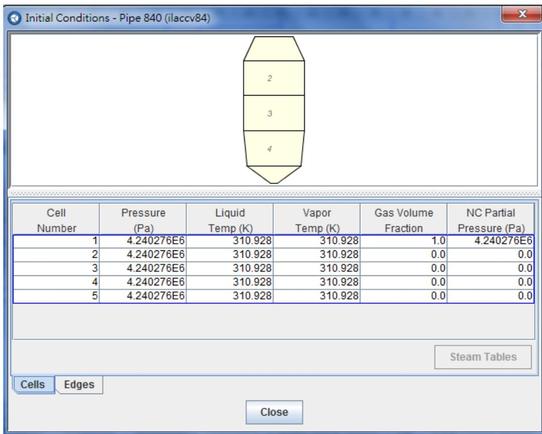
Fig 2.4 The accumulator simulation of TRACE LBLOCA model.
