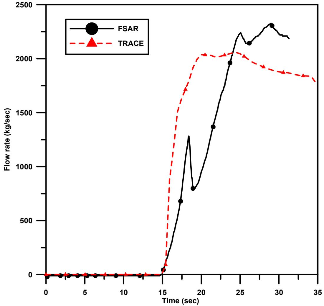
Fig. 4.4 The comparisons of accumulator mass flow rate between TRACE and FSAR data.
