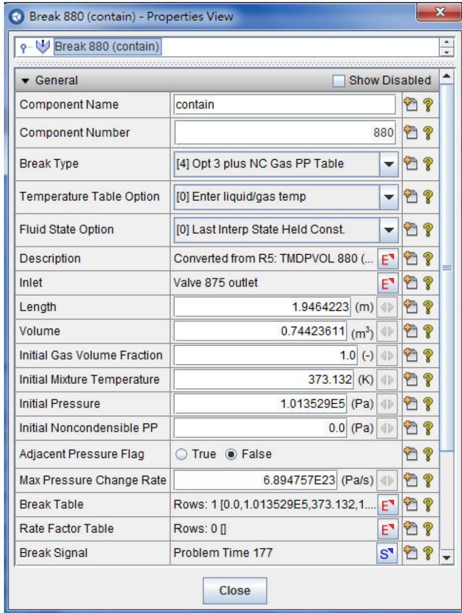
Fig 2.2 The break simulation of TRACE LBLOCA model.
