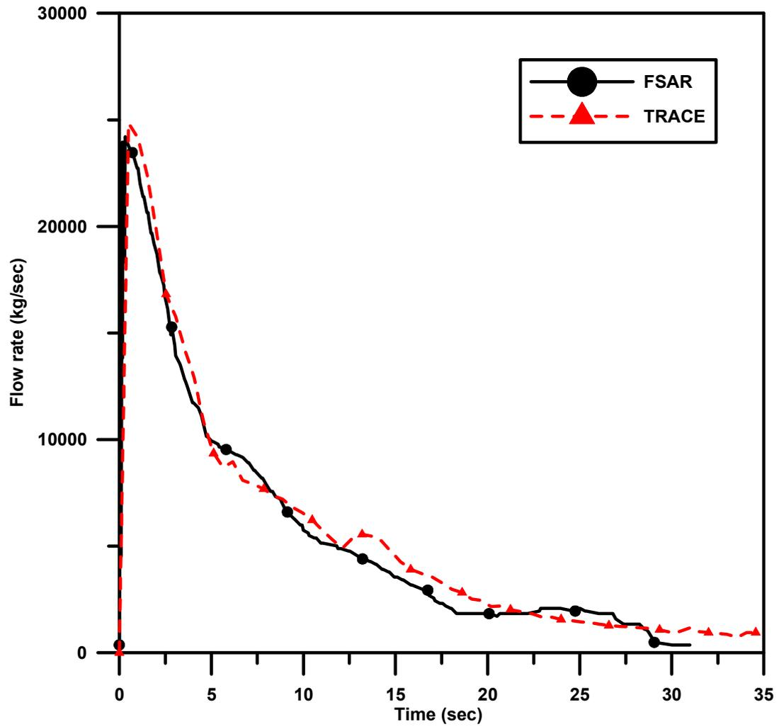
Fig. 4.3 The comparisons of break mass flow rate between TRACE and FSAR data.
