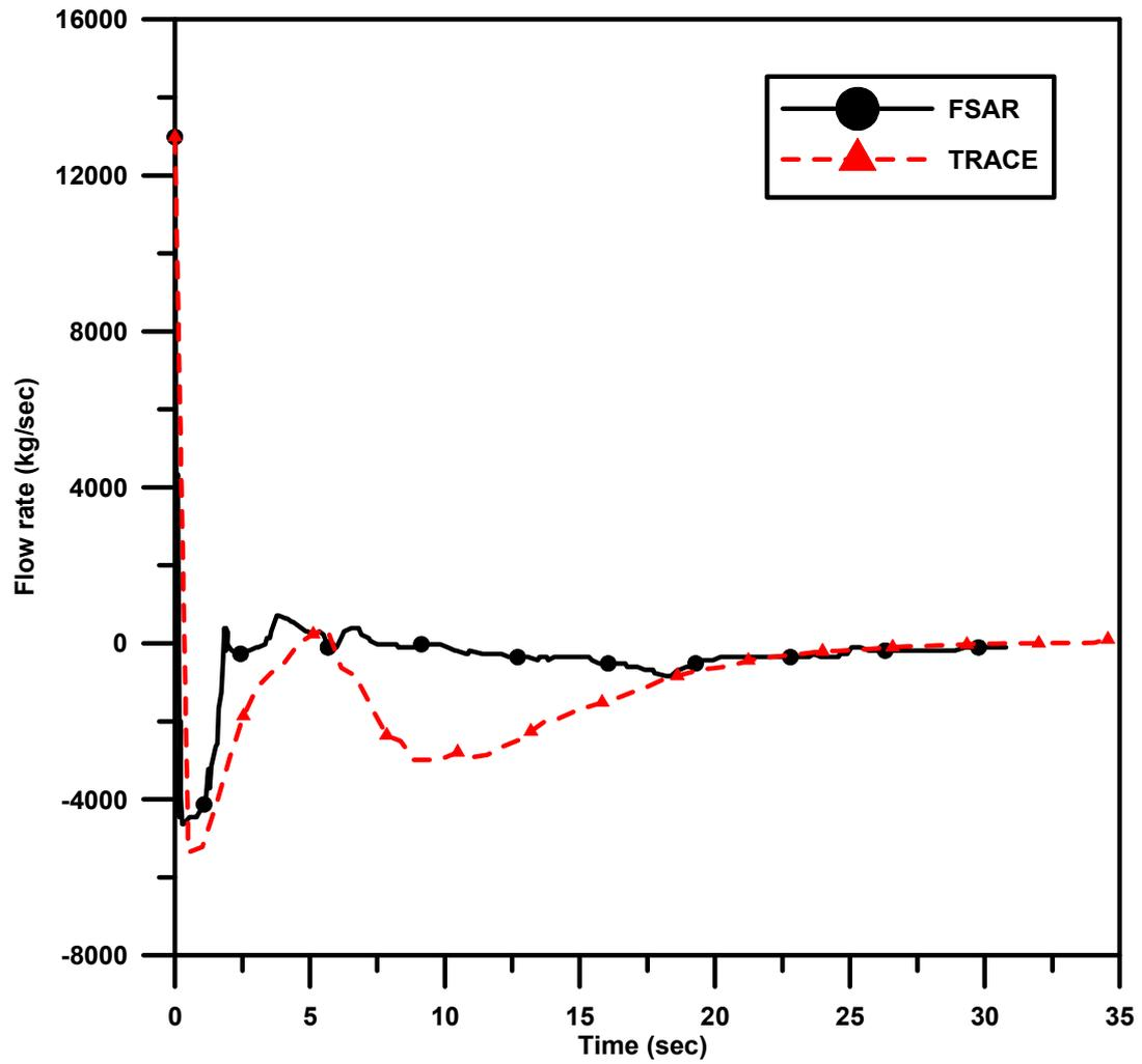
Fig. 4.5 The comparisons of core inlet flow rate between TRACE and FSAR data.
