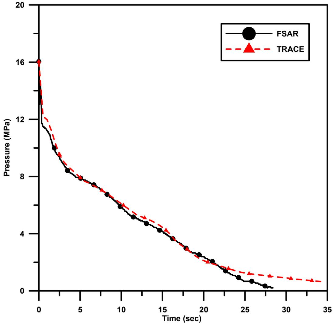
Fig. 4.2 The comparisons of vessel pressure between TRACE and FSAR data.
