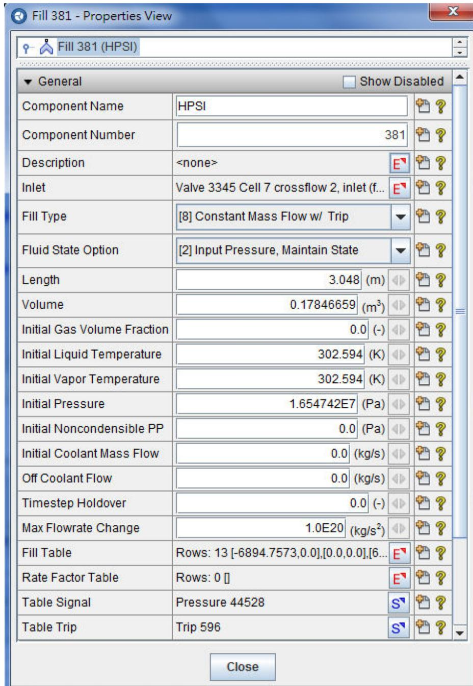
Fig 2.6 The HHSI simulation of TRACE LBLOCA model.
