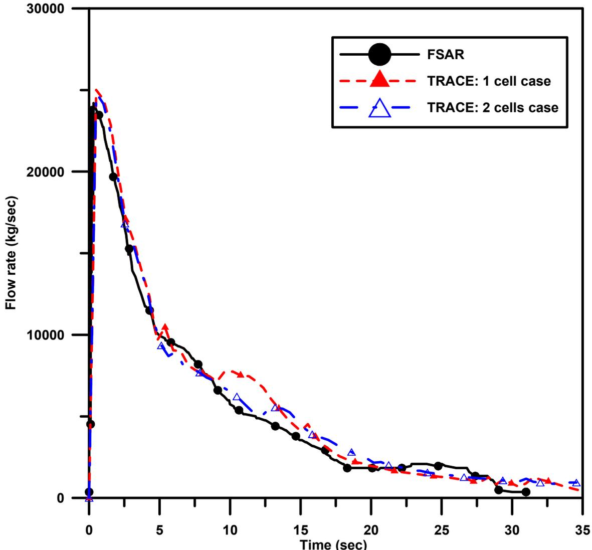
Fig 4.12 The break flow rate results of the pipe nodalization (near the break) sensitivity studies.
