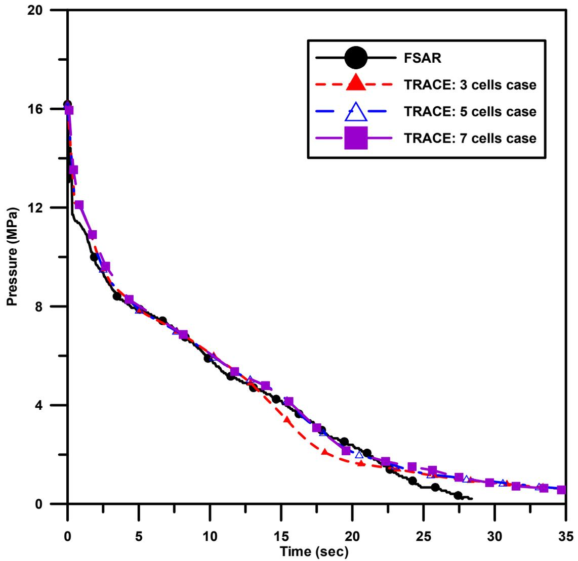
Fig 4.10 The system pressure results of the accumulators nodalization sensitivity studies.
