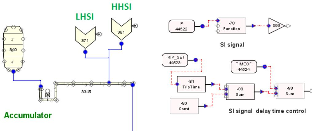
Fig 2.3 The TRACE model of the ECCS control system for Maanshan NPP.
