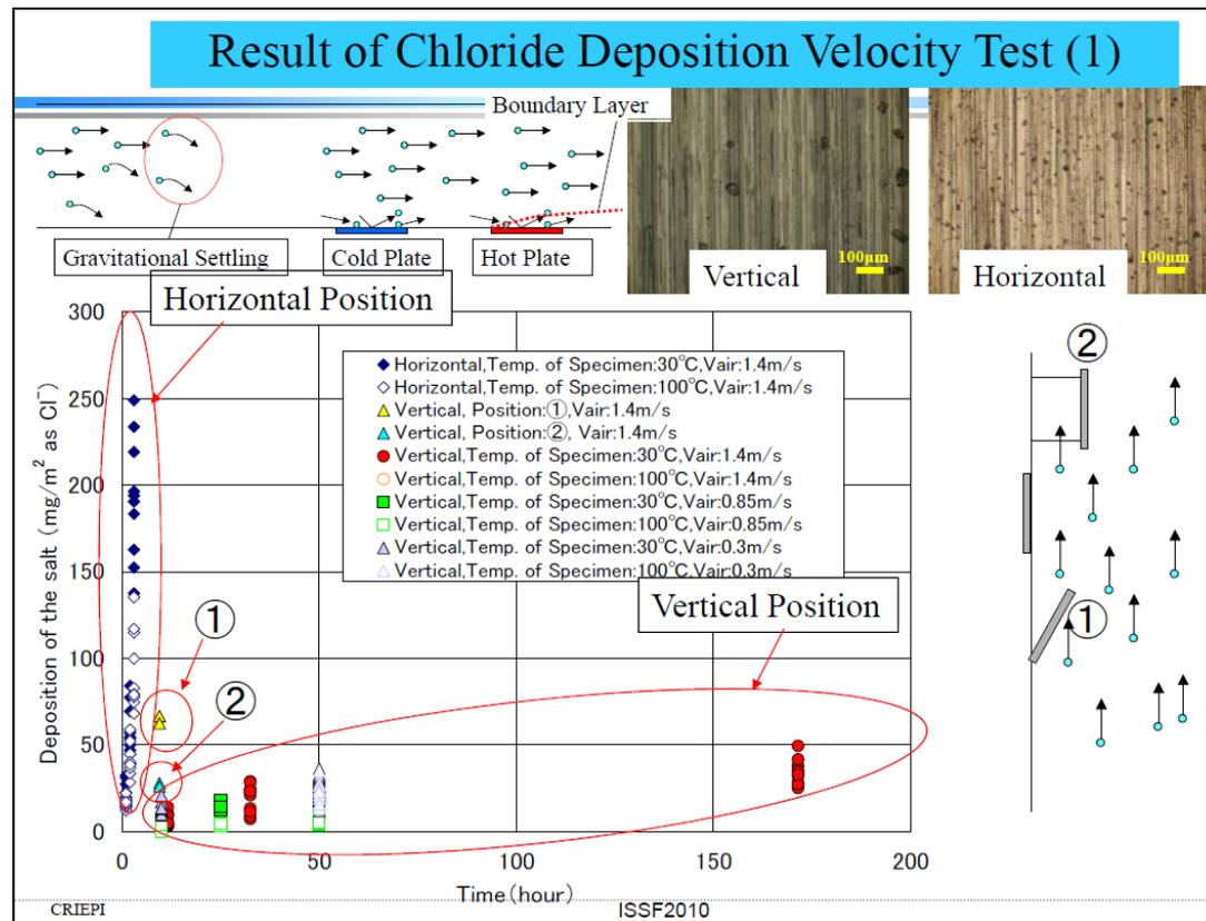
A Schematic Deposition Rate for Various Air Flow Configurations.
