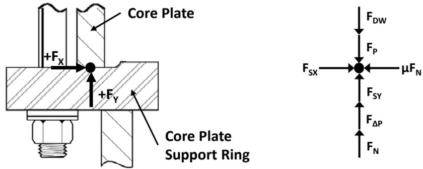
**Figure 2-6: Core Plate Bolt Free-body Diagram**
