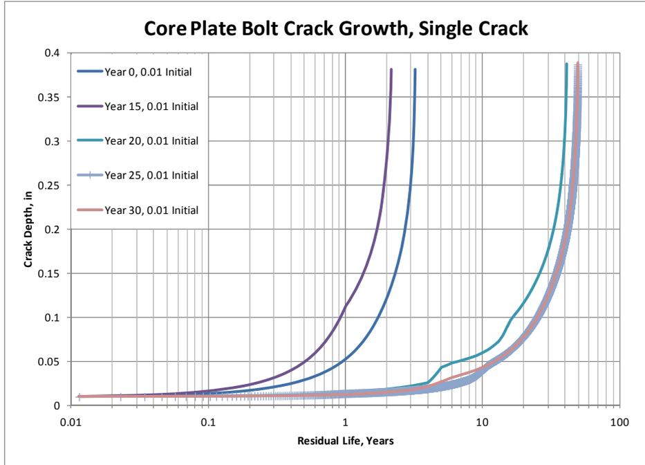
**Figure 2-5: Crack Growth Curves - Single Crack Case, Various Initiation Times**
