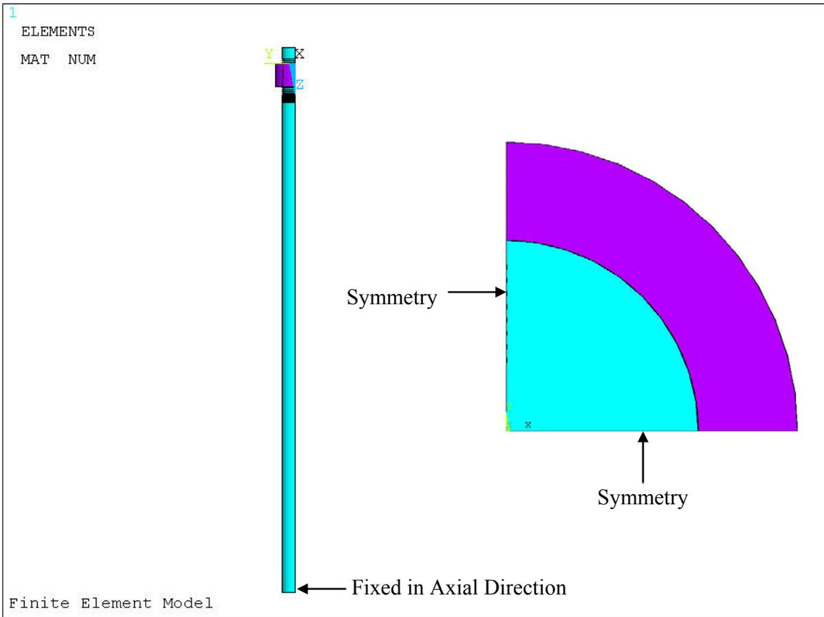
**Figure 2-3: Boundary Conditions Applied to Model**
