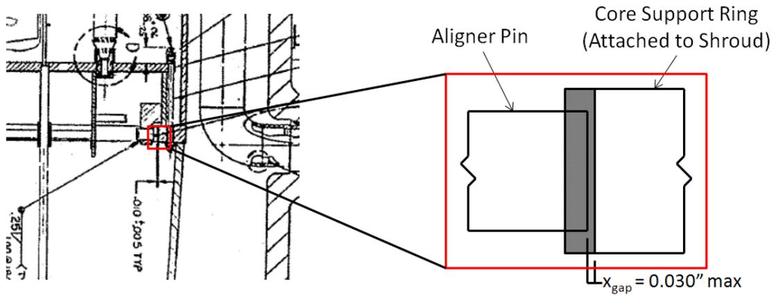
**Figure 2-8: Aligner Pin and Core Support Ring Interface**
