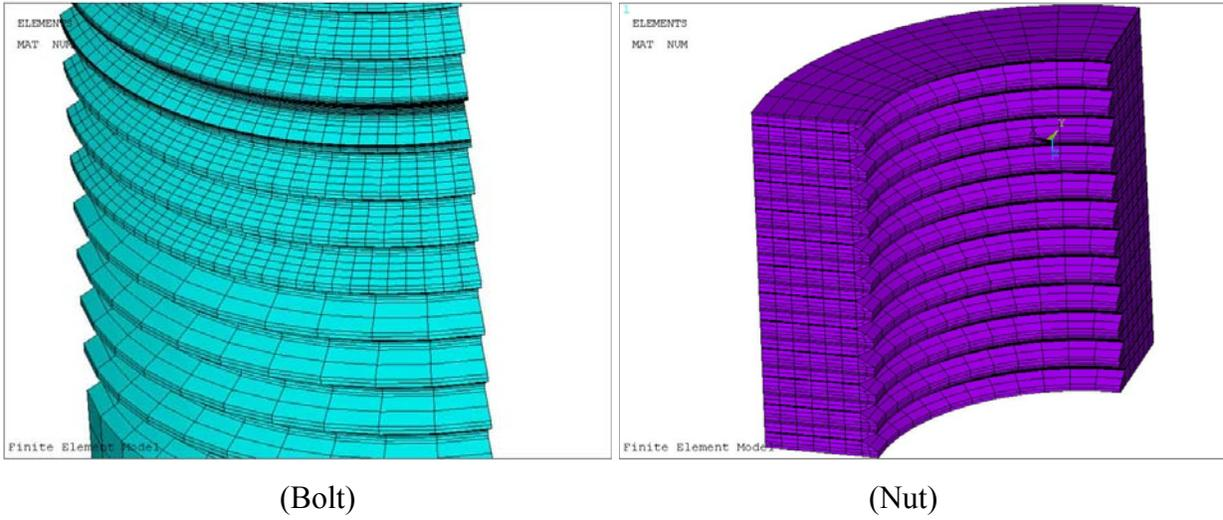
**Figure 2-2: 3-D Finite Element Model, Bolt and Nut Thread Detail View**
