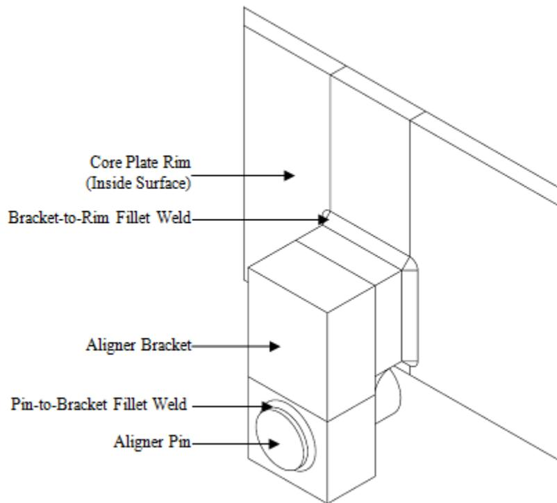
**Figure 2-7: General View of Aligner Pin and Bracket Assembly**
