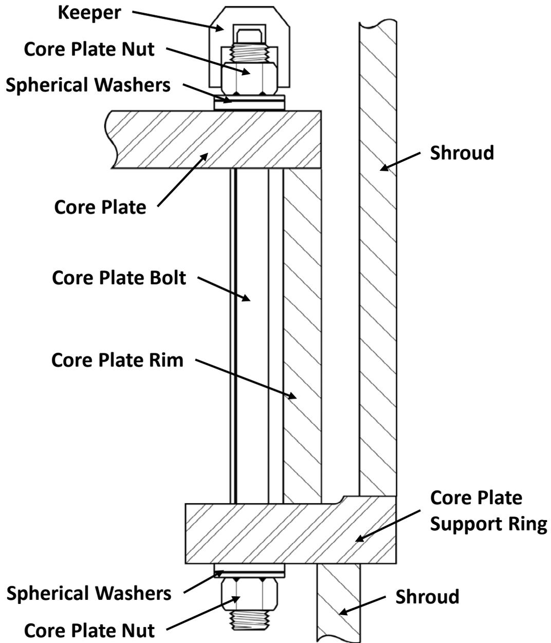
Figure 1-1: Core Plate Bolt Assembly
