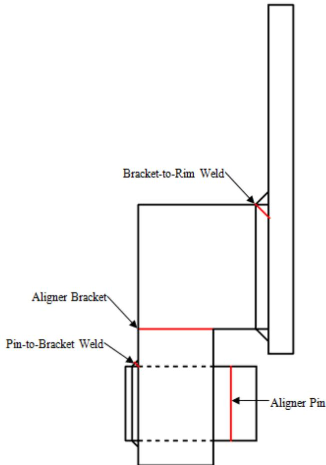
**Figure 2-9: Aligner Pin Assembly Cross Sections Analyzed**
