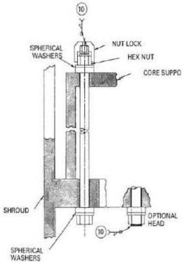
Figure 1: Typical Core Plate Bolt
