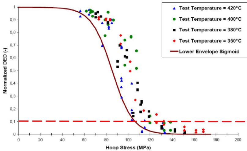
Figure 12 : Ductile to brittle transition observed on unirradiated hydrided Zirlo™ ring tensile specimens tested at ambient temperature as function of the treatment stress and temperature [14]. Normalized DED is the ratio between post treatment DED and initial DED, which is around  $0.6 \text{ J/mm}^2$
