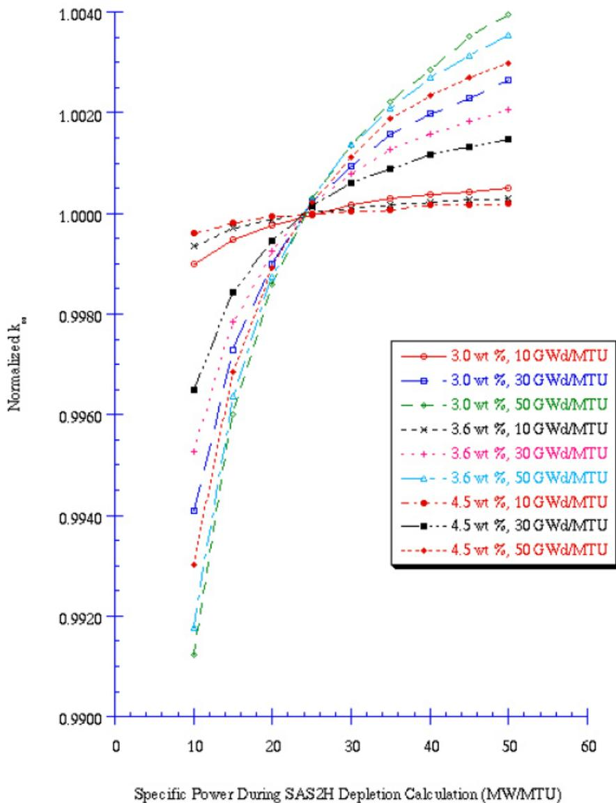
Figure A-5: Reactivity effect of specific power during depletion on  $k_{inf}$  in an array of fuel pins (actinides only).<sup>10</sup>
