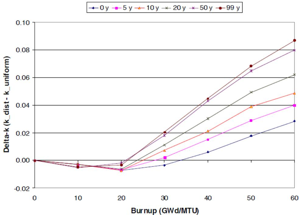
Figure A-7: Effect of axial burnup distribution on  $k_{eff}$  in the GBC-32 cask for actinide-only burnup credit and various cooling times for fuel with 4.0 weight percent initial enrichment.<sup>9</sup>
