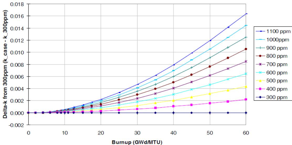
Figure A-4: Reactivity effect of soluble boron concentration during depletion on  $k_{inf}$  in an array of poisoned storage cells. Results correspond to fuel with 5.0 weight percent initial  $^{235}\text{U}$  enrichment.<sup>9</sup>
