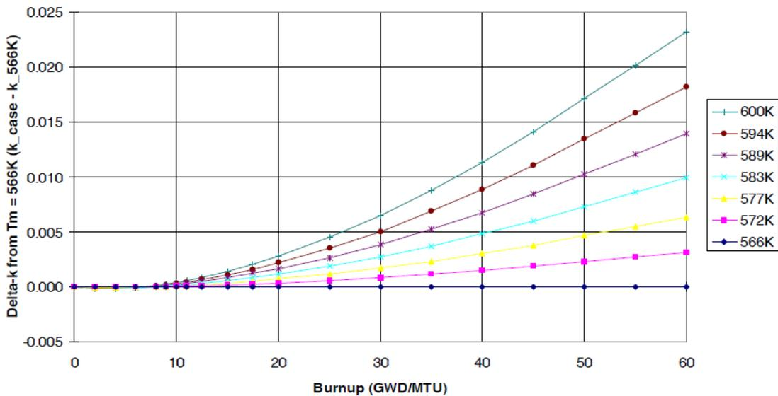
Figure A-3: Reactivity effect of moderator temperature during depletion on  $k_{inf}$  in an array of poisoned storage cells. Results correspond to fuel with 5.0 weight percent initial  $^{235}\text{U}$  enrichment.<sup>9</sup>
