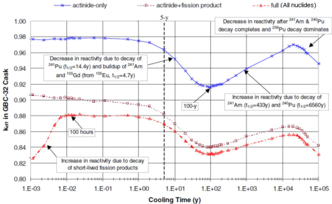
Figure A-1: Reactivity behavior in the GBC-32 cask as a function of cooling time for fuel with 4.0 weight percent  $^{235}\text{U}$  initial enrichment and 40 GWd/MTU burnup<sup>7</sup>
