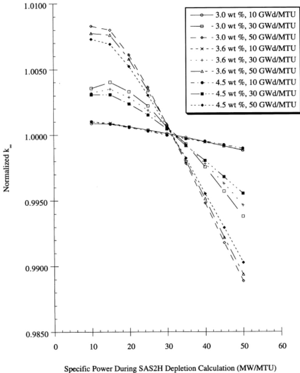
Figure A-6: Reactivity effect of specific power during depletion on  $k_{inf}$  in an array of fuel pins (actinides and fission products).<sup>10</sup>
