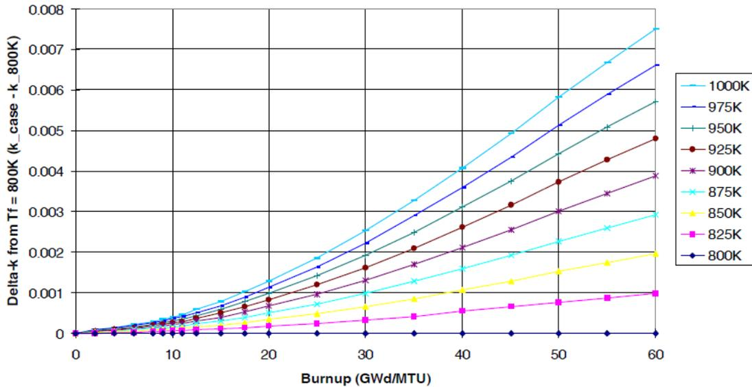
Figure A-2: Reactivity effect of fuel temperature during depletion on  $k_{inf}$  in an array of poisoned storage cells. Results correspond to fuel with 5.0 weight percent initial  $^{235}\text{U}$  enrichment.<sup>9</sup>
