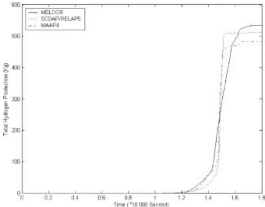
**The onset of hydrogen production** (start of fuel damage) is predicted to occur at nearly the same time by all three codes, and roughly the same amount of hydrogen is produced.
