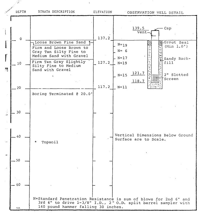
LocationWestinghouseDepth of Water @N/A1. Time of installationN/A2. At least 24 hours laterSee Table 1Drilling MethodWash Boring
